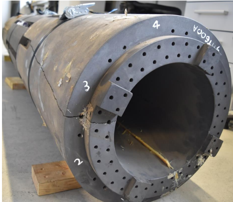
Figure 2.5 - An example of a graphite brick which has an axial crack.
