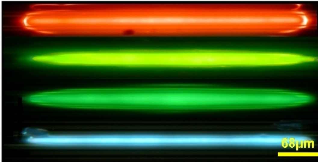
Figure 5.7: Optical micrographs of blue (486 nm), green(524 nm), yellow(560 nm), and red(609 nm) emitting pixels put together.
