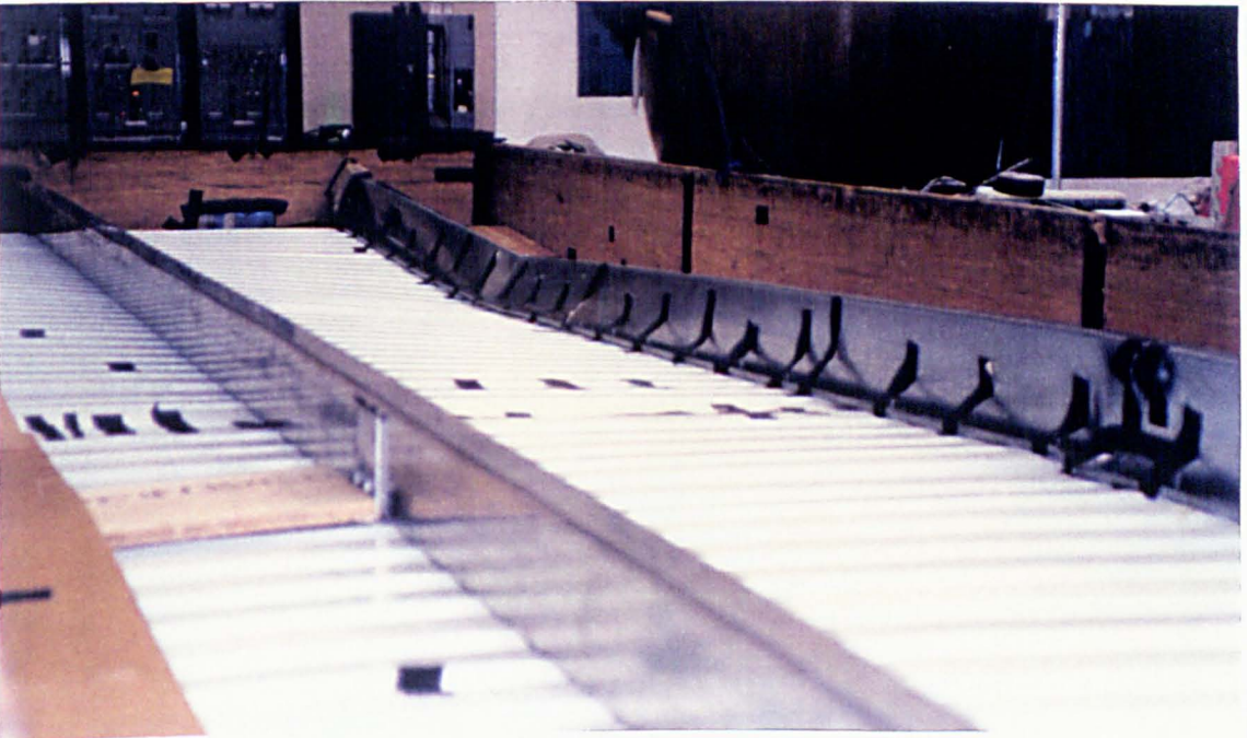
Figure 5.2.5 : Observed Zed Mechanism along the span
