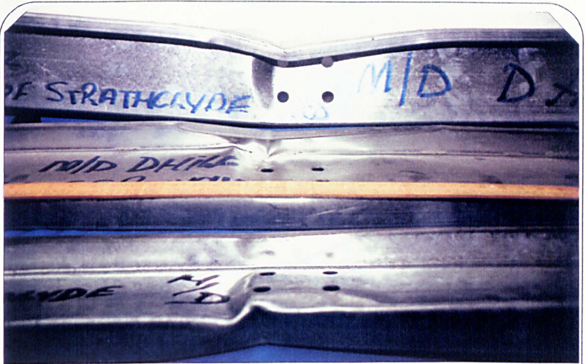
Figure 5.2.1 : Observed Zed Mechanism at Cleat Location
