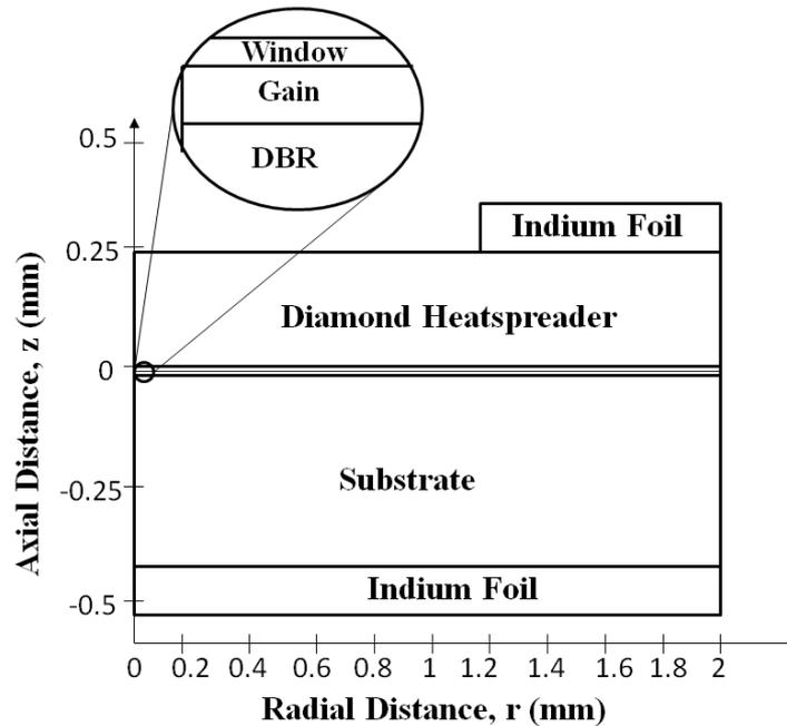
**Figure 3-2: Diagram of thermal model system, including the window, gain and DBR, with the diamond heatspreader adjacent to the confinement window and the substrate under the DBR mirror, with indium foil at the intermediate layer to the submount.**
