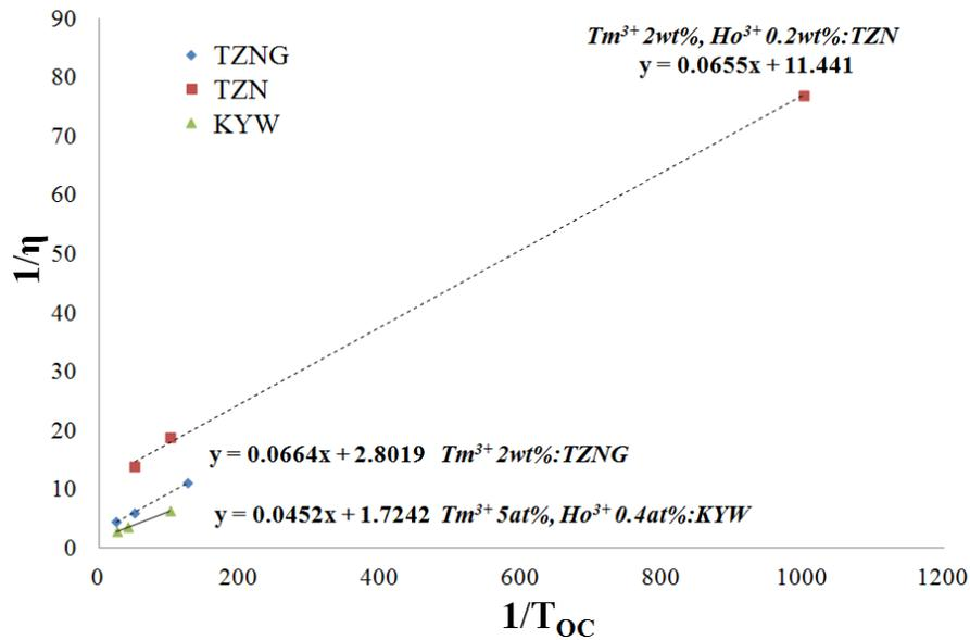
**Figure 5-15: Caird analysis using inverse slope efficiencies as a function of the inverse of the output coupler transmission  $T_{OC}$ , results for  $Tm^{3+}, Ho^{3+}:TZN$ ,  $Tm^{3+}:TZNG$  and  $Tm^{3+}, Ho^{3+}:KYW$ .**
