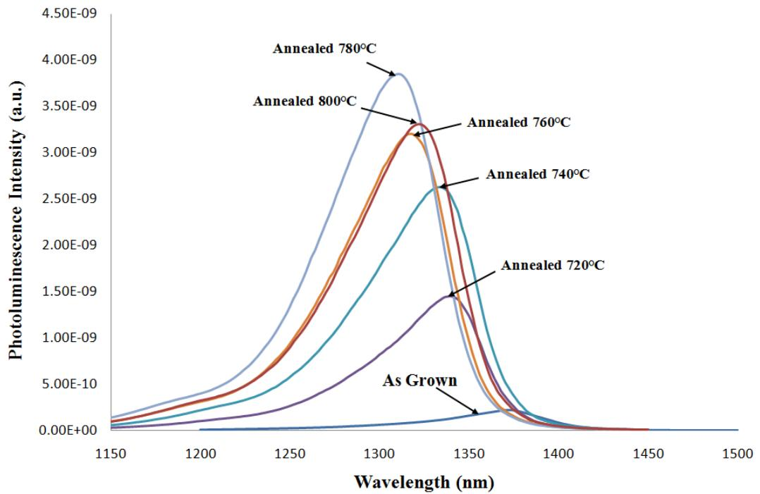
**Figure 2-27: Photoluminescence spectra from  $\text{In}_{0.31}\text{Ga}_{0.69}\text{As}_{0.982}\text{N}_{0.018}/\text{GaAsN}$  QW structure, showing the increased PL intensity compared to the as grown sample with increasing RTA temperature.**
