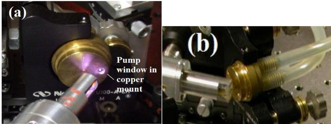
**Figure 3-17: (a) Front view of copper mount of the SDL indicating the pump window cut into the cap of the mount. (b) Side view of the mount to show the connection to the water cooling pvc tubing.**
