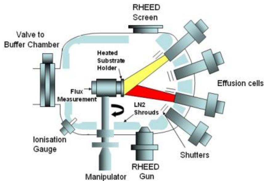
Figure 2-25: Schematic of the MBE chamber.
