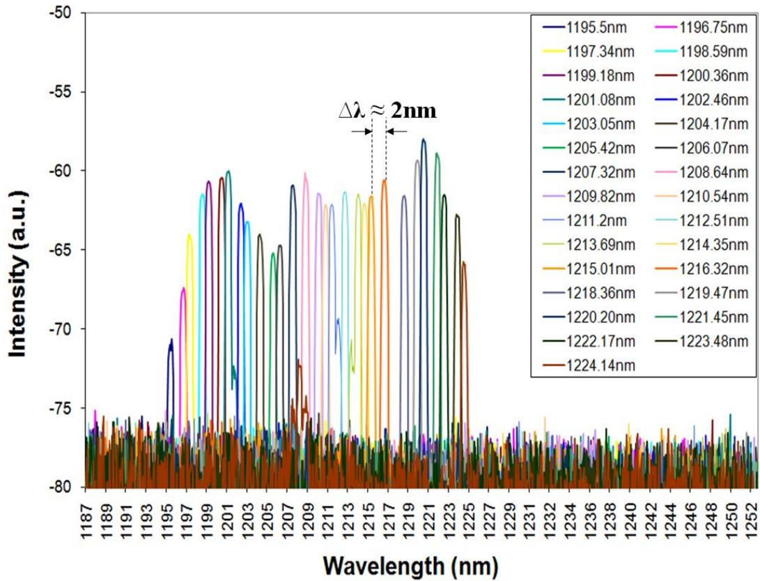
**Figure 4-25: Wavelength tuning spectra, from 1195.5 nm to 1223.48 nm, indicated is the peak-to-peak wavelength separation  $\Delta\lambda \approx 2\text{nm}$ .**
