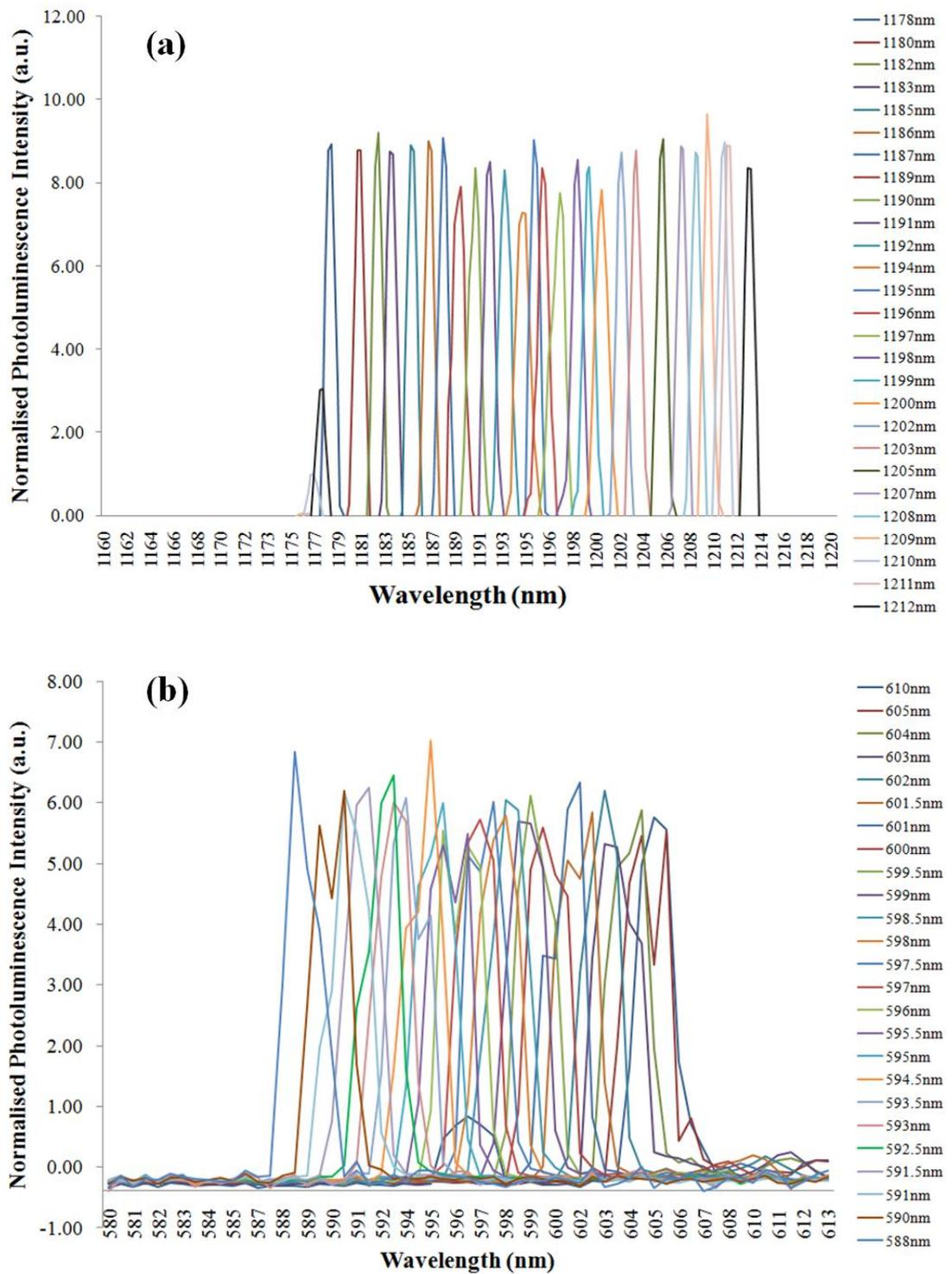
Figure 6-20: (a) Wavelength tuning spectra of the fundamental from 1178 nm to 1212 nm, (b) tuning spectra of the second harmonic from 588 nm to 610 nm.
