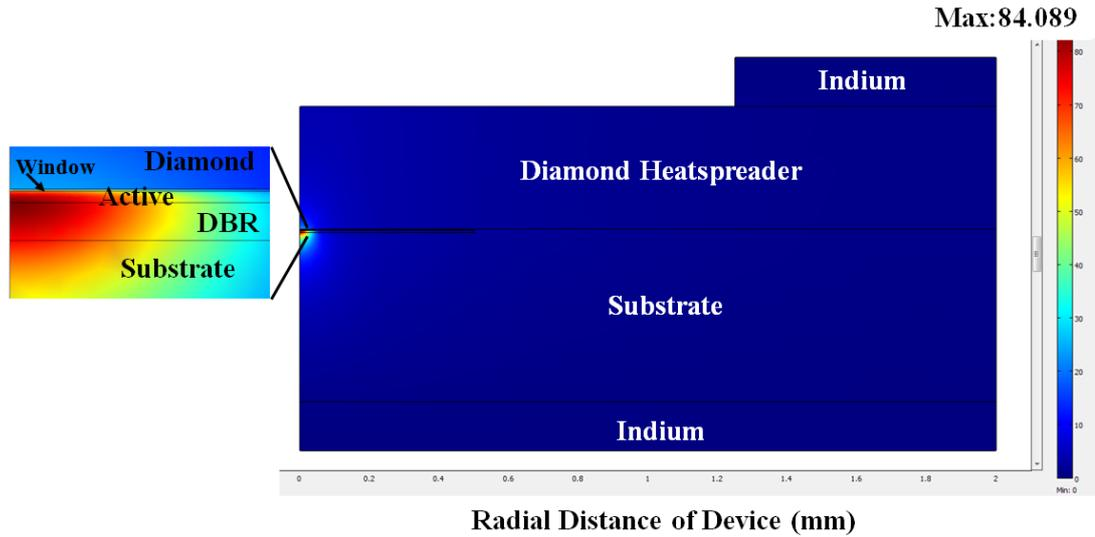
**Figure 4-33: COMSOL Multiphysics™ simulation results of the GaInNAs SDL, indicating a maximum temperature of 84.089°C.**
