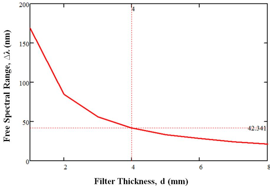
**Figure 4-23: Free spectral range capability over a range of filter thicknesses, indicating  $\Delta\lambda=42nm$  for a 4 mm thick BRF at a tuning angle  $\varphi=41^\circ$ .**
