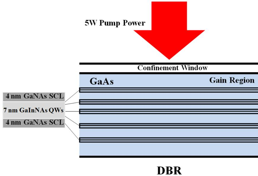
**Figure 3-4: Schematic of pumping with 5W pump power, incident onto the confinement window and absorbed in the gain region, predominantly composed of GaAs absorption/spacer layers with 7 nm GaInNAs QWs and 4 nm GaNAs SCLs.**
