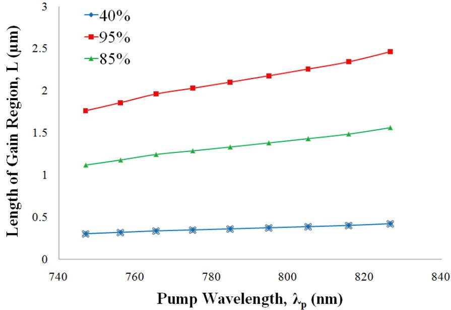
**Figure 2-20: Length of the gain region across a range of pump wavelengths, for expected pump absorptions of 40%, 85% and 95%.**
