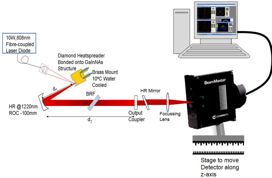
**Figure 4-19: Schematic of  $M^2$  measurement apparatus using the BeamMaster scanning detector.**
