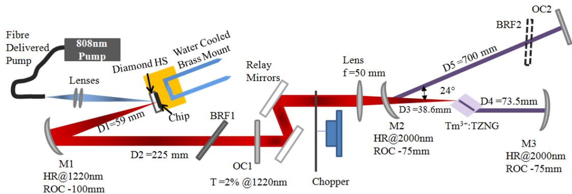
**Figure 5-13: Schematic of the SDL pumping of the Tm-doped glass laser, using the  $\text{Tm}^{3+}:\text{TZNG}$  glass sample that was Brewster cut with length 5 mm.**
