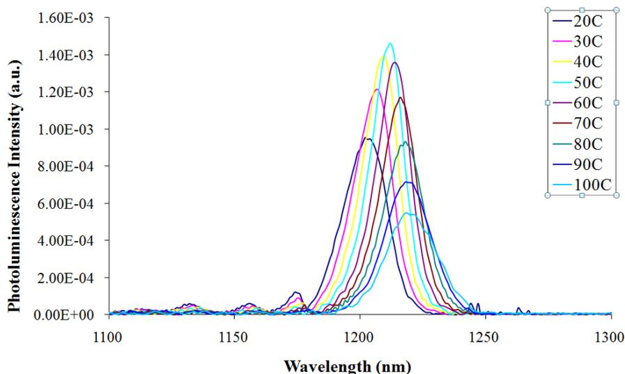
**Figure 4-7: Photoluminescence results for sample *AsN2527* designed with 1220 nm output, over a range of temperatures.**
