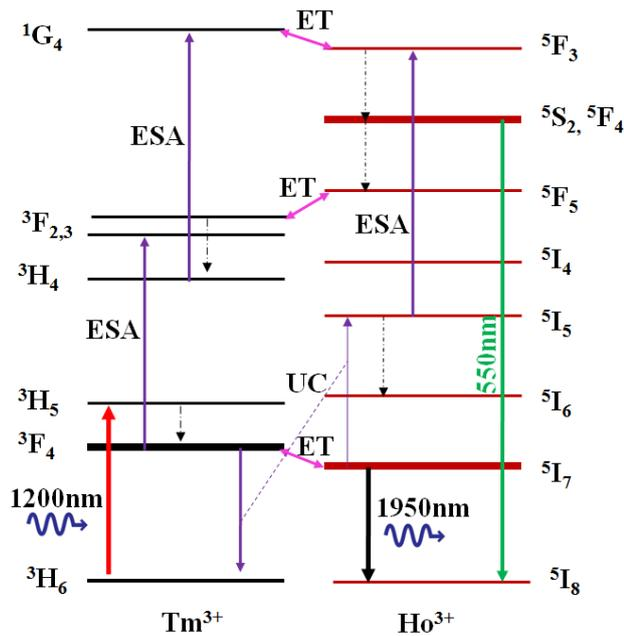
**Figure 5-7:  $\text{Tm}^{3+}$  and  $\text{Ho}^{3+}$  energy transitions using a 1200 nm pumping scheme, with excited-state absorption (ESA) and upconversion (UC) processes (purple), energy transfers (ET) between  $\text{Tm}^{3+}$  and  $\text{Ho}^{3+}$  (pink arrows), nonradiative decay (black dashed), and emission transitions 550 nm and 1950 nm.**
