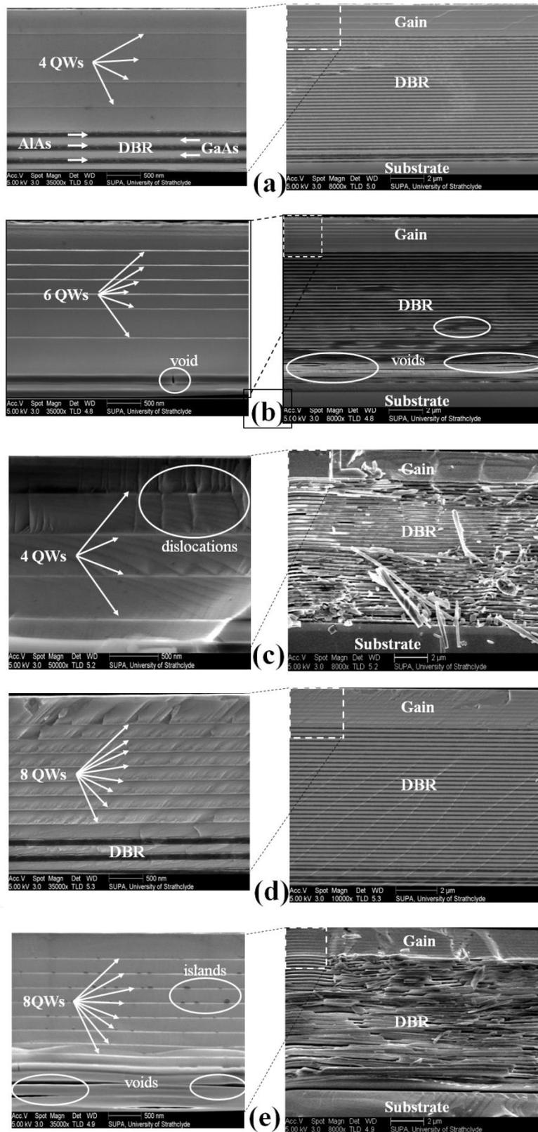
**Figure 4-10: SEM images of (a) 4 QW GaInAs/GaAs Vn1381, (b) 6 QW GaInNAs/GaAs Vn1567, (c) 4 QW GaInNAs/GaAs Vn1534, (d) 8 QW GaInAs/GaAs Vn1399 and (e) 8 QW GaInNAs/GaAs Vn1536.**
