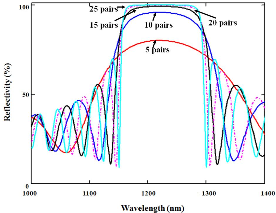
**Figure 2-3: AlAs/GaAs DBR stack with increasing mirror pairs from 5 to 25 ( $\lambda_B=1220\text{nm}$ ).**
