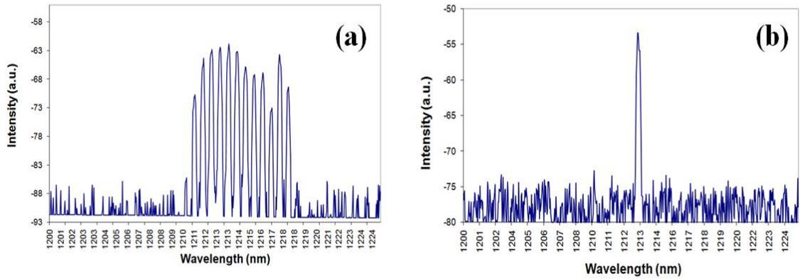
**Figure 4-24: (a) Spectrum of a free-running AsN2527 1220 nm SDL, and (b) BRF selection of 1213 nm output wavelength.**
