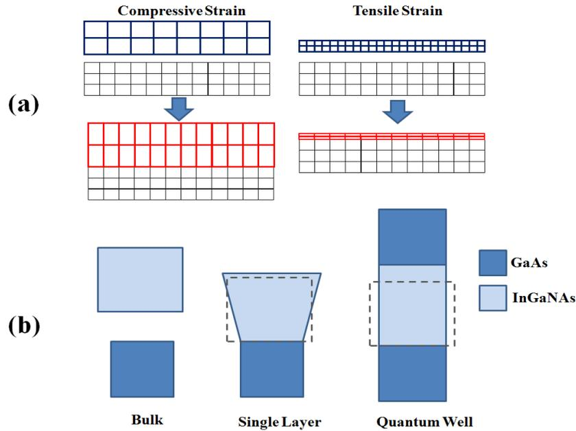
**Figure 2-8: (a) Illustration of compressive and tensile strain due to materials with different lattice constants. (b) Comparison of bulk materials with that of a single layer and quantum well with subsequent strain in the material [21].**
