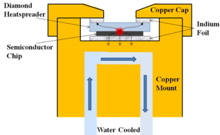
**Figure 3-16: Schematic of the water cooled copper heatsink, with the diamond bonded semiconductor chip and indium foil.**
