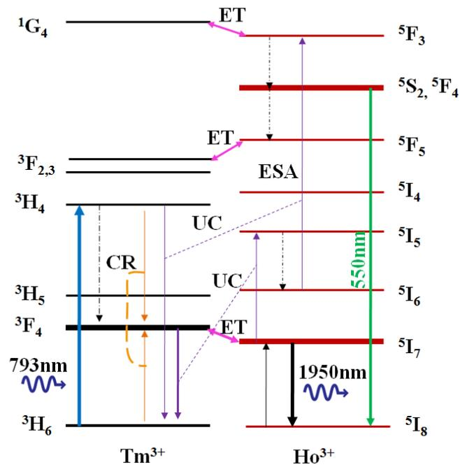
**Figure 5-4:**  $\text{Tm}^{3+}$  and  $\text{Ho}^{3+}$  energy transitions from a 793 nm excitation source, with cross-relaxation (CR) (orange lines), energy transfers (ET) between  $\text{Tm}^{3+}$  and  $\text{Ho}^{3+}$  (pink arrows), upconversion (UC) and excited-state absorption (ESA) (purple lines), nonradiative decay (black dashed) and emission transitions 550 nm and 1950 nm.
