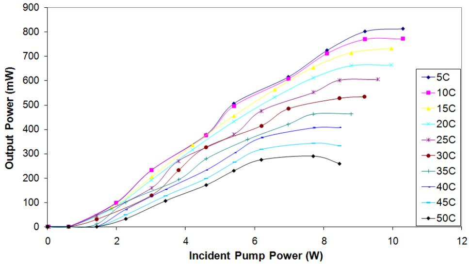
**Figure 4-29: Power transfer curves ranging in temperature from 5°C to 50°C.**
