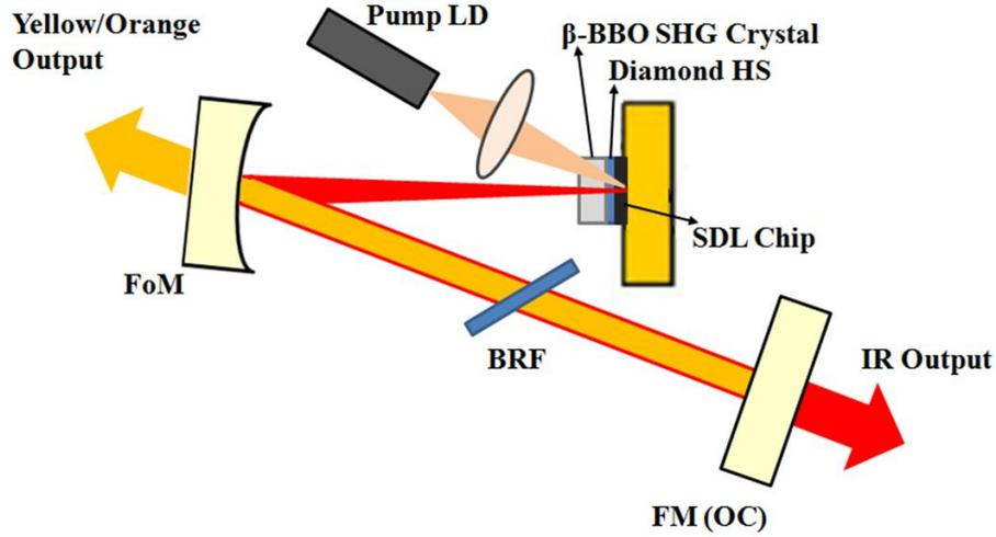
**Figure 6-6: The V-cavity configuration based on Kim et al [60], adapted with the double bonded SDL chip, Diamond HS and  $\beta$ -BBO nonlinear crystal. Includes are the birefringent filter *BRF* between the folding mirror *FoM* and the output coupler/Flat mirror *FM (OC)*.**
