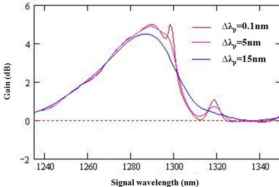
**Figure 5-27: Simulation gain profile at the end of the Raman fibre, across pump laser linewidths  $\Delta\lambda_p = 0.1\text{nm}$ , 5 nm and 15nm (Programme Courtesy of Dr. S. Calvez).**
