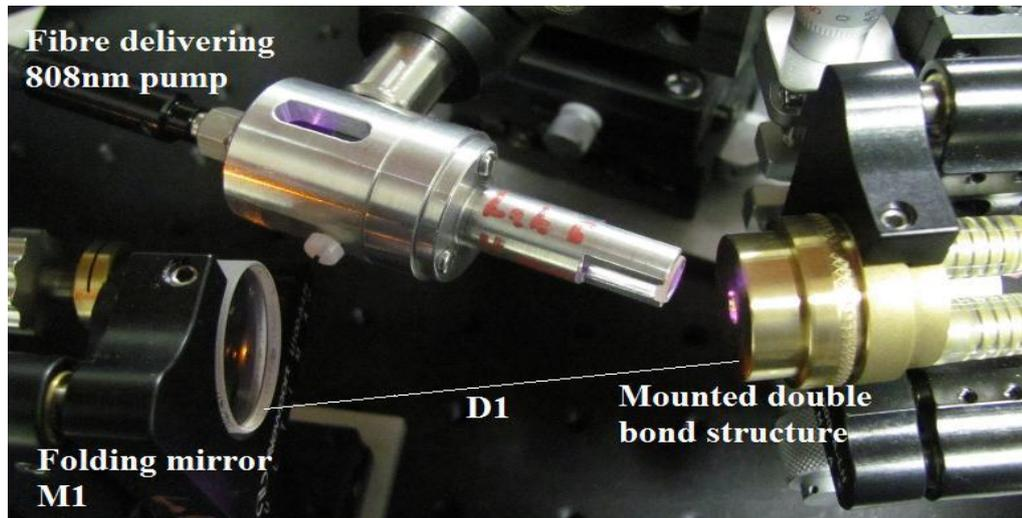
**Figure 6-16: Picture of the 808 nm diode pump delivery through fibre and lenses, the mounted double bonded structure on the right and the folding mirror, M1 on the left. (Photo courtesy of Dr. S. Calvez)**
