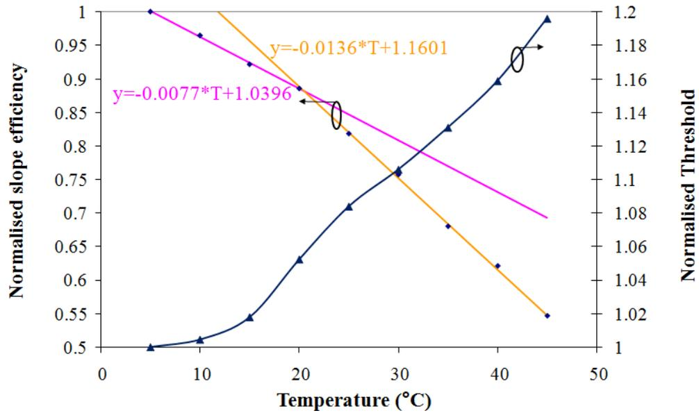
**Figure 4-18: Normalised slope efficiency and threshold pump powers over a range of temperatures for the AsN2592 1200 nm device [11].**
