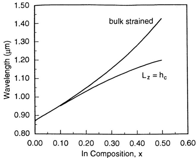
**Figure 2-10: Wavelength ranges possible for  $\text{In}_x\text{GaAs}/\text{GaAs}$  QWs, where the QW thickness is set to the critical thickness, compared with bulk strained QW [21].**
