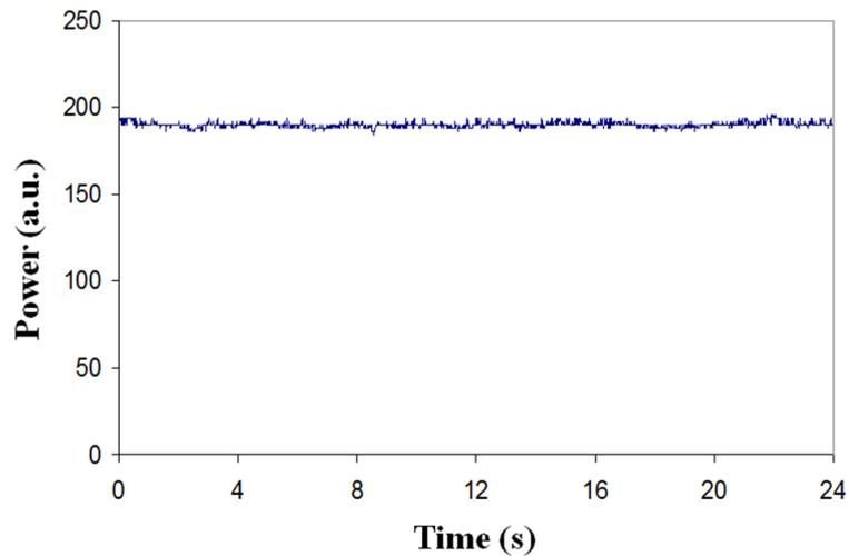
Figure 5-22: Time-dependent performance of 1220 nm SDL operating at full power [59].
