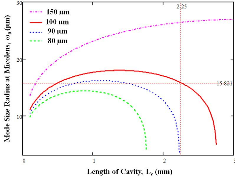
**Figure 6-11: Microlens mode sizes with lens diameters  $d$  150  $\mu\text{m}$ , 100  $\mu\text{m}$ , 90  $\mu\text{m}$  and 80  $\mu\text{m}$  over a range of cavity lengths for a frequency doubled microcavity SDL.**
