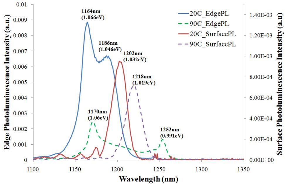
**Figure 4-5: Comparison of Edge and Surface PL for measurements taken at 20°C and 90°C, indicated are the intensity peak wavelengths.**
