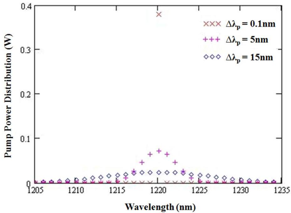
**Figure 5-26: Simulation of 0.38 W Pump power with a variable Gaussian spectral distribution in the Raman fibre, across pump laser linewidths  $\Delta\lambda_p = 0.1\text{nm}$ , 5 nm and 15nm (Programme Courtesy of Dr. S. Calvez).**
