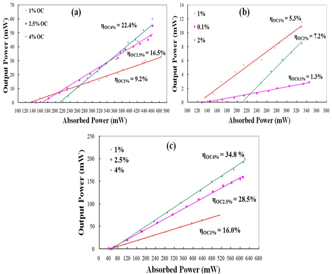
Figure 5-14: ~2  $\mu m$  output power as a function of absorbed power results for (a)  $Tm^{3+}$ :TZNG, (b)  $Tm^{3+}, Ho^{3+}$ :TZNG and (c)  $Tm^{3+}, Ho^{3+}$ :KYW.
