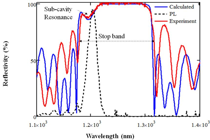
**Figure 4-2: Reflectivity measured at 20°C of sample *AsN2527* (red), indicating the stopband and sub-cavity resonance dip, compared with the calculated reflectivity of a 10 QW 1220 nm SDL is included (blue). Included is PL spectra at 20°C (black dashed line).**
