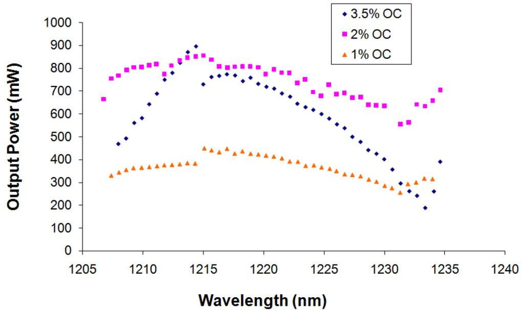
**Figure 4-26: Wavelength tuning results for the *AsN2527* 1220 nm SDL, for output coupler transmissions 1%, 2% and 3.5%.**
