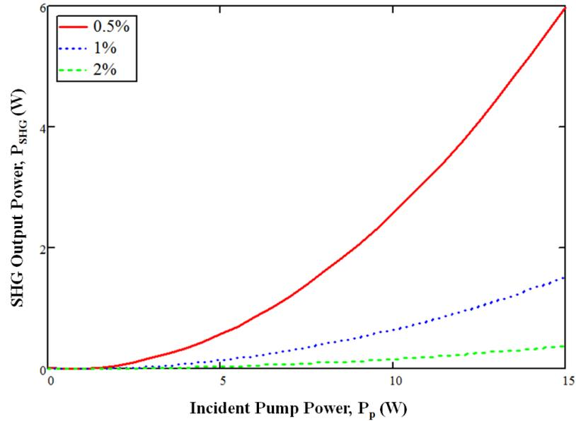
**Figure 6-7: Simulated SHG output power for loss  $\alpha_L$  values of 0.5%, 1% and 2%.**
