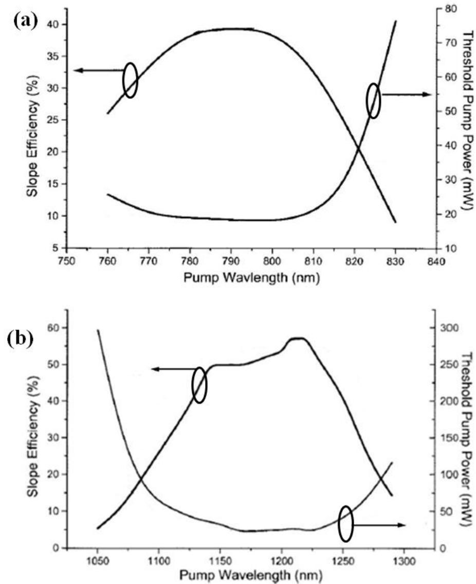
**Figure 5-8:** Calculated results for  $\text{Tm}^{3+}$ -doped silica fibres, showing the estimated slope efficiency and threshold pump power for (a)  ${}^3\text{F}_4$  absorption band pumping and (b)  ${}^3\text{H}_5$  absorption band pumping [36].
