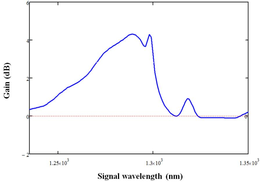
**Figure 5-20: Simulated results of the Raman gain spectrum for the silica fibre pumped by a 1220 nm source.**
