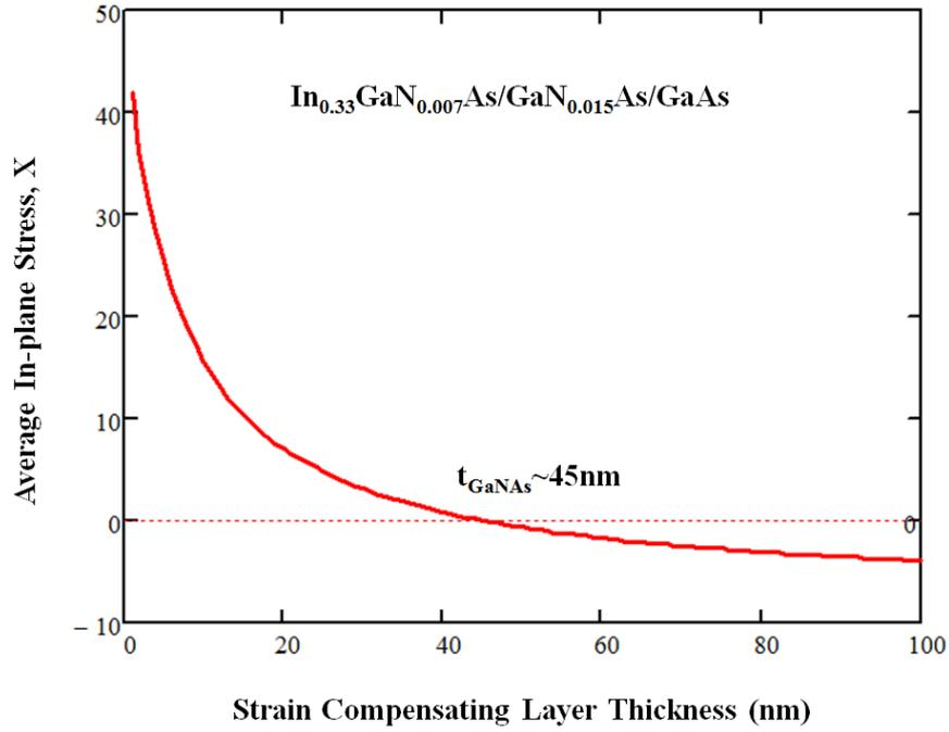
**Figure 2-14: Average in-plane stress for a biaxially strained material system with respect to the compensating layer thickness.**
