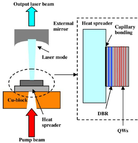
**Figure 3-10: Design of an end pumped SDL as used by Lee et al [32] to achieve 9.1W CW power.**
