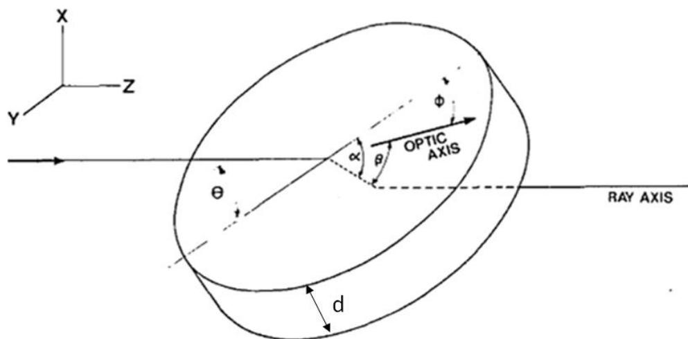
**Figure 4-21: Birefringent filter illustration to show the angular dependence of the incident beam through the filter with thickness  $d$ , at an incident angle  $\theta$ , rotation angle  $\phi$ , angle between the refracted ray and the optic axis  $\beta$ , and the angle between the refracted ray and the plate angle  $\alpha$  [14].**
