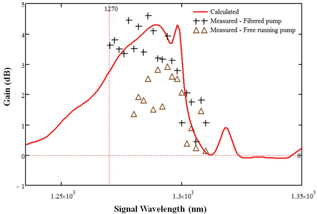
**Figure 5-25: Empirical Raman gain results for free running pump (*brown triangles*) and filtered pump (*black crosses*) at 1216 nm pump wavelength, compared with simulated spectral gain results (*red solid line*) (*Programme Courtesy of Dr. S. Calvez*).**
