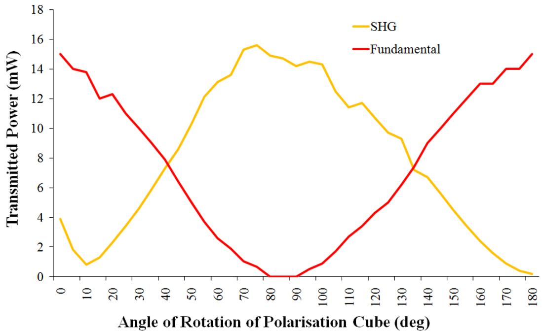
**Figure 6-18: Graph of the transmitted powers of the fundamental and frequency doubled beams through 180° rotation of the polarisation cube.**
