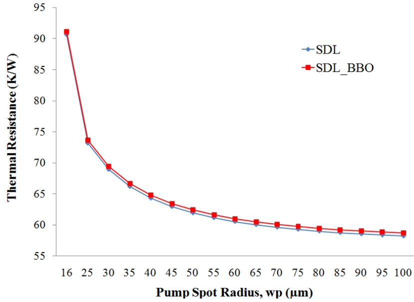
**Figure 6-13: Thermal resistance comparison based on simulations of the 1180 nm GaInNAs SDL and the double bonded  $\beta$ -BBO SDL.**
