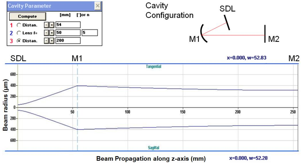
**Figure 4-11: Winlase<sup>TM</sup> simulation of a cavity designed for 1220nm operation, indicated are the locations of the *SDL* chip, folding mirror *M1* and output coupler mirror *M2* as shown in the cavity configuration.**
