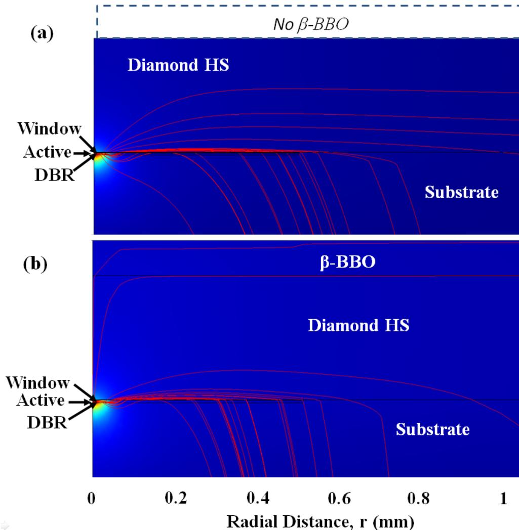
**Figure 6-12: (a) Finite Element Analysis indicating the the heat flux paths (*red lines*) for the 1180 nm 10 QW GaInNAs/GaNAs/GaAs SDL with a diamond HS and pump spot radius  $w_p=40\ \mu\text{m}$ , (b) the same sample with the inclusion of the bonded  $\beta$ -BBO nonlinear crystal.**
