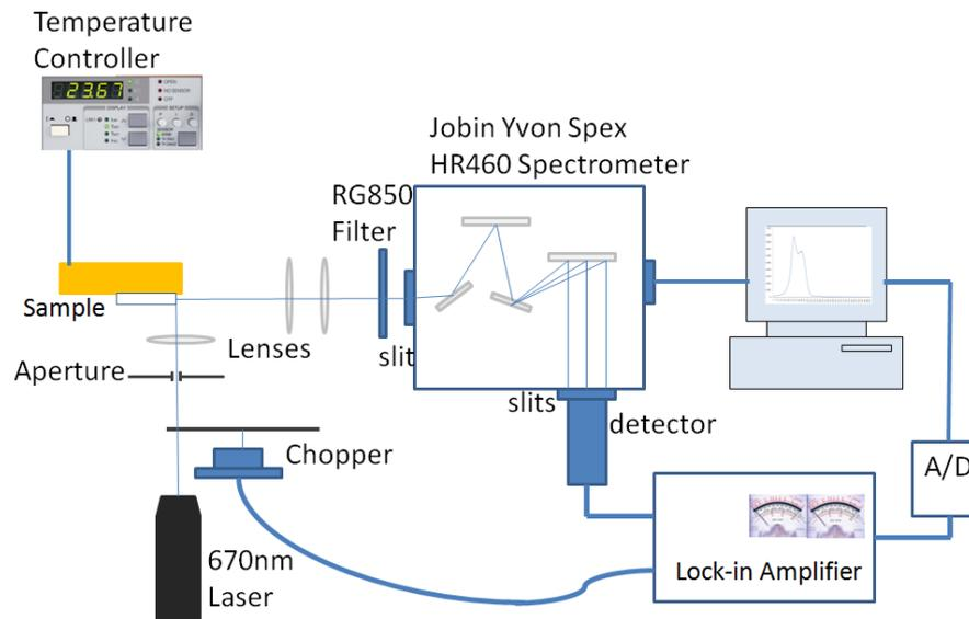
**Figure 4-3: Edge PL measurement setup.**
