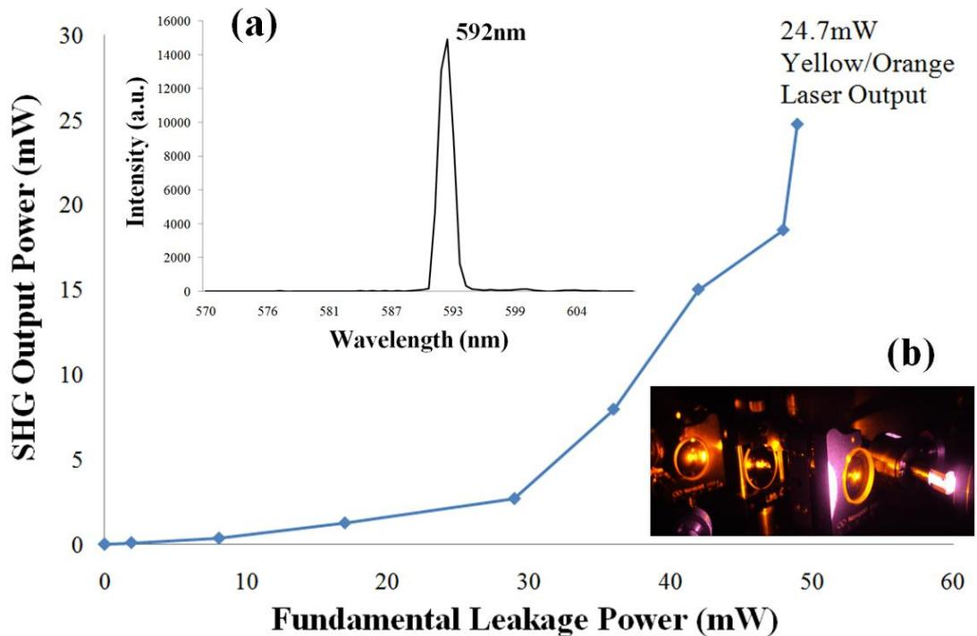
**Figure 6-17: SHG output as a function of the Fundamental Leakage Power, inset (a) the SHG spectrum showing a peak at 592 nm and (b) photo of the yellow/orange laser output at the SDL folding mirror and immediately behind, focussing optics to the detector.**
