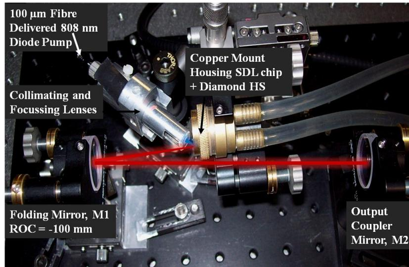
Figure 4-13: SDL in a three-mirror cavity configuration showing the beam path (red), the laser cavity is formed between the SDL, M1 and M2.
