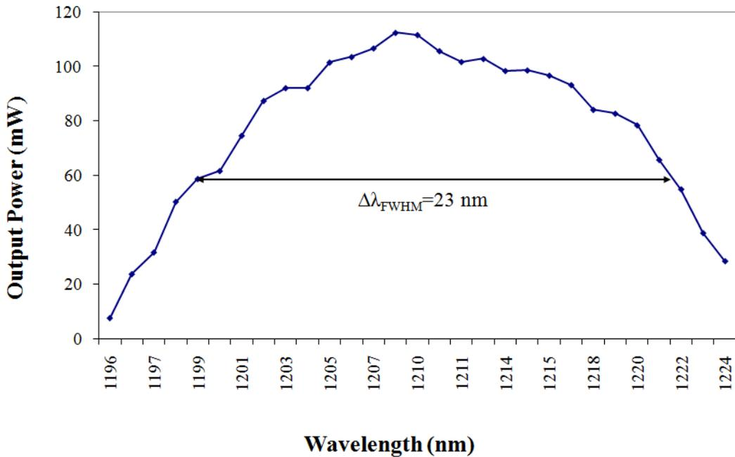
**Figure 5-11: Wavelength tuning range for AsN2527 1220 nm SDL.**
