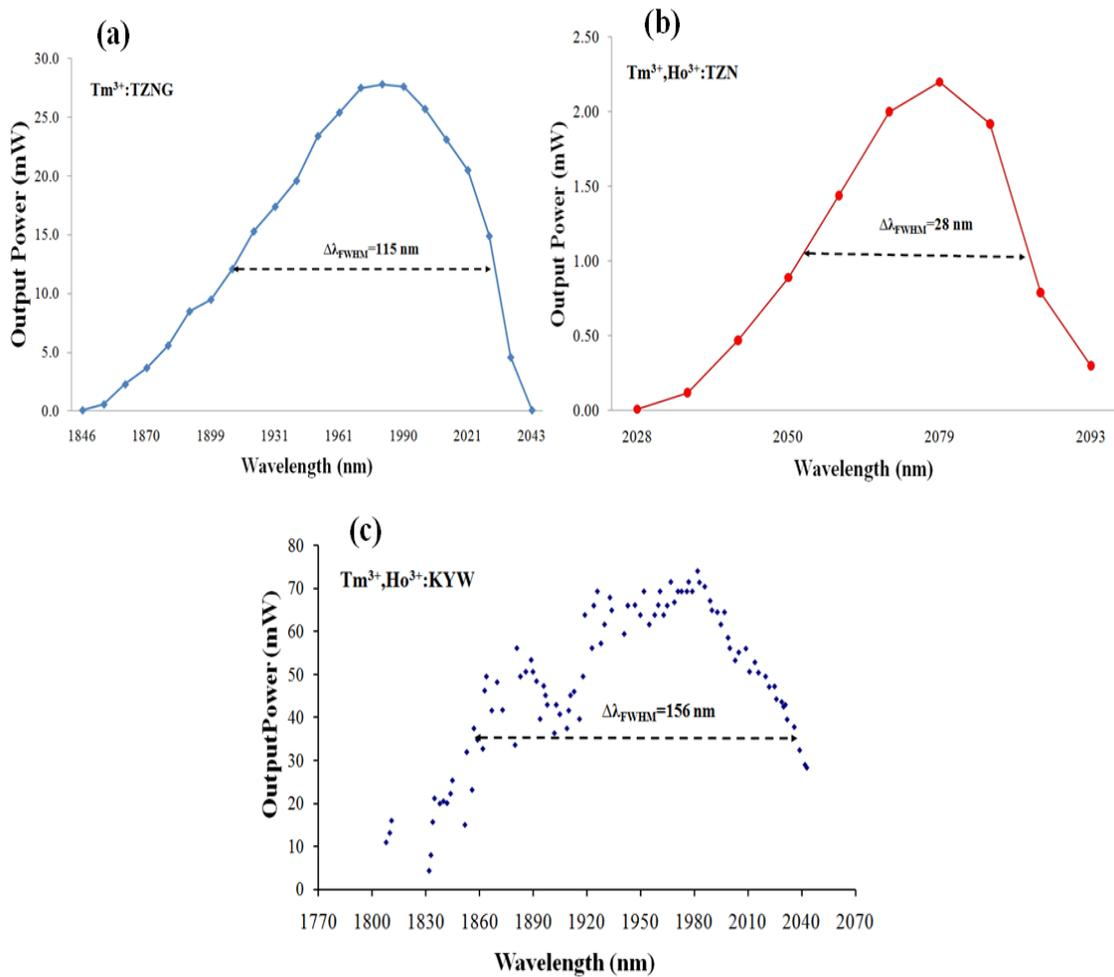
**Figure 5-16: Wavelength tuning curve results using 1% output couplers (OC) for (a)  $\text{Tm}^{3+}:\text{TZNG}$  glass, (b)  $\text{Tm}^{3+},\text{Ho}^{3+}:\text{TZN}$  glass and (c)  $\text{Tm}^{3+},\text{Ho}^{3+}:\text{KYW}$  crystal.**
