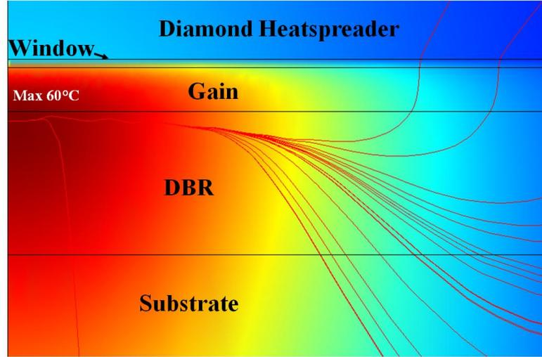
**Figure 3-5: COMSOL Multiphysics™ plot showing the simulation results for a  $\text{GaIn}_{0.33}\text{N}_{0.007}\text{As}/\text{GaN}_{0.011}\text{As}/\text{GaAs}$  SDL designed for 1220 nm operation, using  $\text{AlAs}/\text{GaAs}$  DBR and  $\text{Al}_{0.3}\text{GaAs}$  confinement window. (Darkest red region corresponds to maximum heat graduating to darker blue areas of lowest temperature.)**
