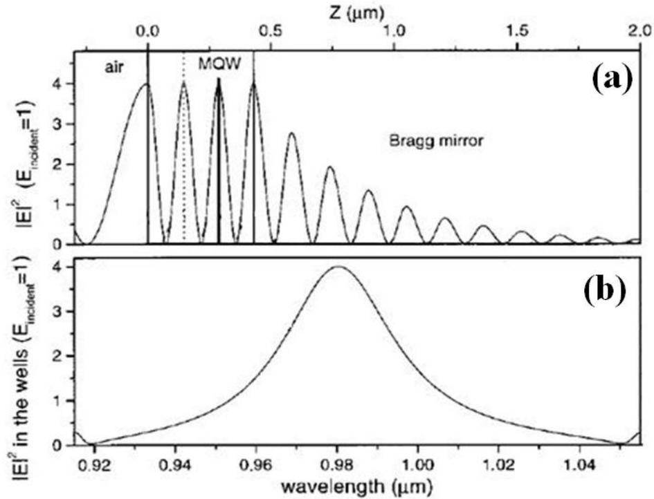
**Figure 2-15: The  $|E|^2$  field (with incident E-field normalised to 1) through the SDL structure (a) and in the QWs (b), showing an intensity peak at the design wavelength of 980 nm [30].**
