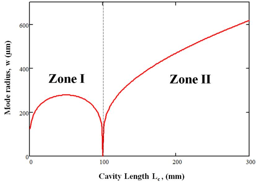
**Figure 4-12: Mathcad™ simulation of the mode radius  $w$  over a range of cavity lengths  $L_c$ , using a folding mirror radius of curvature  $R_c = 100$  mm.**
