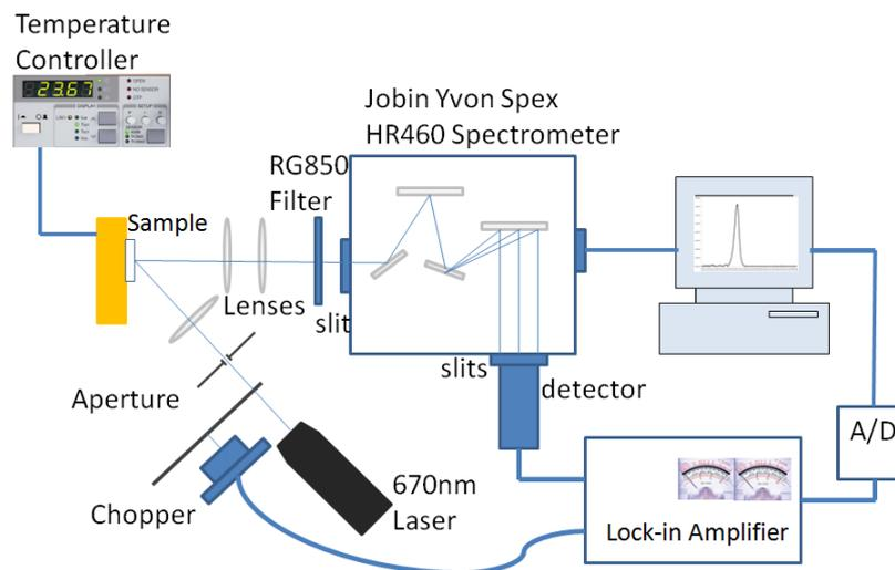
**Figure 4-6: Photoluminescence experimental setup.**
