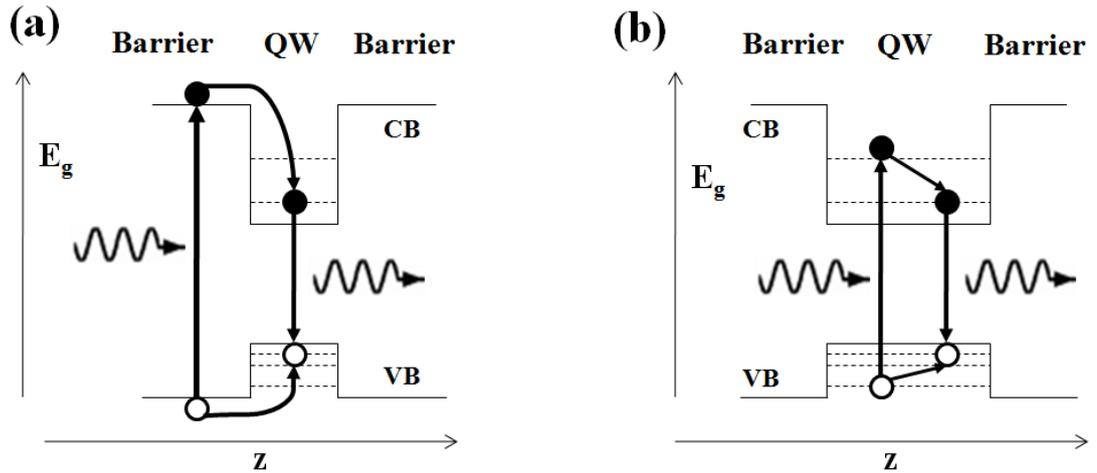
**Figure 2-19: Comparison of (a) barrier pumping regime and (b) in-well pumping.**
