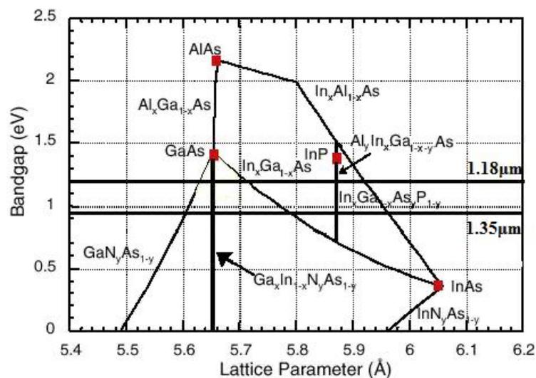
**Figure 1-6: Binary, ternary and quaternary semiconductor material systems with respect to their bandgap energy and crystal lattice parameter. Indicated is the wavelength region 1.18  $\mu\text{m}$  to 1.35  $\mu\text{m}$  [74].**
