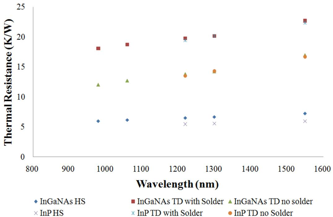
**Figure 3-8: Thermal resistance of InGaNAs and InP-based SDL devices, designed across a range of operational wavelengths implementing a heatspreader (HS), thin disk (TD) with solder and without solder, using a pump spot radius of 50  $\mu\text{m}$ .**
