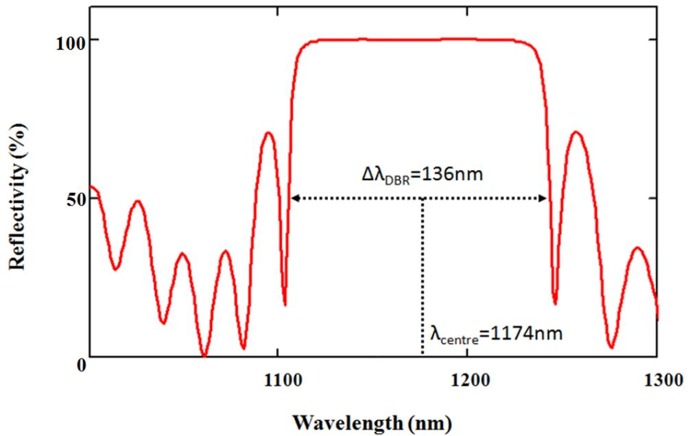
**Figure 2-2: Reflectivity of sample AsN2592 designed for 1180 nm with 25 pairs AlAs/GaAs.**
