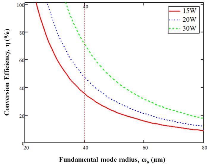
**Figur 6-9: Theoretical conversion efficiencies across a range of fundamental mode radius sizes, for powers  $P_\omega=15\text{W}$ ,  $20\text{W}$  and  $30\text{W}$ .**
