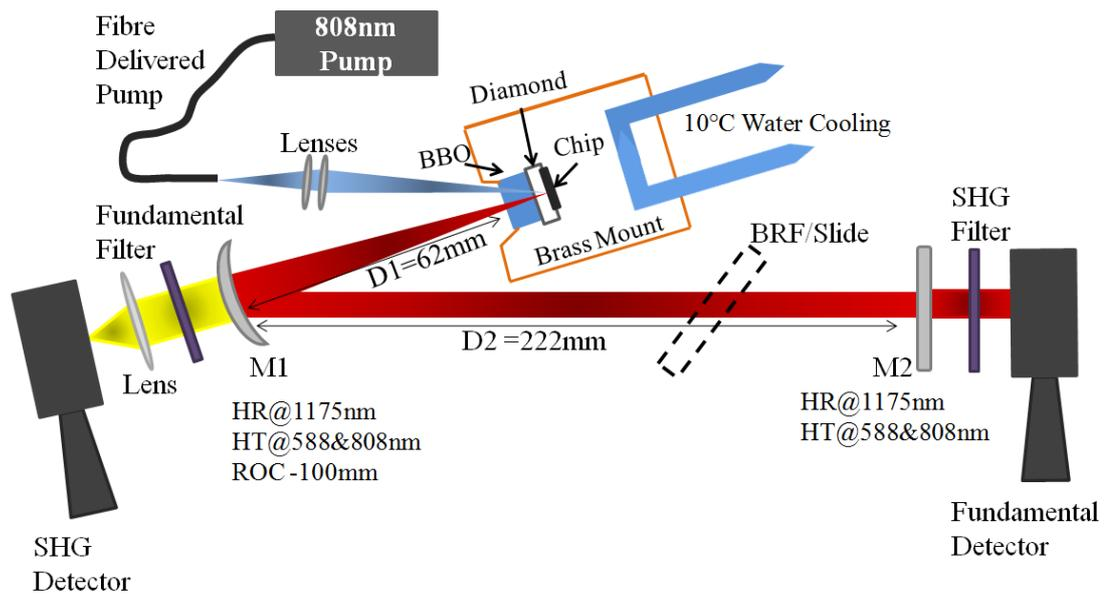
**Figure 6-15: Schematic diagram of the SDL cavity consisting of an 808nm pump diode laser, the mounted double bonded chip-diamond-BBO structure, with HR cavity mirrors M1 and M2, and the birefringent filter *BRF* in the long arm of the cavity.**
