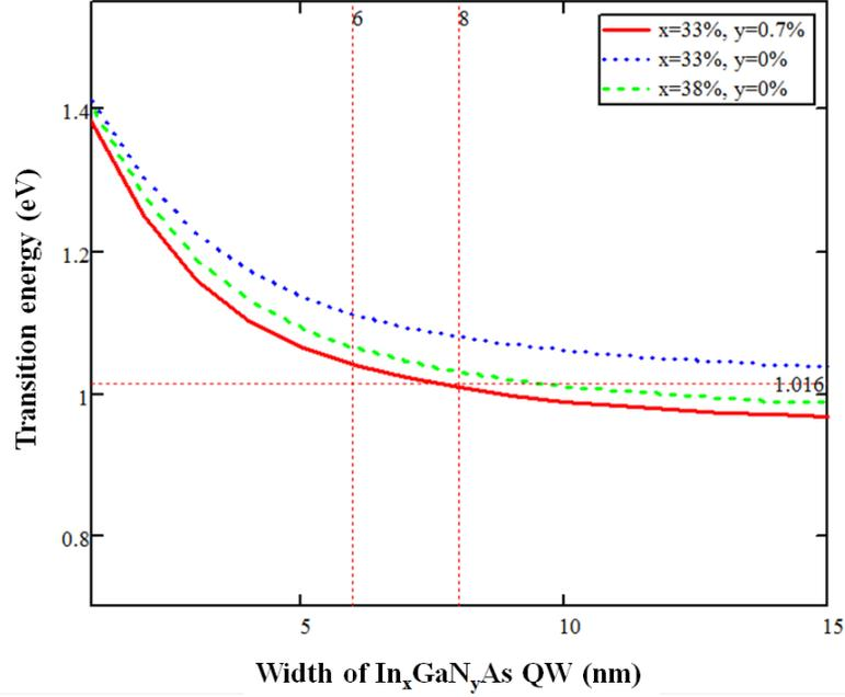
**Figure 2-7: Transition energy over a range of QW lengths, to compare GaIn<sub>0.33</sub>N<sub>0.007</sub>As (solid red), In<sub>0.33</sub>GaAs (dashed blue) and In<sub>0.38</sub>GaAs (dashed green). The marker line is the emission energy 1.016 eV (1220 nm).**
