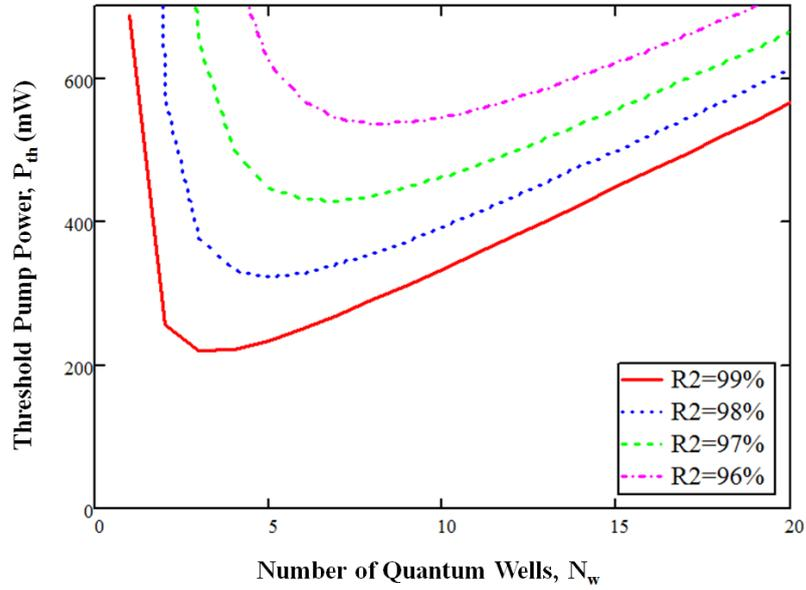
**Figure 2-21: Threshold pump power with respect to Number of QWs for output coupler reflectivity values of 99%, 98%, 97% and 96%.**
