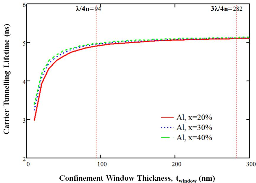
**Figure 2-23: Tunneling rate of carriers from the gain region into the confinement window, as a function of the barrier thickness.**
