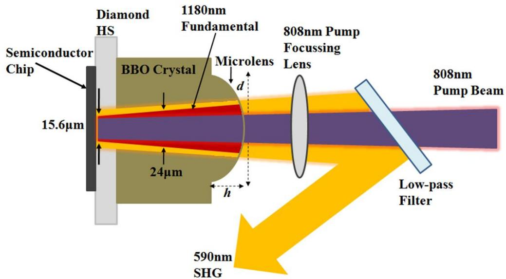
**Figure 6-10: Microchip configuration indicating an 808nm pump beam (*purple*) at normal incidence focused onto the semiconductor chip, with the 1180 nm fundamental (*red*) within the micro-cavity and the 590 nm (*orange*) SHG output.**
