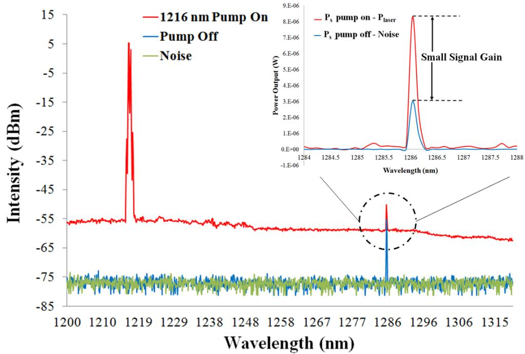
**Figure 5-24: Spectra measured using the OSA with a resolution of 0.06 nm, showing the 1216 nm SDL pump, 1286 nm signal and noise level measured in the absence of both signal and pump. Inset is the result showing the small signal gain, found through the difference between the ( $P_s$  with pump on -  $P_{laser}$ ) and ( $P_s$  with pump off- Noise).**
