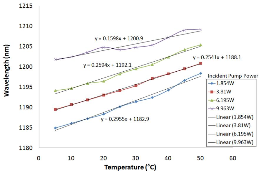
**Figure 4-31: Wavelength variation across all temperatures at different incident pump powers.**
