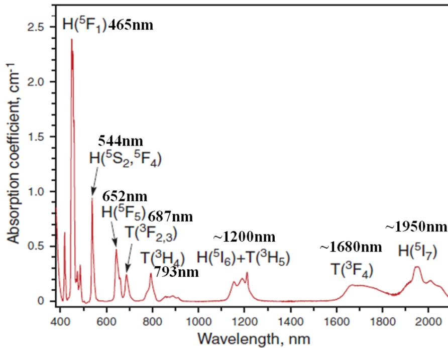
Figure 5-2: Absorption coefficient spectra for the Tm2%wt,Ho0.2%wt:TZN bulk glass sample [23].
