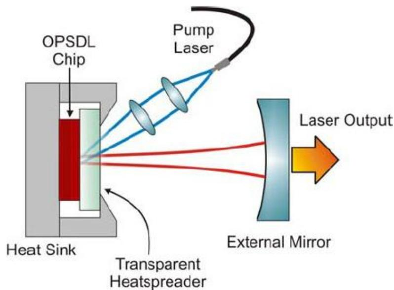
**Figure 1-2: General form of an optically pumped Semiconductor Disk Laser (OPSDL) [63].**
