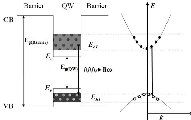
**Figure 1-7: Quantum well structure showing the energies  $E_c$  and  $E_v$  of the conduction band (CB) and valence band (VB) edges respectively, and the bandgaps of the barrier  $E_{g(\text{Barrier})}$  and QW  $E_{g(\text{QW})}$  with photon emission  $\hbar\omega$  from  $e1$ - $h1$  transitions between the quantized energy bands within the well, and the reciprocal energy dispersion in  $k$ -space.**
