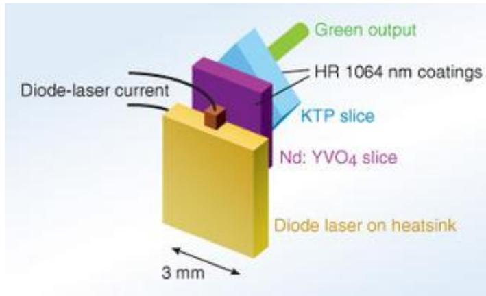
**Figure 1-4: Diode pumped solid-state laser (DPSS) comprising Nd:YVO<sub>4</sub> gain material, with KTP doubling crystal to produce green (532nm) laser output [71].**
