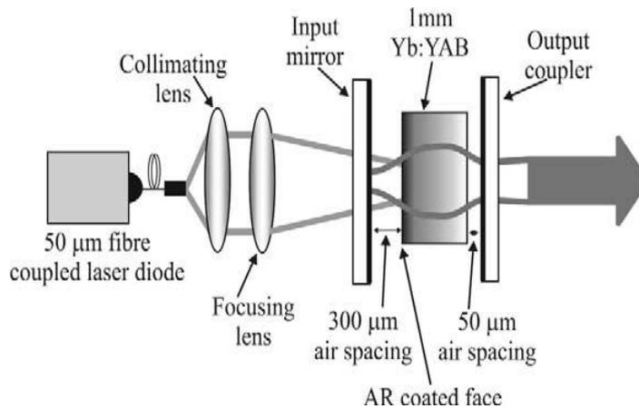
**Figure 1-5: Schematic of diode pumped Yb:YAB self-frequency doubled laser developed by Burns et al [72].**
