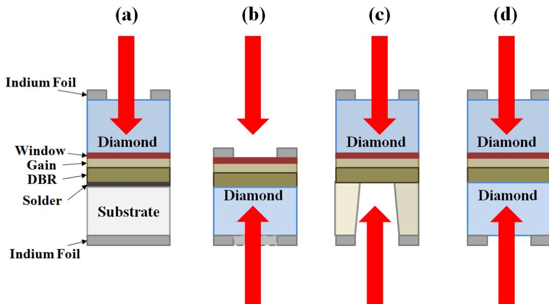
**Figure 3-9:** (a) Front pumped device employing a diamond heatspreader and soldered onto the substrate, (b) thin disk device front or end pumped, (c) thin disk device with the substrate which can be partially removed (*end pumped via hole*) or fully removed (*front pumped*) and (d) thin disk device ‘sandwiched’ between diamond heatspreaders front or end pumped [28].
