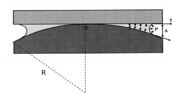
**Figure 3-13: Illustration of forces due to stress exerted between two surfaces  $T'$  and the hydrostatic pressure  $P$  during liquid capillary bonding [38], with the radius of curvature  $R$  of the material.**
