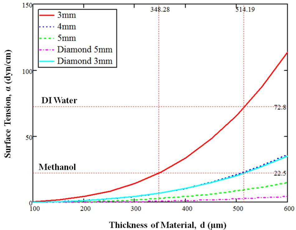
**Figure 3-14: The surface tension of GaAs based material across a range of thicknesses, for lengths  $L=3\text{mm}, 4\text{mm}$  and  $5\text{mm}$  and of diamond heatspreader having length of 3mm and 5mm. Indicated are the surface tension values for DI water ( $72.8\text{dyn/cm}$ ) and Methanol ( $22.5 \text{ dyn/cm}$ ).**
