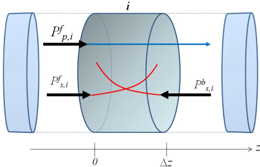
**Figure 5-19:** Schematic of the silica fibre in a section  $i$  over a distance  $\Delta z$ , in which the forward pump power  $P_{p,i}^f$  and the signal power in the forward direction  $P_{s,i}^f$  and backwards direction  $P_{s,i}^b$  are shown.
