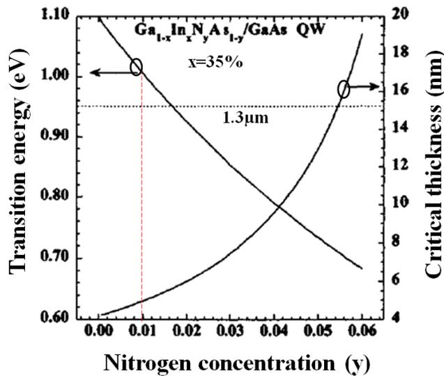
**Figure 2-13: Transition energies and critical thicknesses for a GaIn<sub>0.35</sub>N<sub>y</sub>As/GaAs QW across a range of nitrogen concentrations ( $y$ ) [24]. Indicated is 1.3  $\mu\text{m}$  emission and  $y=1\%$ .**
