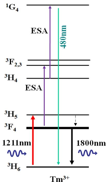
**Figure 5-5:**  $\text{Tm}^{3+}$  energy transitions using a 1211 nm excitation source, with excited-state absorption (ESA) (purple lines), and emission transitions of 480 nm and  $\sim 1800$  nm.
