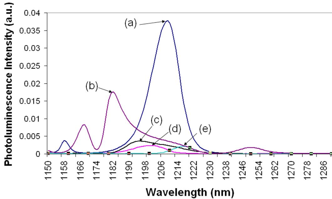
**Figure 4-9: Photoluminescence intensity profiles comparing 5 different structures; (a) 4QW GaInAs Vn1381, (b) 6QW GaInNAs Vn1567, (c) 4QW GaInNAs Vn1534, (d) 8QW GaInAs Vn1399 and (e) 8QW GaInNAs Vn1536.**
