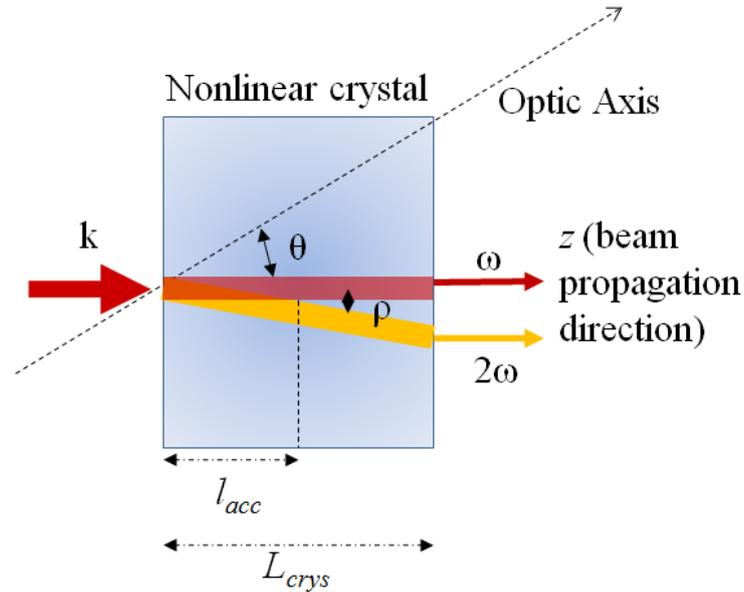
**Figure 6-4: The beam walk-off angle  $\rho$  with respect to the phase matching angle  $\theta$  and the optic axis in a nonlinear crystal, where the input  $k$  wavevector and fundamental frequency  $\omega$  with frequency doubled  $2\omega$  outputs. The acceptance length,  $l_{acc}$  indicated is the length before the frequency doubled beam ‘walks-off’ the fundamental beam.**
