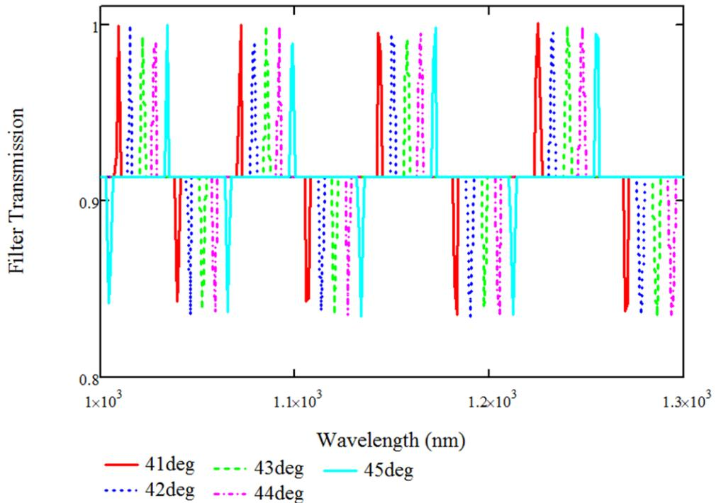
**Figure 4-22: Transmission of a 4 mm BRF with rotational angles  $\phi = 41^\circ - 45^\circ$ .**
