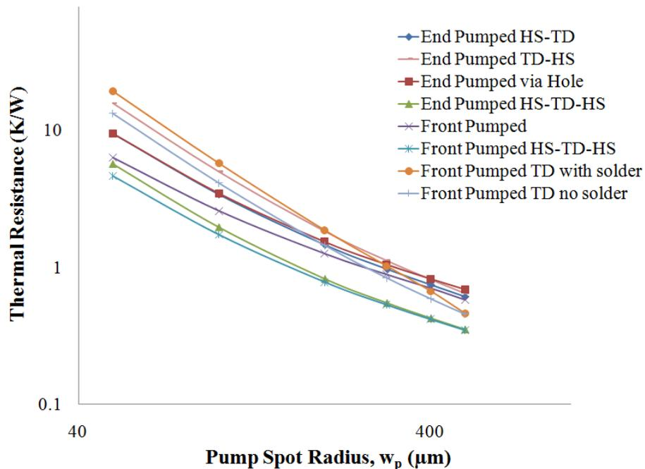
**Figure 3-12: Pump-dependent average thermal resistances for both front and end pumped architectures, using InGaAs/GaAs 1060 nm designed devices with the diamond heatspreader (HS) and /or thin disk (TD) approaches.**
