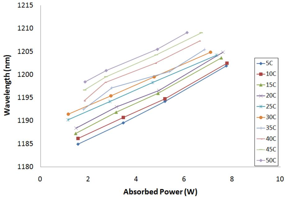
**Figure 4-30: Wavelength variation with respect to the absorbed power across all temperatures.**
