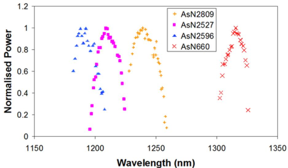
**Figure 4-27: Wavelength tuning ranges for SDL devices *AsN2596* (1190 nm), *AsN2527* (1220 nm), *AsN2809* (1230 nm) and *AsN660* (1300 nm).**
