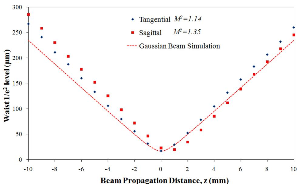
**Figure 5-12:  $M^2$  measurements for  $AsN2527$  1220 nm SDL with cavity dimensions  $D1=59$  mm and  $D2=225$  mm.**
