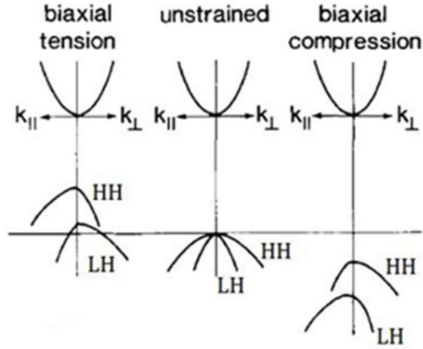
**Figure 2-12: Effects of strain on the band structure of a zinc-blende crystal, indicating the heavy-hole (HH) and light-hole (LH) valence band degeneracy [25].**
