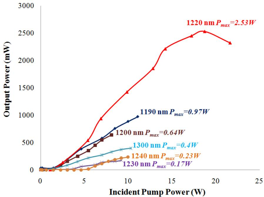
**Figure 4-15: Highest achieved power transfer curves for all devices measured, indicating the device design wavelengths.**
