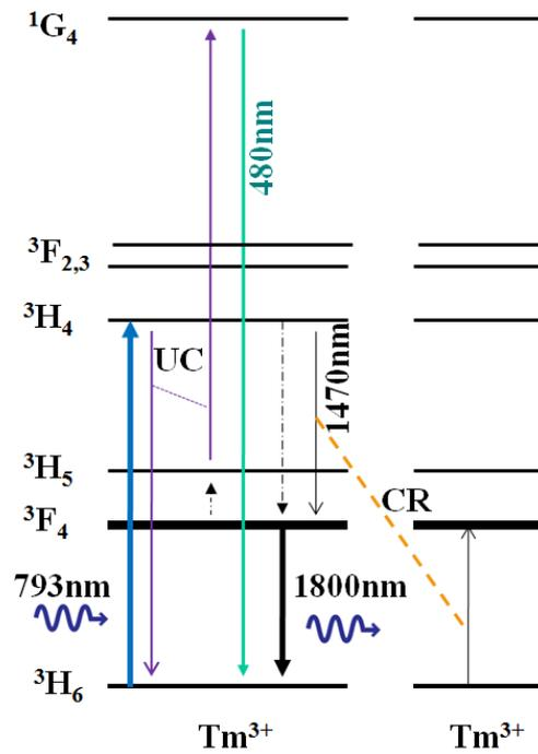
**Figure 5-3: Tm<sup>3+</sup> energy transitions from a 793 nm excitation source, with upconversion (UC) processes (purple), nonradiative decay (black dashed), cross-relaxation (CR) (orange dashed) and emission transitions of 480 nm, 1470 nm and 1800 nm.**
