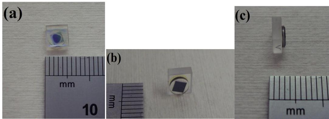
**Figure 6-14: (a) Top view of the double bond between AsN2906 GaInNAs/GaAs semiconductor chip, diamond heatspreader and the  $\beta$ -BBO crystal, (b) back view of the device and (c) side view with the marked 'arrow' on the side indicating the AR@1180&590&808nm coating.**
