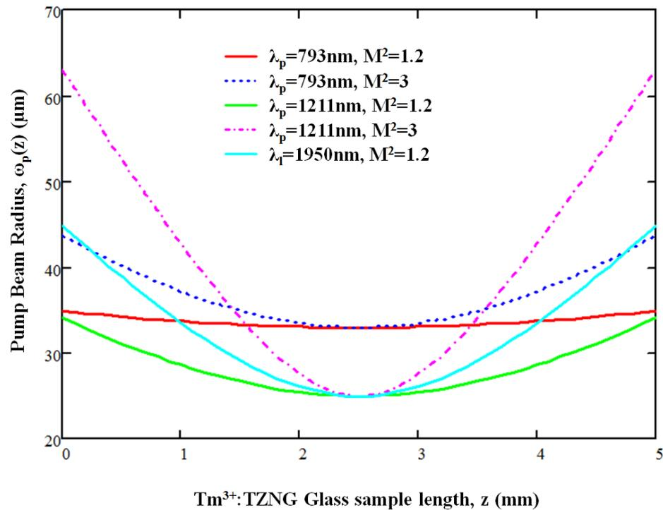
**Figure 5-17: Comparison of 793 nm and 1211 nm pumping, with varying  $M^2$  parameters showing the pump beam radii inside the  $\text{Tm}^{3+}$ :TZNG glass sample of length 5 mm. Included is the 1950 nm laser beam profile through the crystal with  $M^2=1.2$ .**
