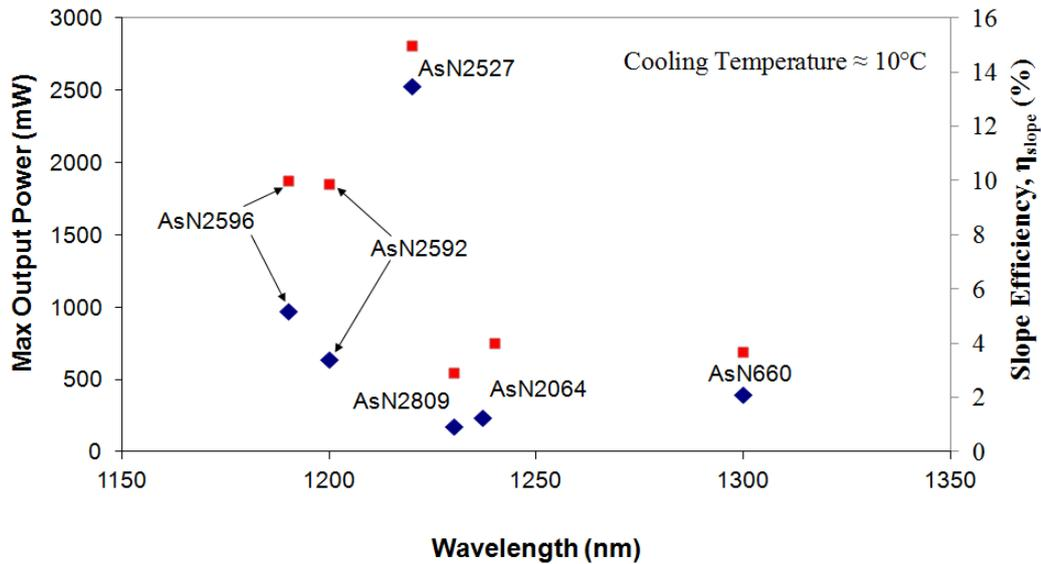
**Figure 4-16: Comparison of maximum output powers (*blue diamond*) and slope efficiencies (*red squares*) for all samples.**
