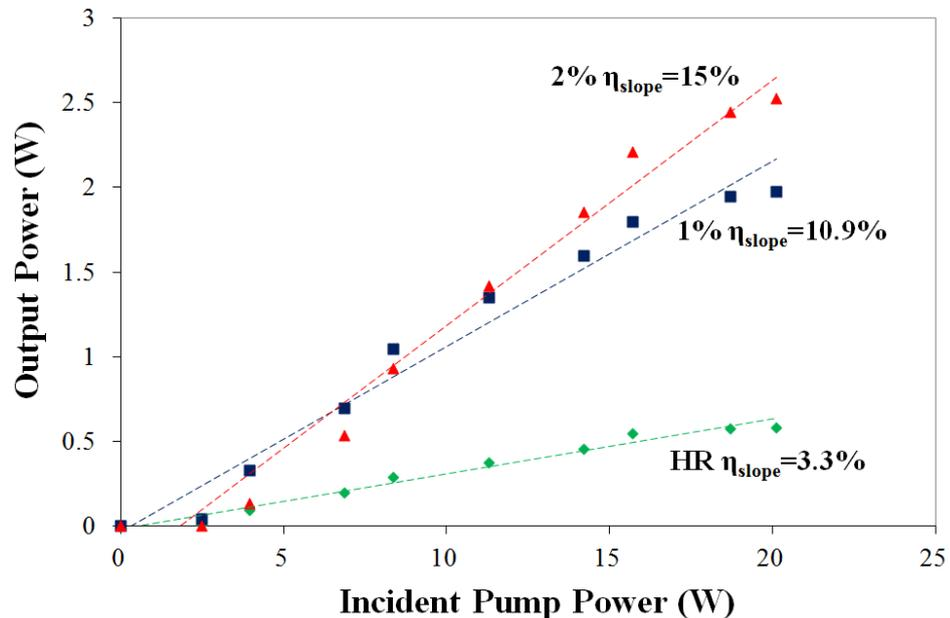
Figure 4-14: Power transfer curves of AsN2527 1220nm SDL with Output Couplers (OC) High Reflectance (HR), 1% and 2% transmissions.
