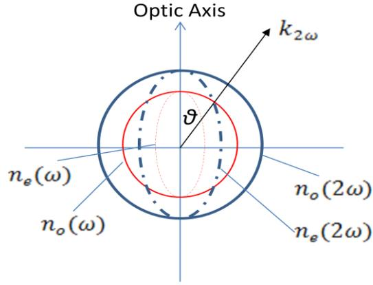
**Figure 6-2: Refractive index ellipsoid indicating the ordinary and extraordinary indices for the fundamental,  $\omega$  and doubled frequency,  $2\omega$ . Included is the frequency doubled propagating wave vector,  $k_{2\omega}$  and its phase matching angle  $\theta$  with the optic axis.**
