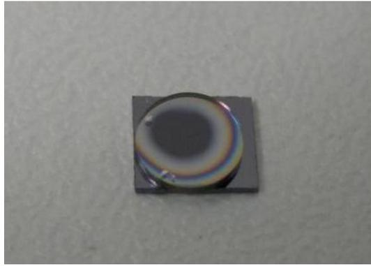
**Figure 3-15: 1180 nm Sample *AnN2596* bonded to CVD synthetic diamond.**
