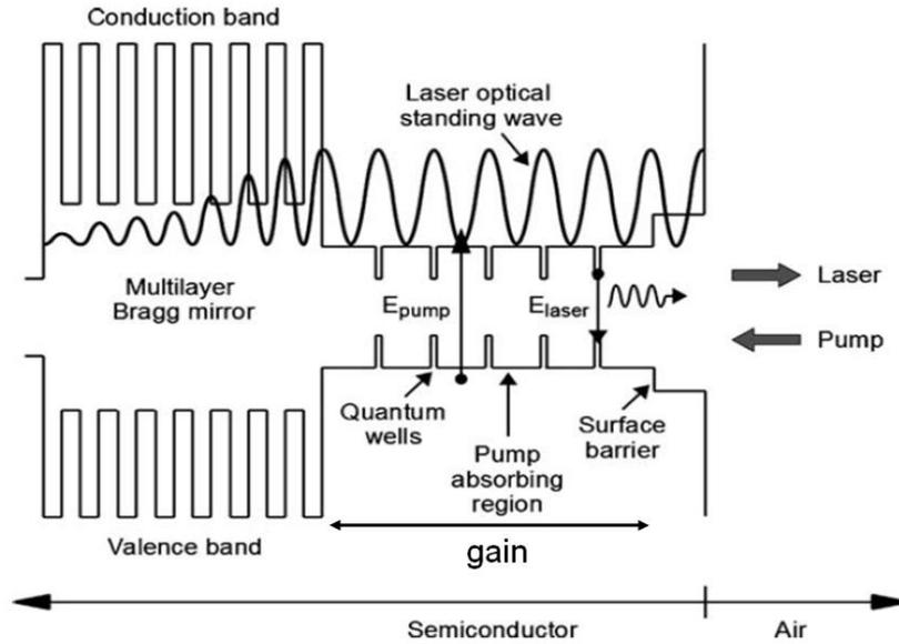
**Figure 2-1: General structure of an SDL including the Bragg mirror, active region containing the quantum wells and the surface barrier comprising the confinement window and cap [1].**
