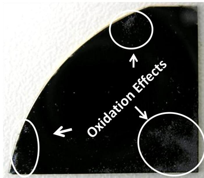
**Figure 2-24: Samsung sample K732 1047nm indicating the result of oxidation on the surface of the semiconductor wafer.**
