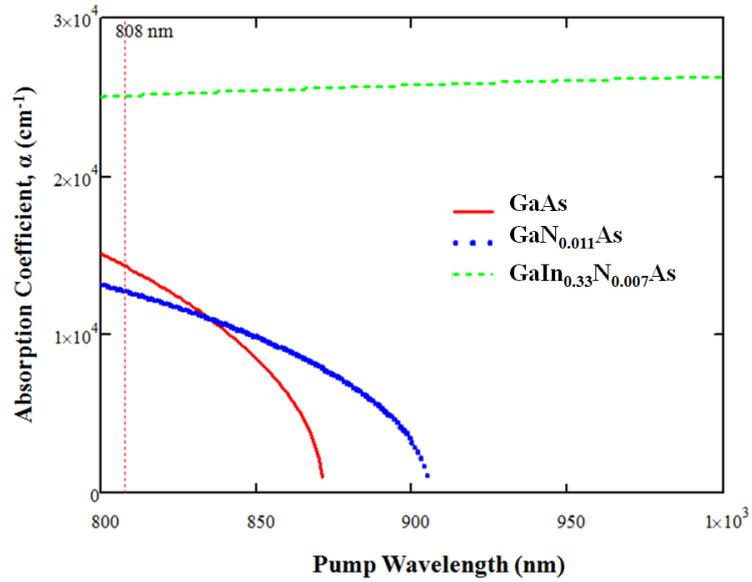
**Figure 3-3: Absorption coefficients for GaAs, GaNAs and GaInNAs over a range of pump wavelengths.**
