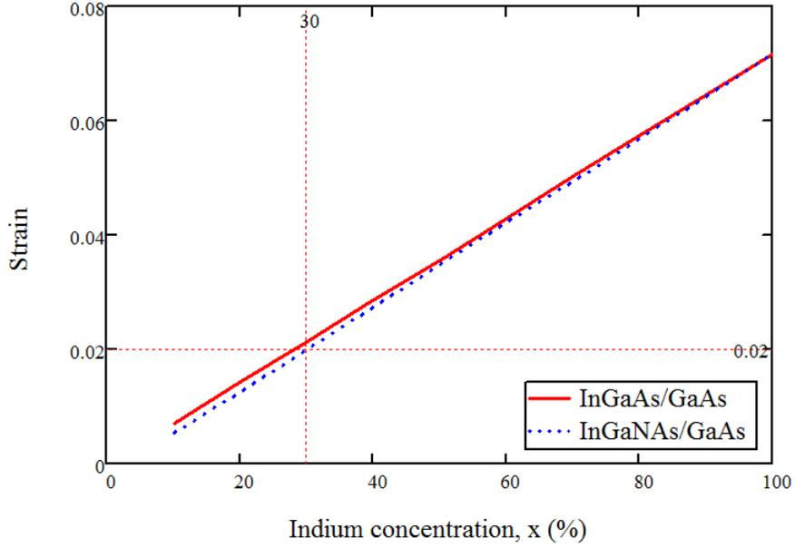
**Figure 2-9: The compressive strain experienced in an  $\text{In}_x\text{GaAs}/\text{GaAs}$  material system compared to that of  $\text{In}_x\text{GaN}_{0.01}\text{As}/\text{GaAs}$  with increasing indium concentrations.**
