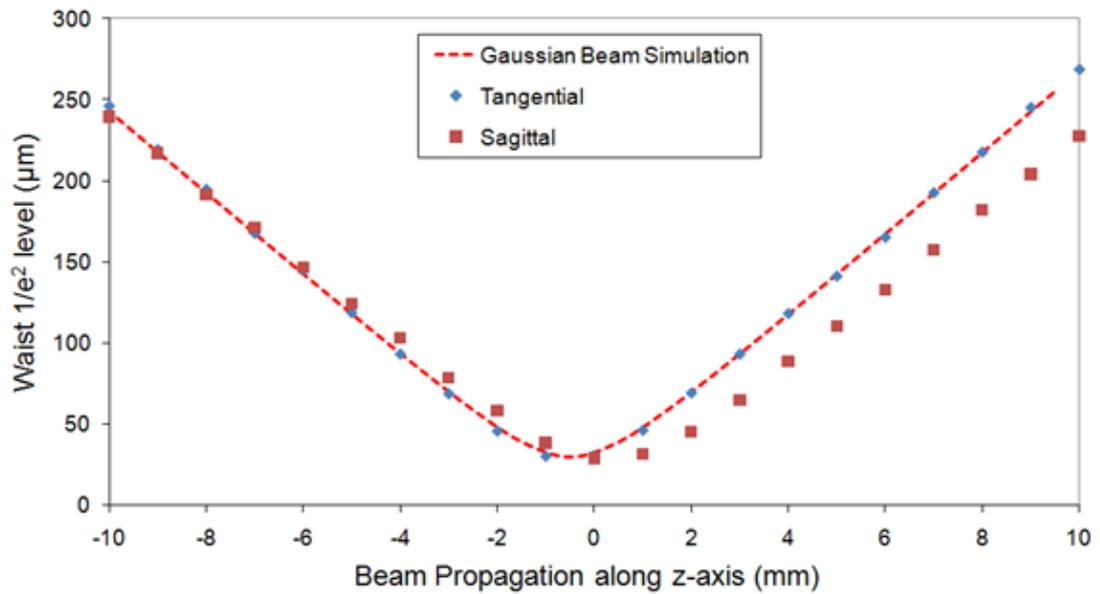
**Figure 4-20: Beam profile plots for the tangential  $M^2 \approx 2$  and sagittal  $M^2 \approx 1.7$ , compared with the Gaussian beam.**
