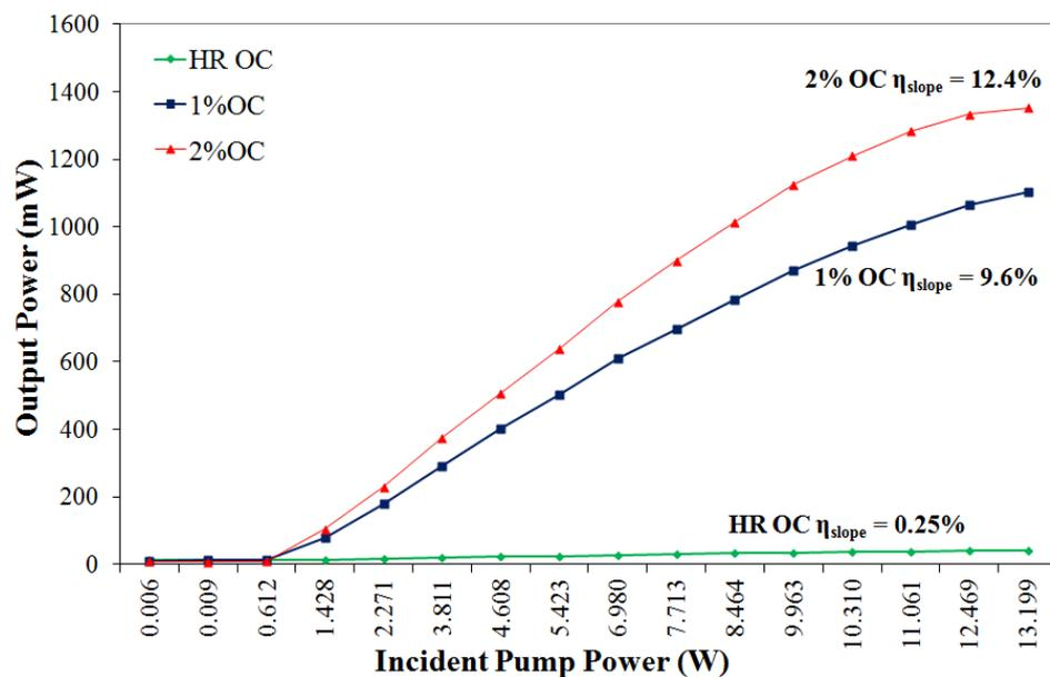
**Figure 5-9: Power transfer curves of *AsN2527* 1220 nm SDL with Output Couplers (OC) High Reflectance (HR), 1% and 2% transmissions.**
