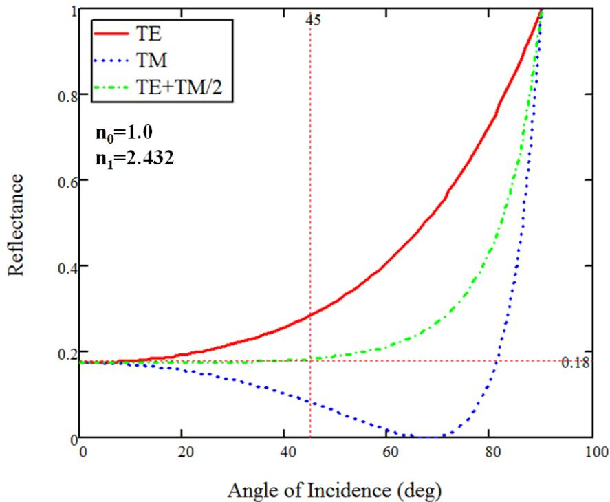
**Figure 4-28: Reflectance of TE, TM and average TE+TM/2 of an incident beam from air,  $n=1$  to a CVD diamond heatspreader  $n=2.432$  over a range of incident angles.**
