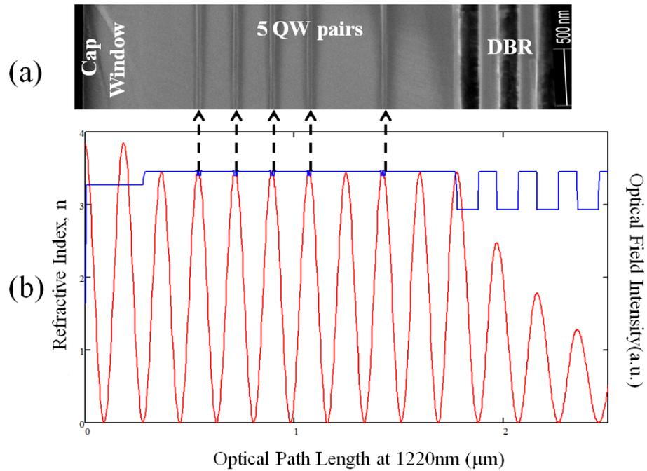
**Figure 2-18: (a) The SEM image of AsN2527 1220 nm structure to align with (b) the design profile of the same structure with the refractive index of the layers (*blue*) and the optical field intensity (*red*) illustrating the QW positioned at the anti-nodes of the field intensity.**
