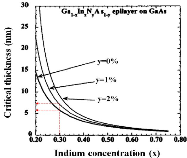
**Figure 2-11: Critical thickness for  $\text{In}_x\text{Ga}_{1-x}\text{N}_y\text{As}_{1-y}/\text{GaAs}$ , with comparison made between nitrogen inclusion of 0%, 1% and 2% [24].**
