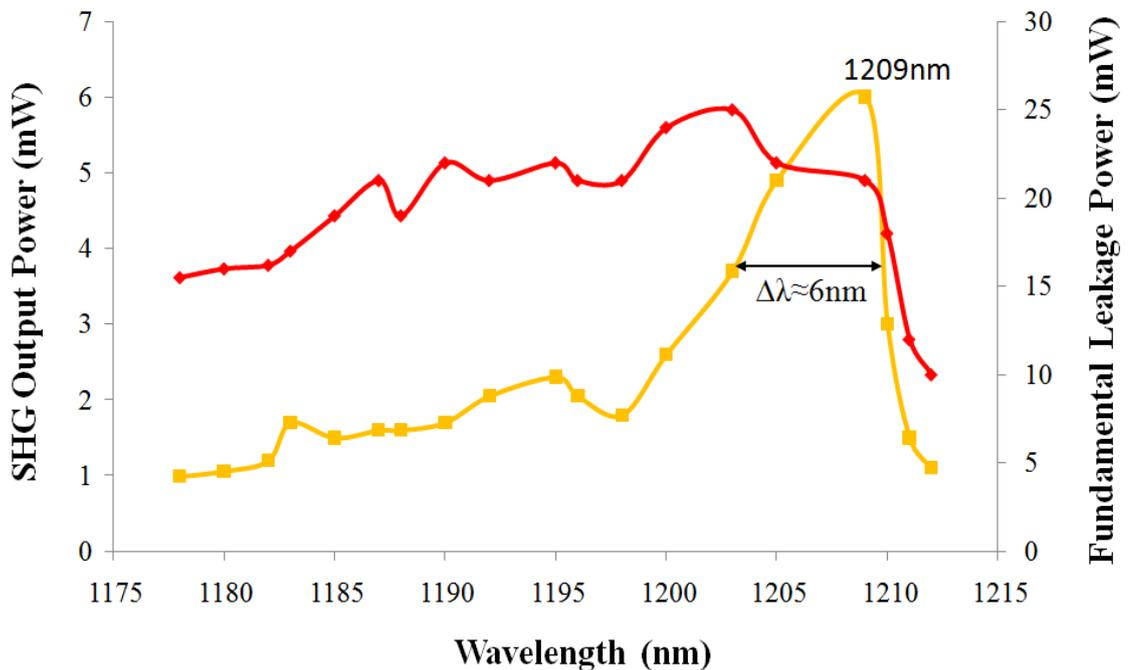
**Figure 6-21: Graph of wavelength tuning using a 4 mm thick BRF.**
