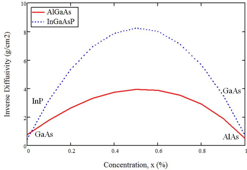
**Figure 3-7: Inverse thermal diffusivity of  $\text{Al}_x\text{GaAs}$  (red solid) compared with  $(\text{GaAs})_x(\text{InP})_{1-x}$  (blue dashed), with the extreme ends of the curve corresponding to GaAs/AlAs and InP/GaAs respectively [22].**
