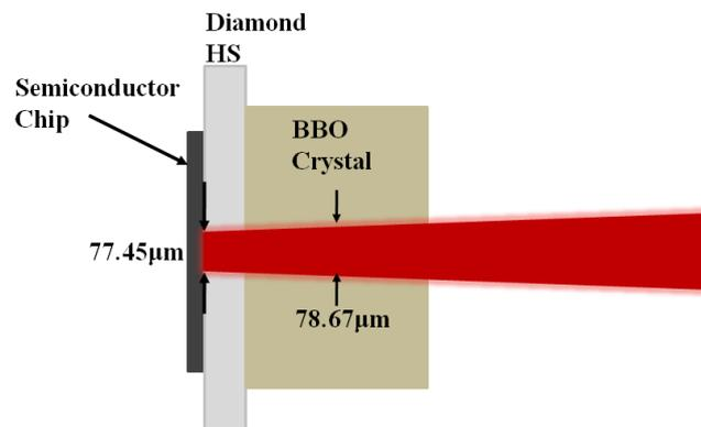
**Figure 6-8: Beam incident onto the semiconductor chip, and at the centre of the BBO crystal, indicating the beam diameters.**
