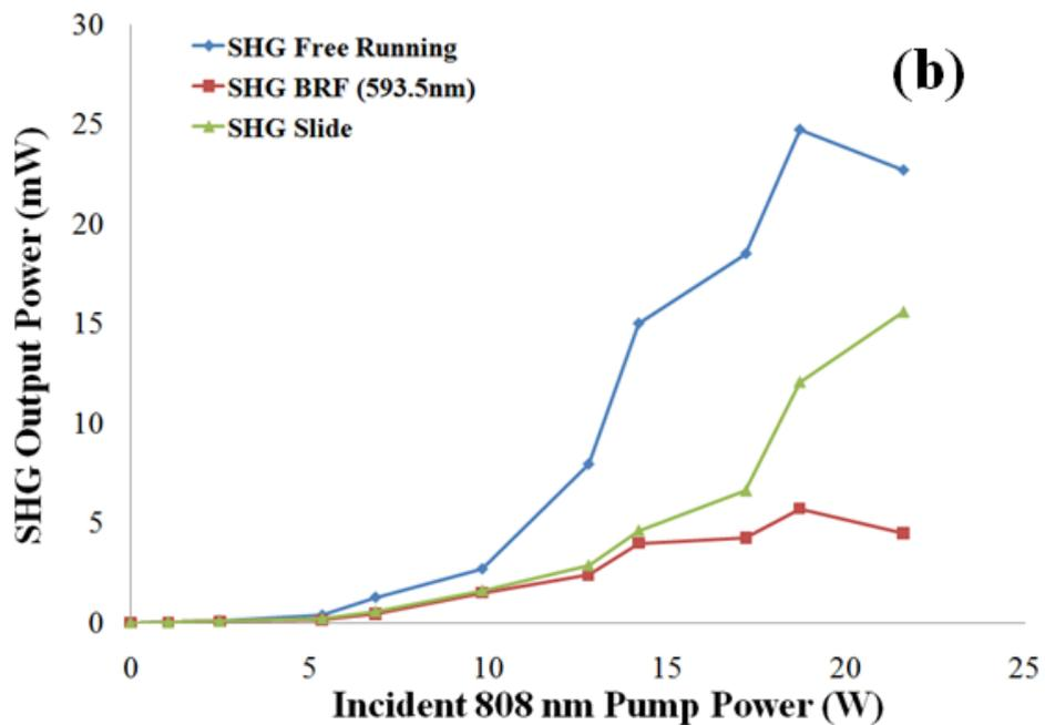
**Figure 6-22: Power transfer curves for the (a) fundamental and (b) SHG, in free running mode, wavelength tuned using the BRF to 1187 nm (fundamental frequency) and with an uncoated slide.**
