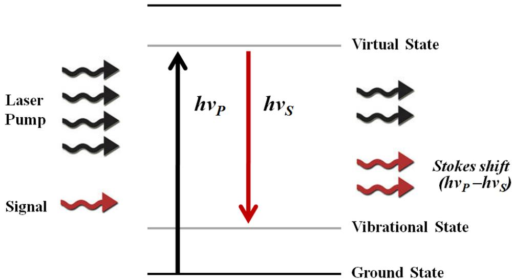
**Figure 5-18: Schematic of the stimulated Raman scattering process.**
