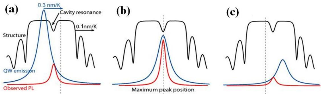
**Figure 2-16: (a) Shift rates of the RPG cavity resonance compared with QW emission, indicating also the observed PL, (b) the maximum PL intensity at the optimal operating temperature, when the RPG cavity resonance and QW emission are aligned, and (c) the rapid decrease in PL and QW emission as the mismatch increases.**
