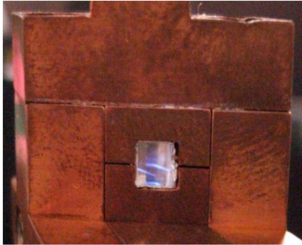
**Figure 5-6:  $\text{Tm}^{3+}$ :TZNG glass sample in a brass mount, with visible blue fluorescence due to upconversion along the incident pump radiation within the glass.**
