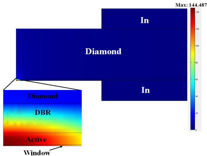
**Figure 3-11: End pumped simulation with the diamond bonded onto the back of the thin disk SDL.**
