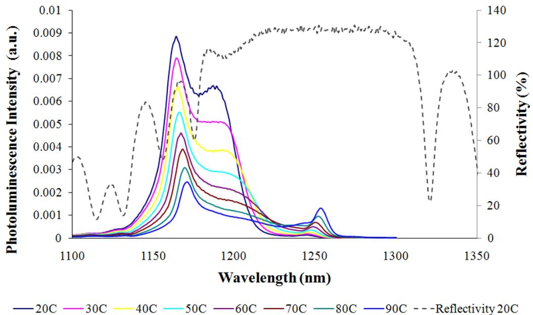
**Figure 4-4: Edge PL for AsN2527 1220 nm sample, from 20°C to 90°C, with an included Reflectivity spectrum measurement at 20°C.**
