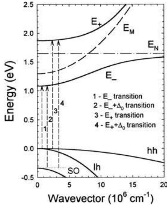
**Figure 1-8: Energy band splitting into  $E_+$  and  $E_-$  bands, indicating the  $N$  impurity level energy band  $E_N$  and host energy level  $E_M$ . The transitions between the light/heavy hole and spin-orbital split-off valence bands in relation to the  $E_+$  and  $E_-$  bands are shown. [112]**
