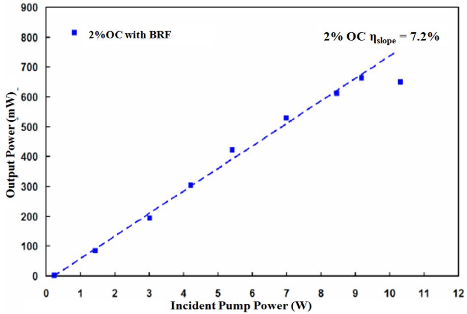
**Figure 5-10: Power transfer results of the SDL with an intracavity birefringent filter (BRF), tuned to 1212 nm.**
