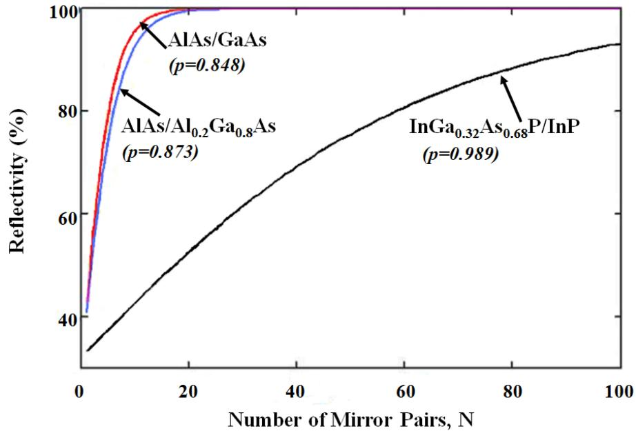
**Figure 2-4: Reflectivity with respect to the number of mirror pairs for AlAs/GaAs (red), AlAs/AlGaAs (blue) and InGaAsP/InP (black) having a bandgap energy  $E_g=0.91$  eV [4] ( $\lambda_B=1300$ nm).**
