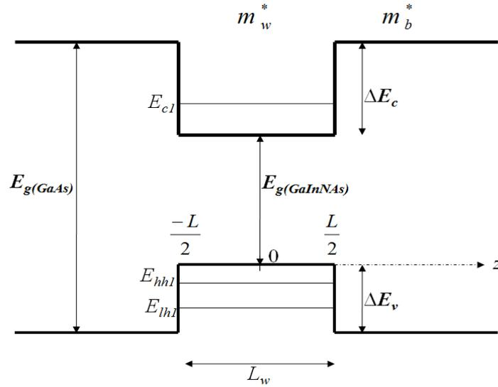
**Figure 2-6: GaInNAs QW of width  $L_w$  with GaAs barriers, indicating the bandgap energies  $E_{g(\text{GaAs})}$  and  $E_{g(\text{GaInNAs})}$ , effective masses in the well  $m_w^*$  and the barrier  $m_b^*$ , the differences in conduction band edge  $\Delta E_c$  and valence band  $\Delta E_v$ , with the subband energy levels  $E_{c1}$ ,  $E_{hh1}$ , and  $E_{lh1}$  (where  $c$ =conduction band,  $hh$ =heavy hole and  $lh$ =light hole).**
