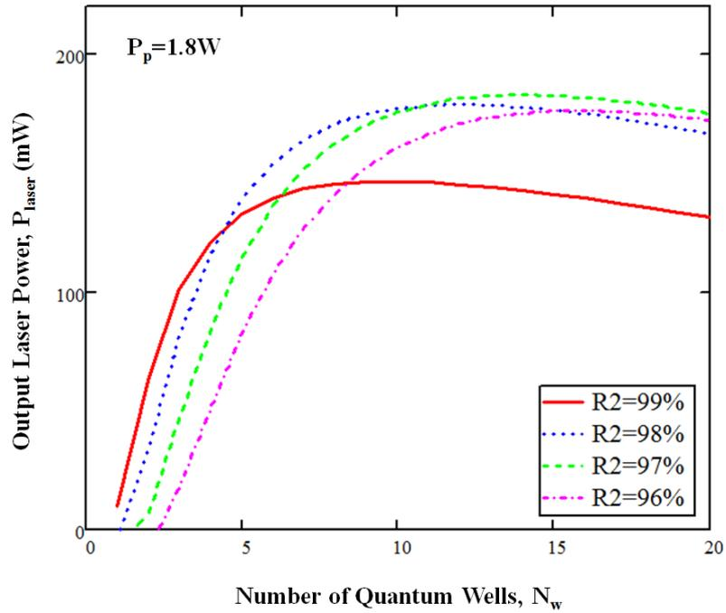
**Figure 2-22: Output laser power as a function of the number of QWs over output coupler reflectivity 99%, 98%, 97% and 96%.**
