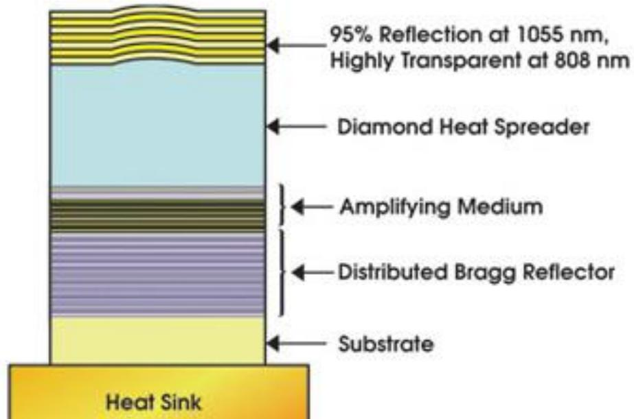
**Figure 1-3: Illustration of plano-concave microchip SDL design [67].**
