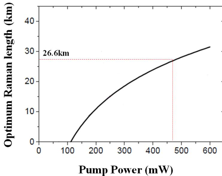
**Figure 5-21: Optimum Raman fibre length as a function of pump power.**
