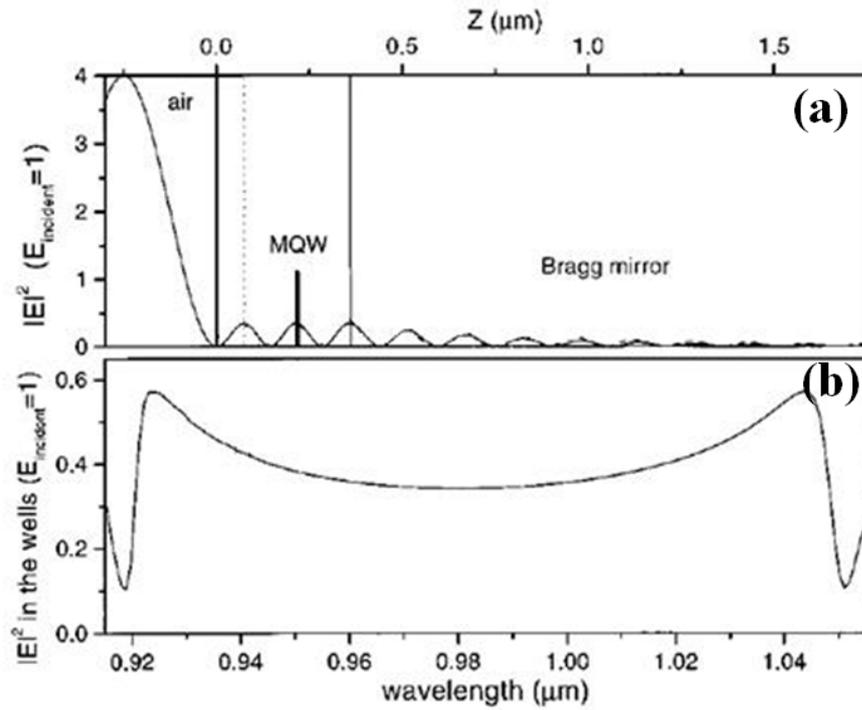
**Figure 2-17: (a) The  $|E|^2$  field (with the incident E-field normalised to 1) along the SDL device for an anti-resonant design, and (b) the  $|E|^2$  field in the wells is a minimum at the design wavelength 980 nm [30].**
