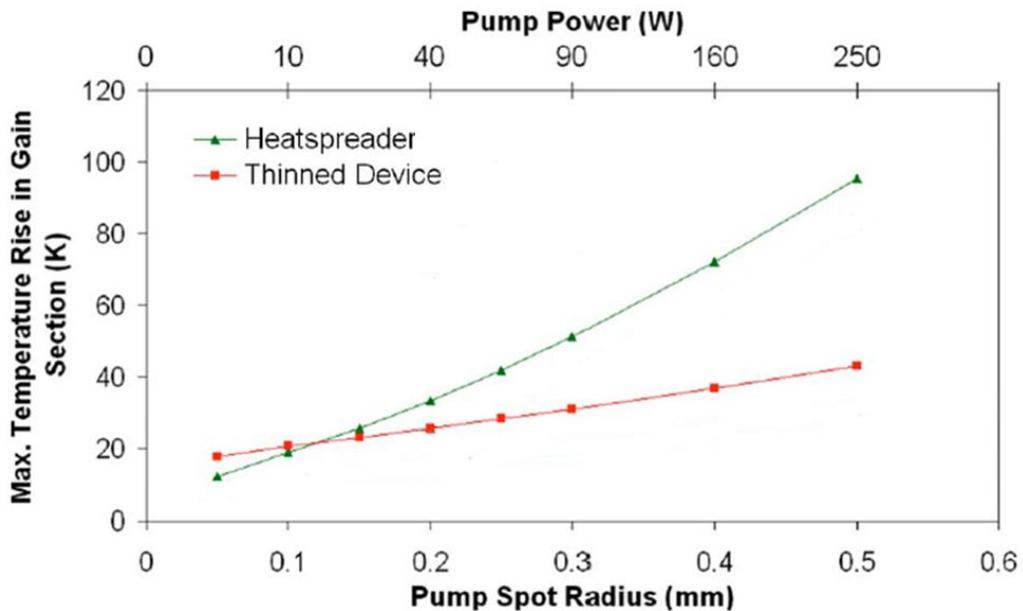
**Figure 3-1: Graph of temperature rises in the gain section employing the thin disk (*thinned device*) or heatspreader thermal management techniques, for increasing pump spot radii at constant power intensity of 32 W/cm<sup>2</sup> [10].**
