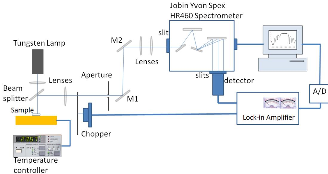
**Figure 4-1: Reflectivity experimental setup.**
