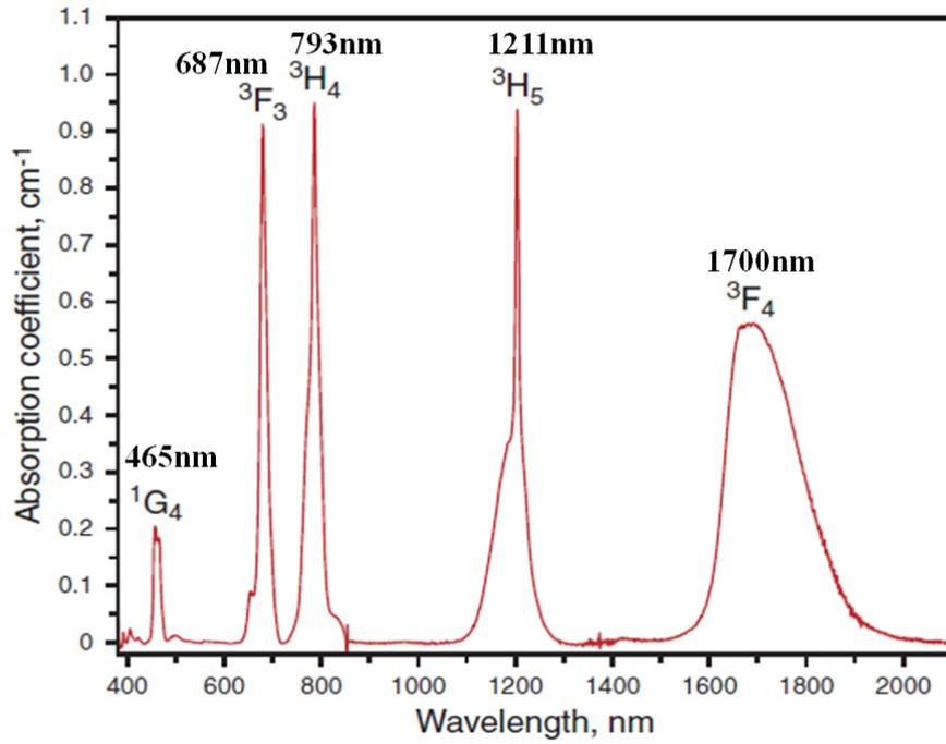
Figure 5-1: Absorption coefficient spectra for the Tm2%wt:TZNG bulk glass sample indicating the energy transitions and respective wavelengths [23].
