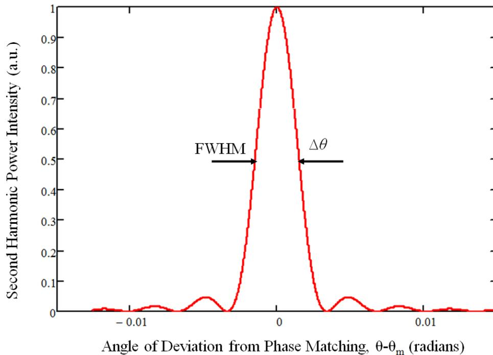
**Figure 6-5: Second harmonic power as a function of the deviation from the phase matching angle.**
