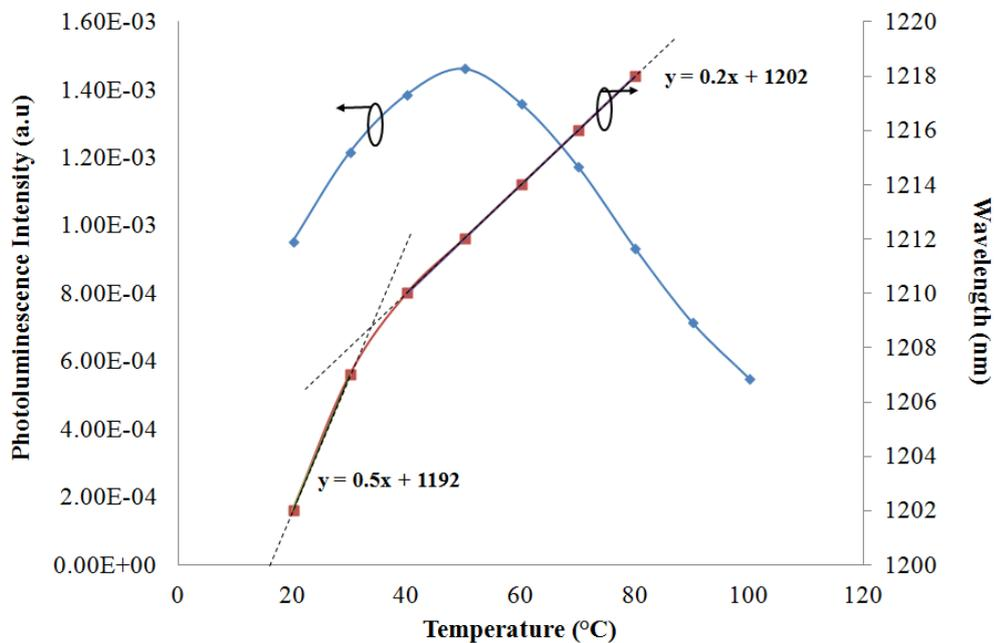
**Figure 4-8: PL intensity and wavelength shift with respect to increasing temperature.**
