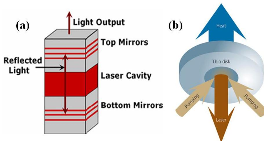
**Figure 1-1: Schematic of (a) Vertical-Cavity Surface-Emitting Laser (VCSEL) [61] and (b) solid-state optically pumped thin disk laser[62].**
