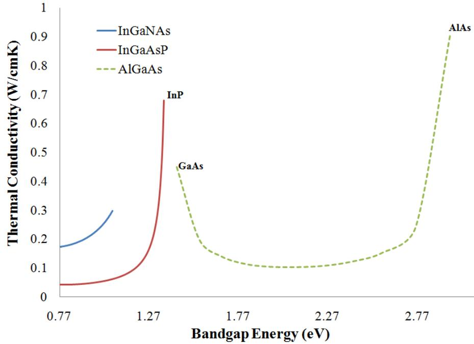
**Figure 3-6: Thermal conductivity comparing materials systems InGaNaNs, InGaAsP and AlGaAs.**
