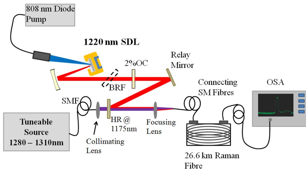
Figure 5-23: Raman amplification setup. The optically pumped V-cavity SDL uses a 2% output coupler (OC) and intracavity birefringent filter (BRF). The tuneable source and pump beams are coupled into a single mode fibre (SMF), which has been connected to the 26.6km Raman fibre with the output collected by the optical spectrum analyser (OSA).
