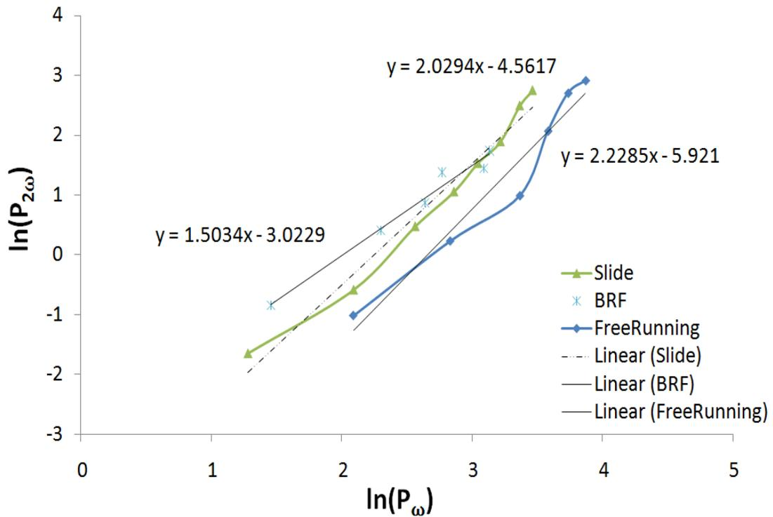
Figure 6-23: Graph of the relationship between the  $\ln(P_\omega)$  and  $\ln(P_{2\omega})$  for the free running laser, an uncoated slide and a BRF tuned to 1187nm wavelength. The linear regression of this data provides the slope to evaluate  $\ln(I_{2\omega}) = a\ln(I_\omega) + \ln(\sigma)$ .
