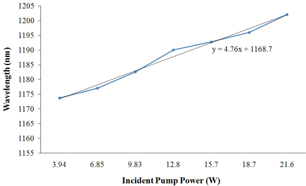
**Figure 6-19: Wavelength shift with increasing incident pump power for free running fundamental output from the SDL.**
