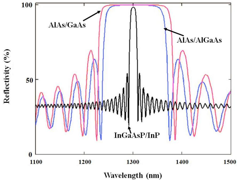
**Figure 2-5: Reflectivity profiles of 25 mirror pairs DBR stack of AlAs/GaAs (red), AlAs/AlGaAs (blue) and 150 mirror pairs of InGaAsP/InP (black) with  $\lambda_B=1300\text{nm}$ .**
