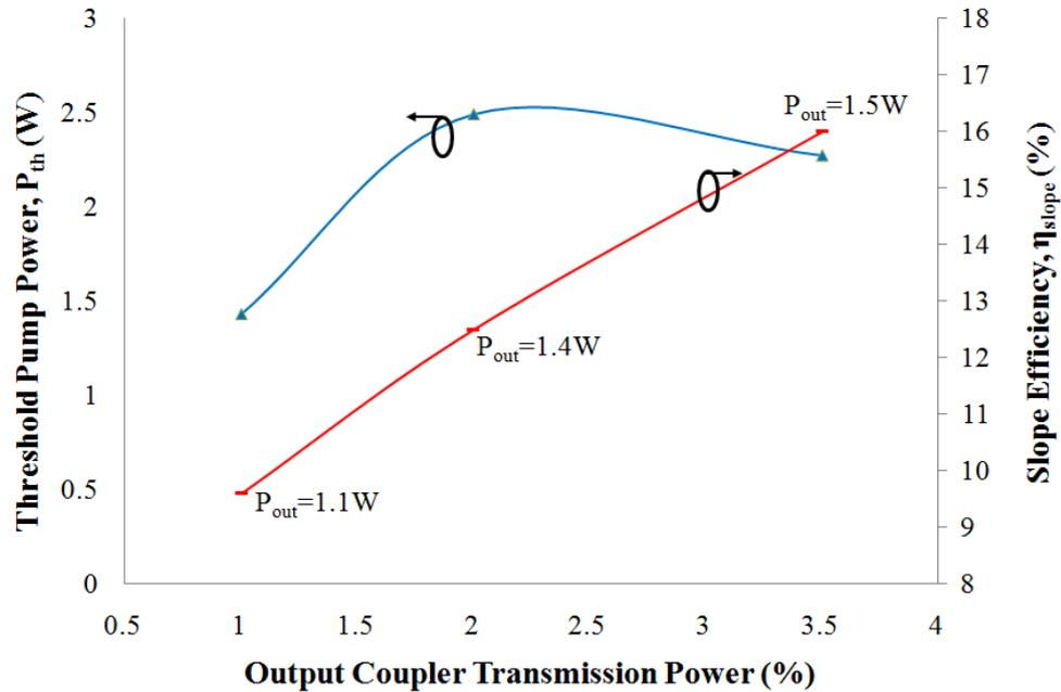
**Figure 4-17: Threshold pump powers (blue) and slope efficiencies (red) across a range of output couplers  $T=1\%$ ,  $2\%$  and  $3.5\%$  for sample  $AsN2527$  1220 nm.**
