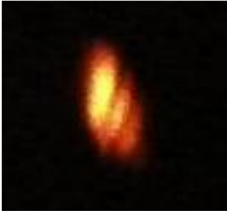
**Figure 6-24: Picture of the yellow/orange frequency doubled output beam indicating a multimode profile.**
