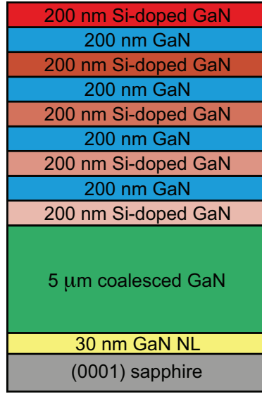
Figure 4.1: Schematic of the sample structure of the Si-doped c -plane GaN epilayer. The Si concentration increases from 5.5 \times 10^{17} to 1.0 \times 10^{19} \text{ cm}^{-3} in the bottom four n -type GaN layers. The Si concentration of the top GaN layer is 1.0 \times 10^{18} \text{ cm}^{-3} .
