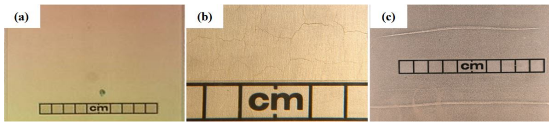
Figure 7.15: Photographs (a) circular blowhole of approx. 10 mm diameter, (b) lining shrinkage cracks (c) scoring
