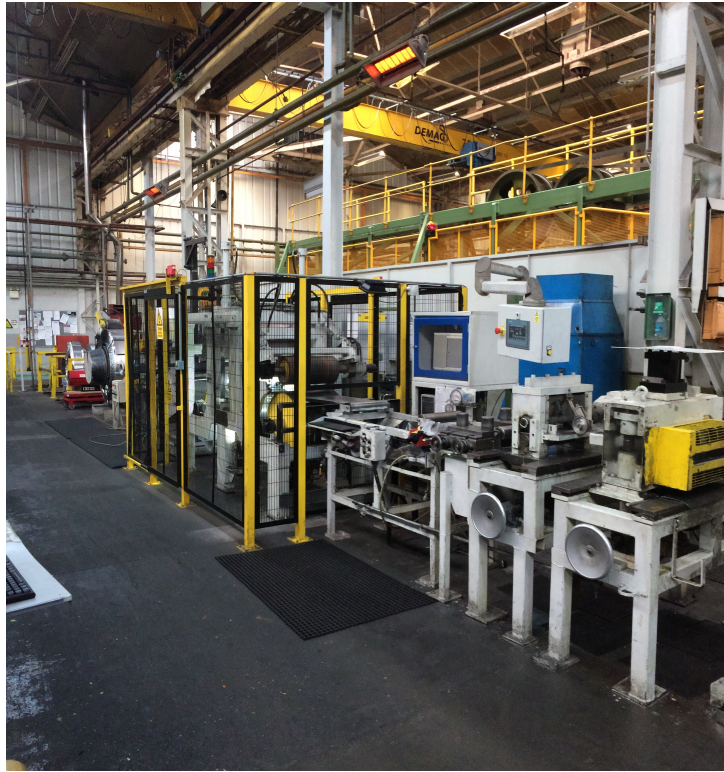
Figure 9.2: SIC machine vision final inspection line in Kilmarnock
