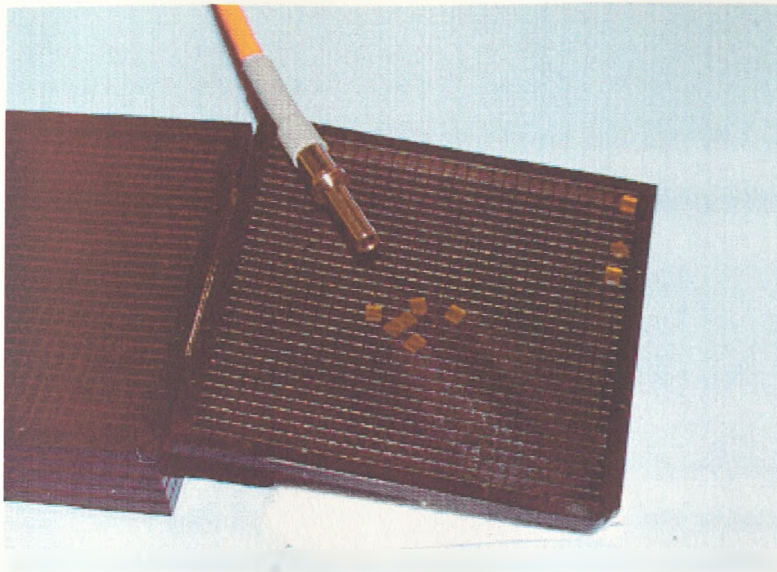
Figure 5-17 GRIN lens assembly and POLARCOR polarisers
