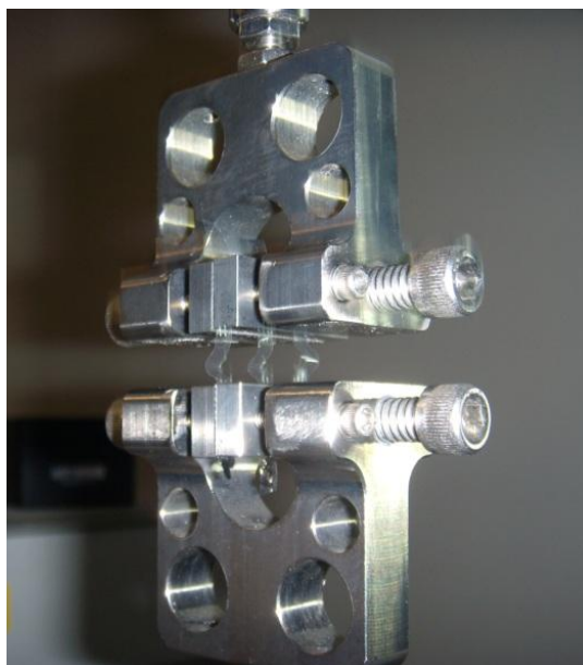
Figure 7.4 - Fatigue testing polymer samples between grips of the Bose ELF Tester.
