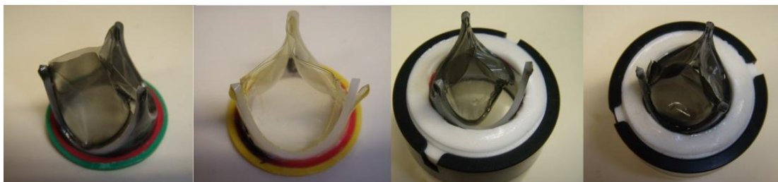
Figure 8.14 - Initial failure modes of valves with a Delrin stent; leaflet de-bonding from stent.
