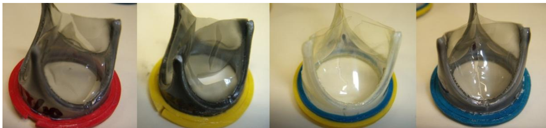
Figure 8.16 - Primary failure mode of valves with a polycarbonate stents; leaflet rupture across belly region.
