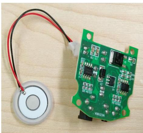
Figure 7.3 Ultrasonic atomiser used to generate micro drops.
