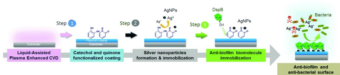
Figure 2.20 Schematic of the elaboration of multifunctional surfaces achieved via liquid-assisted plasma-enhanced chemical vapour deposition [197].
