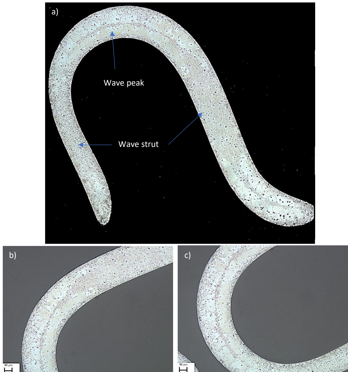
Figure 5.14: Microstructure of a single wave of a 0.5Y device annealed in the vacuum furnace for 30mins at 300°C a) complete wave b) wave strut c) wave peak
