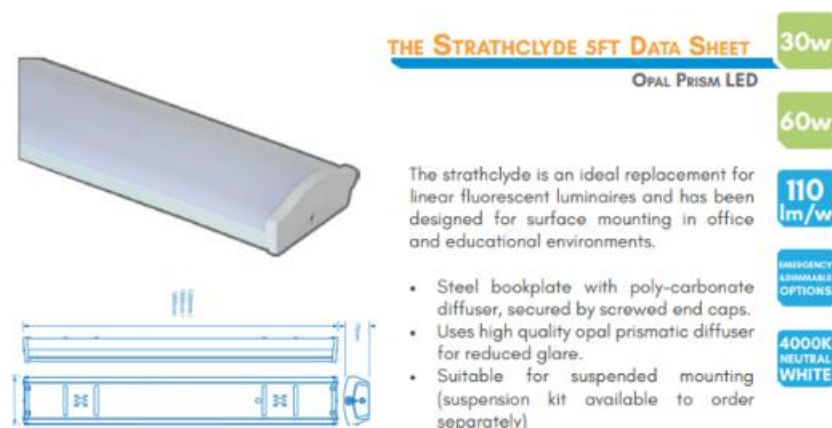
Figure 5.4: ‘Strathclyde’ luminaire description from the company’s catalogue
