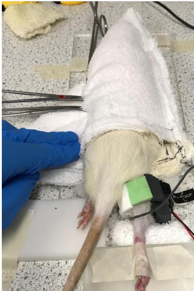
Figure 31: Animal Trial experimental set-up showing rat pouch, vibration device on hindleg, during vibration session
