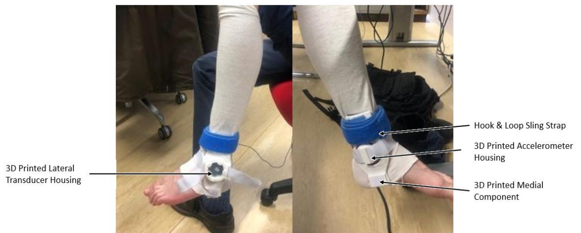
Figure 24: Photo of the wearable ankle device as used during the 2nd investigation at the University of Strathclyde
