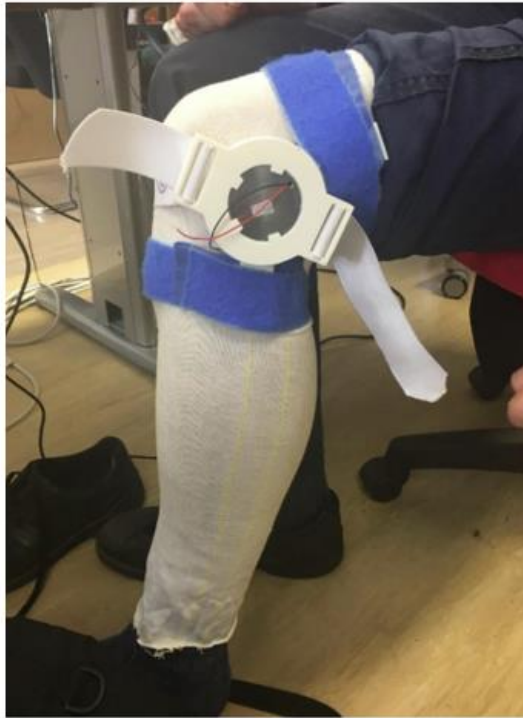
Figure 22: Photograph of the early straps used (hook & loop sling) vs. knee straps as applied to the knee region
