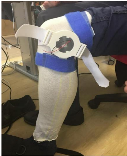
Figure 15: Photo of early wearable device prototype applied to the knee with hook & loop sling and elasticated strap, unpowered featuring tubigrip sock padding
