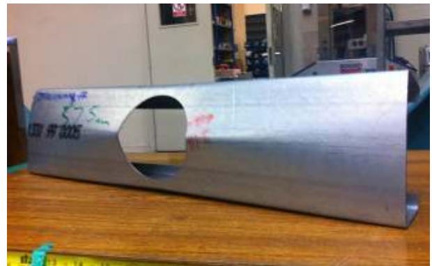
(c) Comparison deformation shape for type-2 holes
