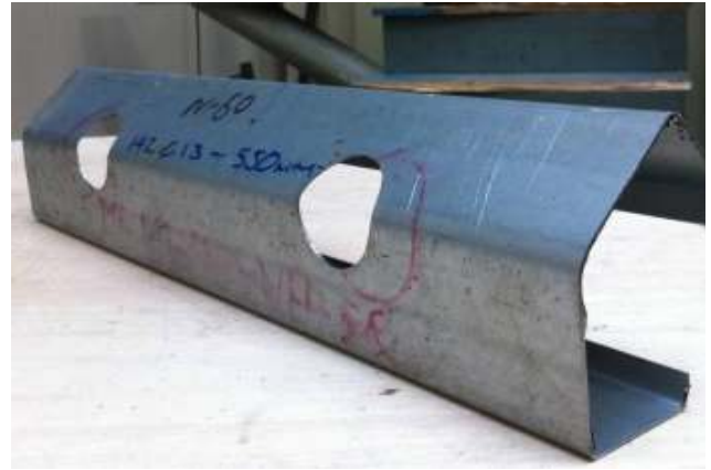
(b) Comparison deformation shape for type-1 holes
