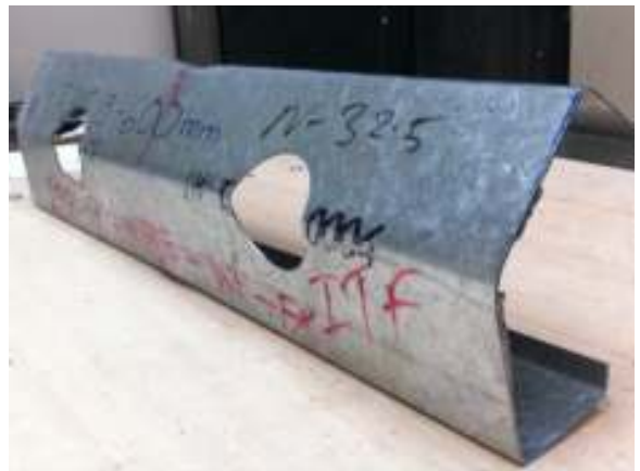
(b) Comparison deformation shape for type-1 holes
