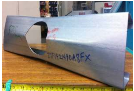
(c) Comparison deformation shape for type-2 holes
