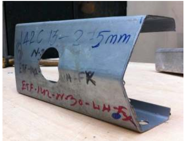
(b) Comparison deformation shape for type-1 holes
