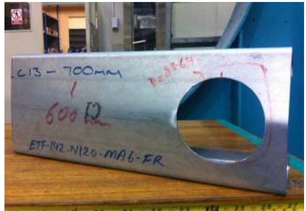
(c) Comparison deformation shape for type-2 holes
