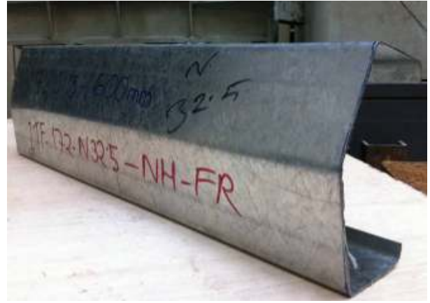
(a) Comparison deformation shape for without holes
