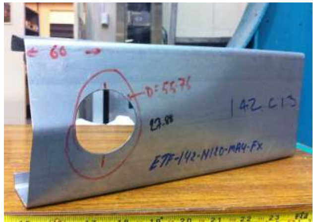
(c) Comparison deformation shape for type-2 holes
