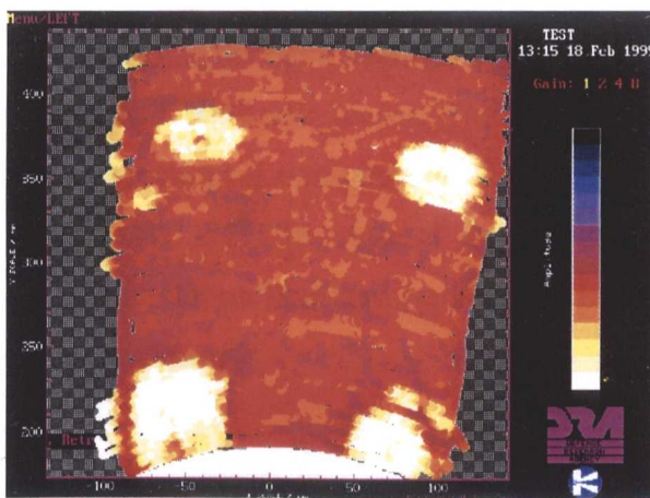
Figure 6.53 C-scan of damaged carbon fibre plate Figure 6.54 Schematic of carbon fibre testplate
