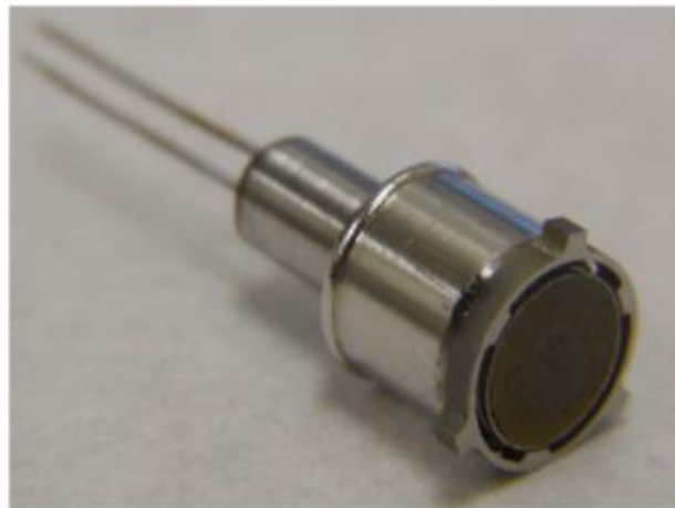
Figure 1-11. A cesiated tungsten photocathode [123].
