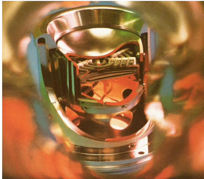
Figure 1-10. Thermionic electron gun showing the cathode and the heater mechanism for the electron extraction (photograph courtesy of TMD Ltd).
