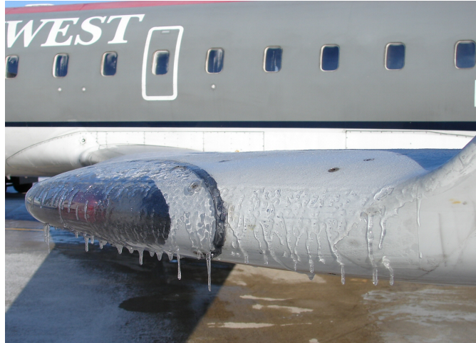
Figure 1.3: The accretion of ice on the wing of an aeroplane. Image courtesy of Cory W. Watts, sourced from [174].
