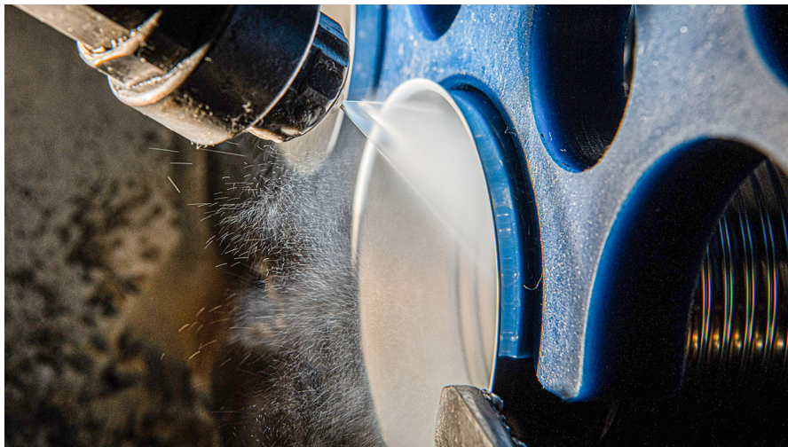
Figure 1.4: Spray coating of a thin protective coating onto the inside of a metal can. Sourced from Cornwall [29], reprinted with permission from The American Association for the Advancement of Science (AAAS).
