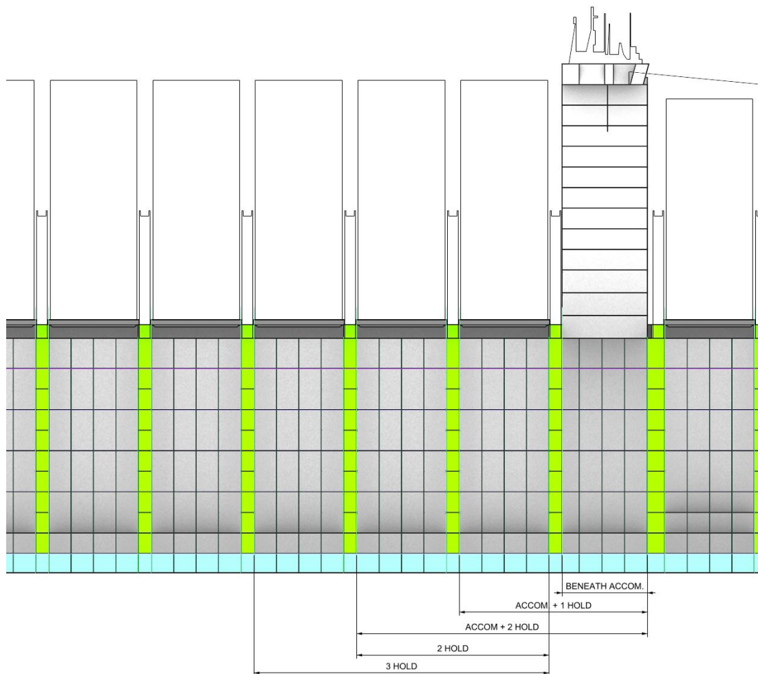
Figure 45: Tank Size Designation defining Different Tank Extents
