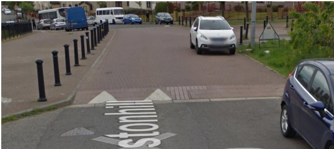
Figure 3-9 – Raised Platform Creating High Vertical Acceleration
