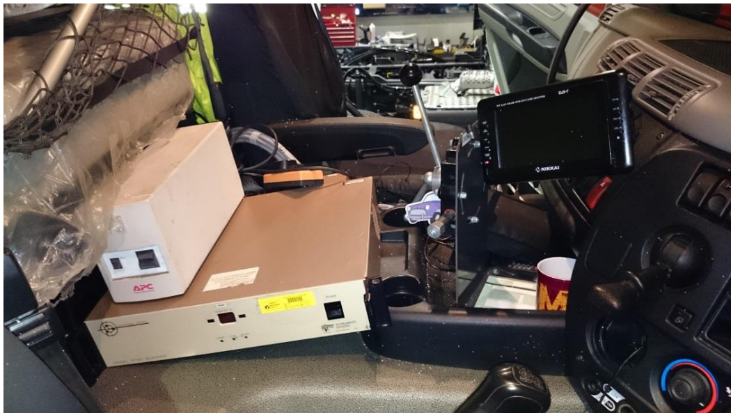
Figure 3-1 - In-cab Data Logging Equipment
