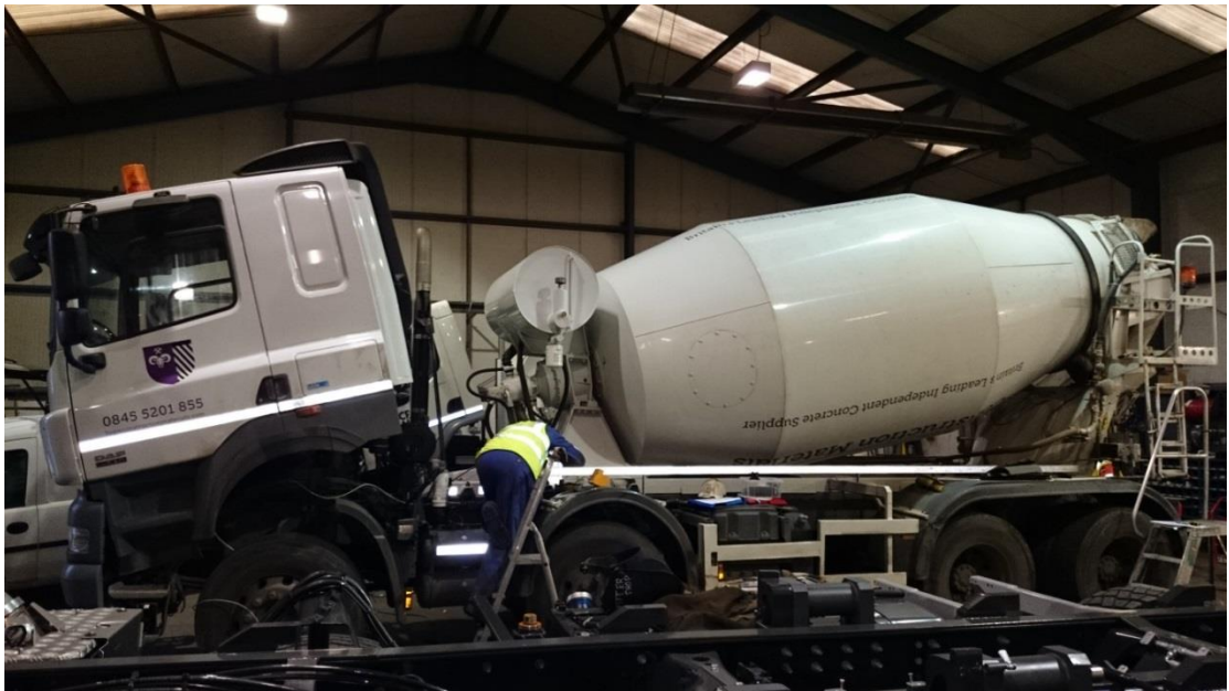
Figure 3-2 - Test Truck - DAF CF85 with 8m 3 Mixer Unit
