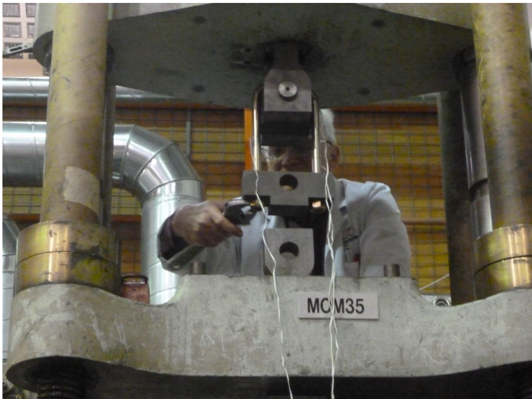
Figure 3-20 - Setting up U-Bolt Test
