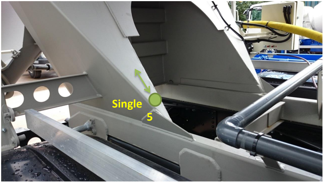
Figure 3-4 - Schematic of Strain Gauge Position 5
