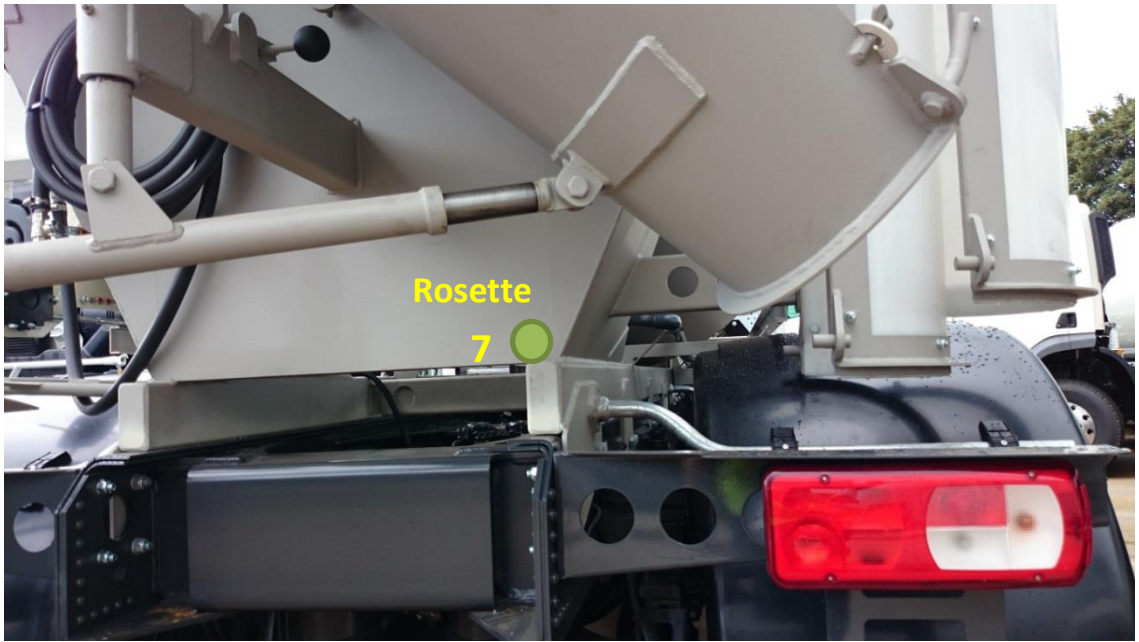
Figure 3-6 - Schematic of Strain Gauge Position 7
