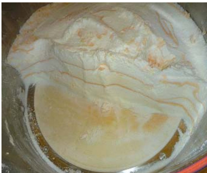
Figure 32: Filter cake of API 1 obtained in pilot plant.
