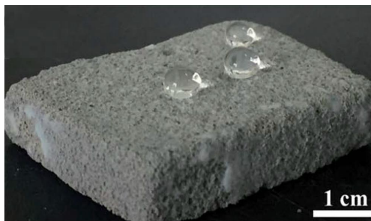
Figure 2-2 Aerogel/geopolymer composites during the hydrophobicity test, reproduced from [38]
