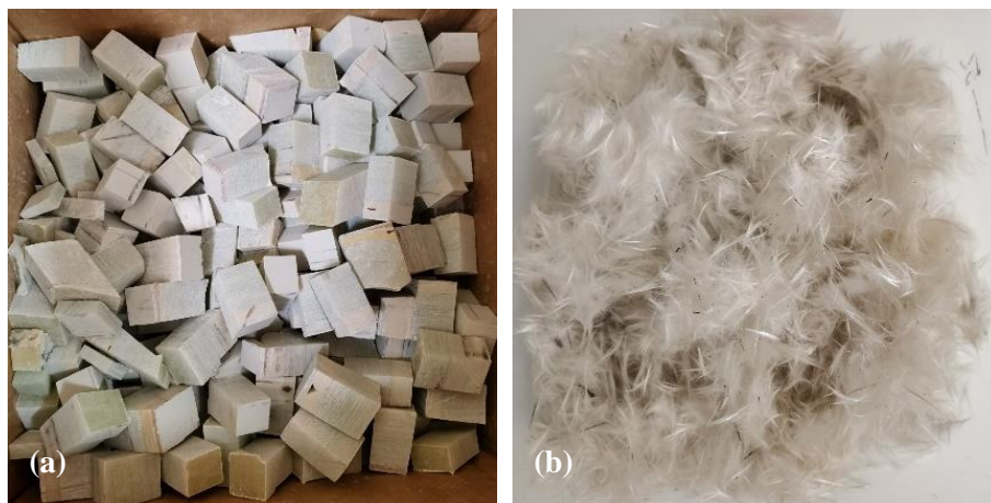
Figure 2-18 (a) GFRP cubes before the recycling process, and (b) Recycled glass fibre after the recycling process
