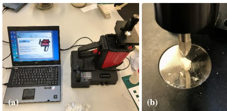
Figure 4-6 (a) Agilent Technologies 4100 Exo Scan (b) detailed view of the sample
