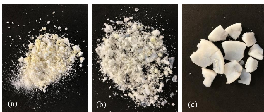
Figure 4-9 The morphology of aerogel prepared with solvent: gel (amount of sodium silicate, HCl, and \text{NH}_4\text{OH} ) volume ratio (a) 1:1, (b) 1.5:1, and (c) 2:1
