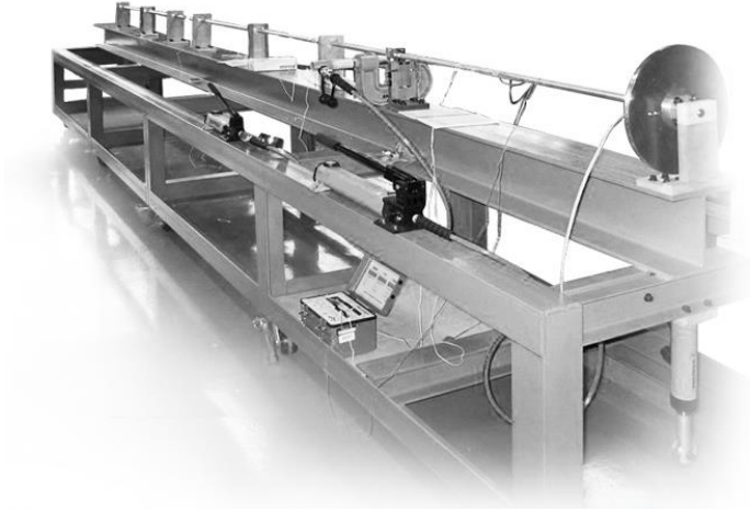
Split Hopkinson pressure bar test equipment
