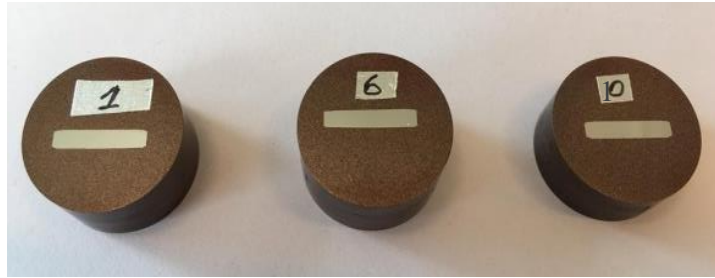
Figure 4.25 Prepared specimens from the electrolyte containing 1, 6 and 10 wt% of water for EBSD analysis.
