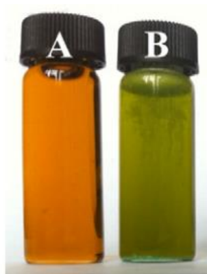
Figure 2.11 a) Appearance of the fresh electrolyte ChCl: 2 EG containing 0.45 M of Cu (II) species, and b) appearance of the electrolyte after 6 h of plating. Adapted from [113].
