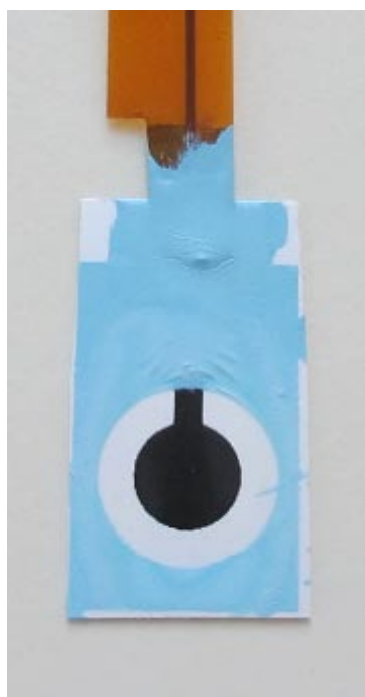
Figure 6.6 Fully isolated sensor to allow full emersion in solution.
