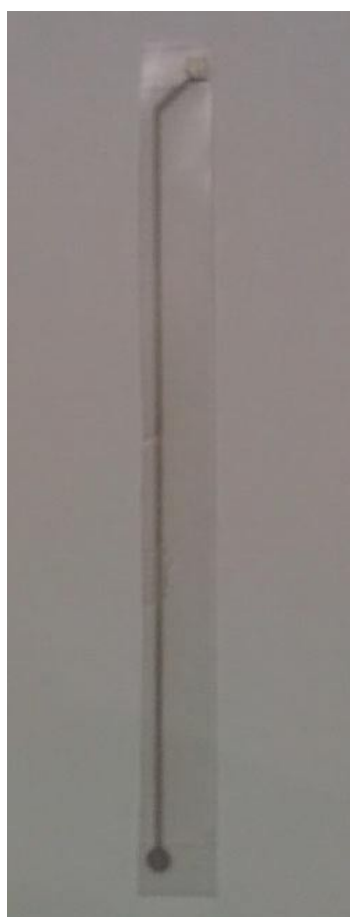
Figure 3.11 Screen printed Ag/AgCl of reference electrode.
