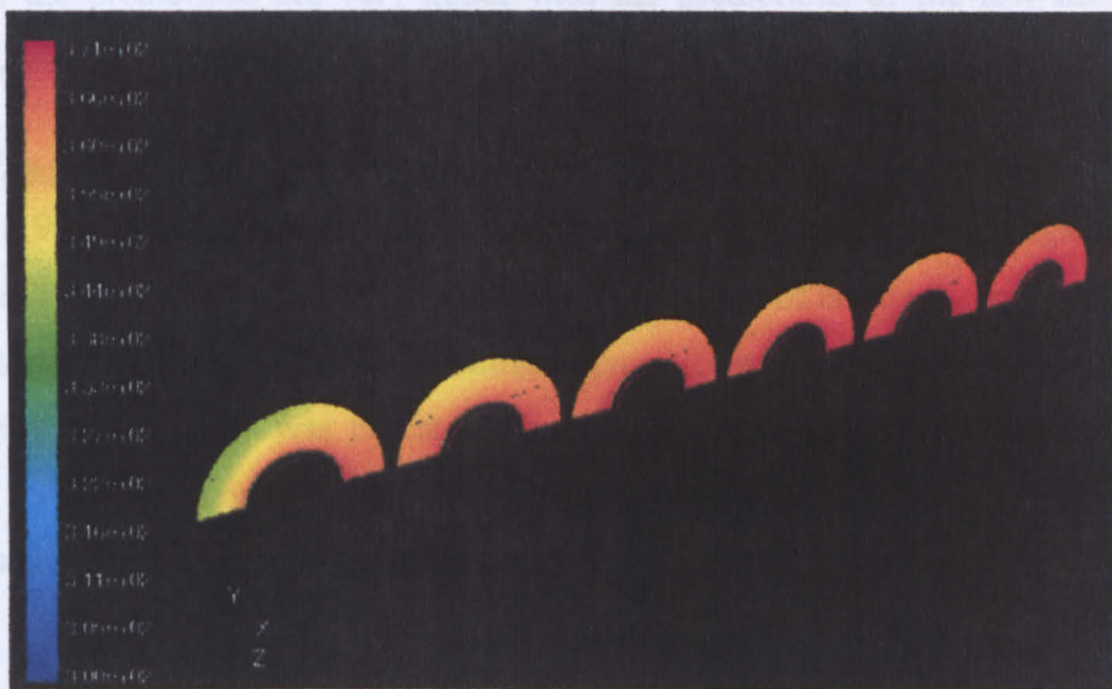
Figure 7.11: Temperature contours over fins and tubes for Bundle 3 at 0.79kg/s (Flow direction left to right, temperature scale (K) on left)
