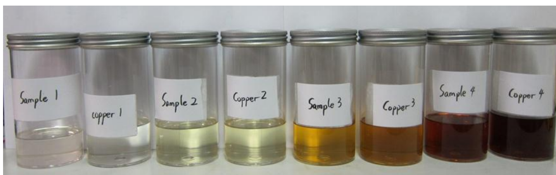
Figure 5-1 Aged Samples: Sample 1 and Copper 1 unaged; Sample 2 and Copper 2 aged for 2 days at 120°C; Sample 3 and Copper 3 aged for 4 days at 120°C; Sample 4 and Copper 4 aged for 8 days at 120°C.
