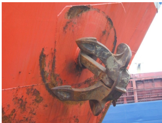
Figure4.15. Damages of front area paint because of anchor
