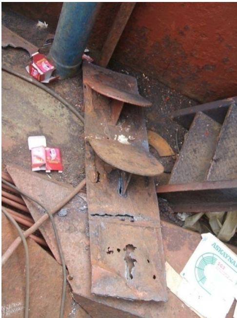
Figure4.7.a. Damaged ladder sample
