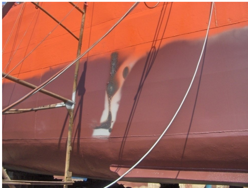
Figure4.16. Sample of paint burning due to wrong work order
