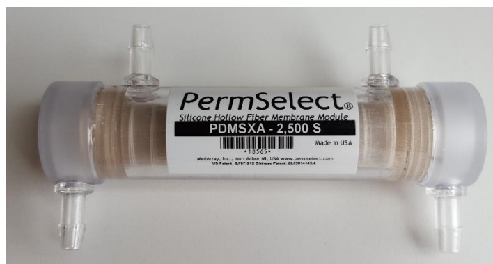
Figure 4.21. An in-line degassing module. Vacuum is applied to the shell side and the liquid to be degassed flows through a bundle of silicone fibres.
