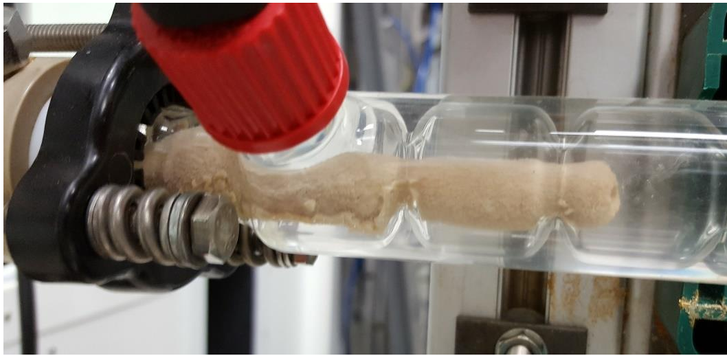
Figure 4.18. Localised fouling of the stainless steel inlet at the mixing location in the COBC.
