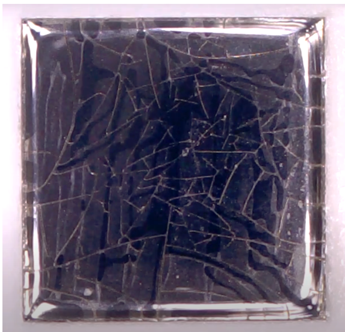
Figure A3.3 – Microscope image of a dehydrated ‘concentrate’ sample. As the sample dries it begins to crack and then lifts off the SIRE surface.
