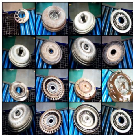
Figure 42 One batch of the original torque converter samples used to train the model
