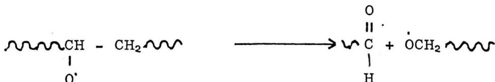
The free radical formation in the irradiated polyethylene is a main step in the crosslinking process, and one which is readily observed by E.S.R. (13). These free radicals which are formed could be trapped firm within the crystalline region of the irradiated polyethylene.
