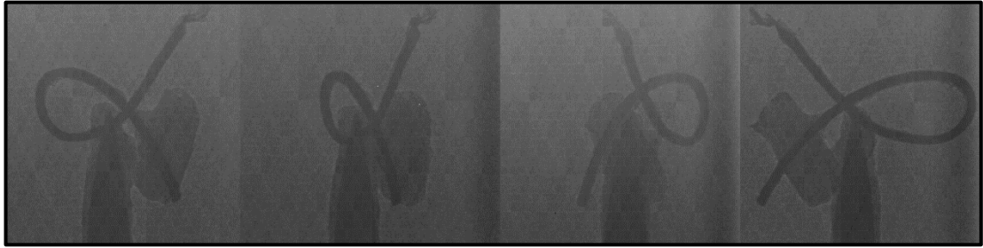
Figure 4.34. Four raw projections recorded by the ANDOR X-ray camera during the micro-tomography experimental run. It can be seen that the contrast changes between projections.
