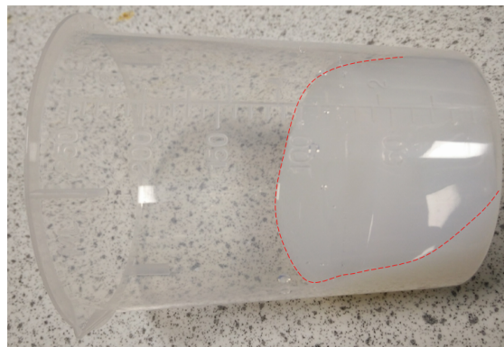
Figure 5-24 Modified gel state test control specimen following 45 mins of testing.
