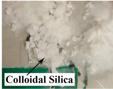
Figure 3-10 Colloidal silica specimen following freeze drying
