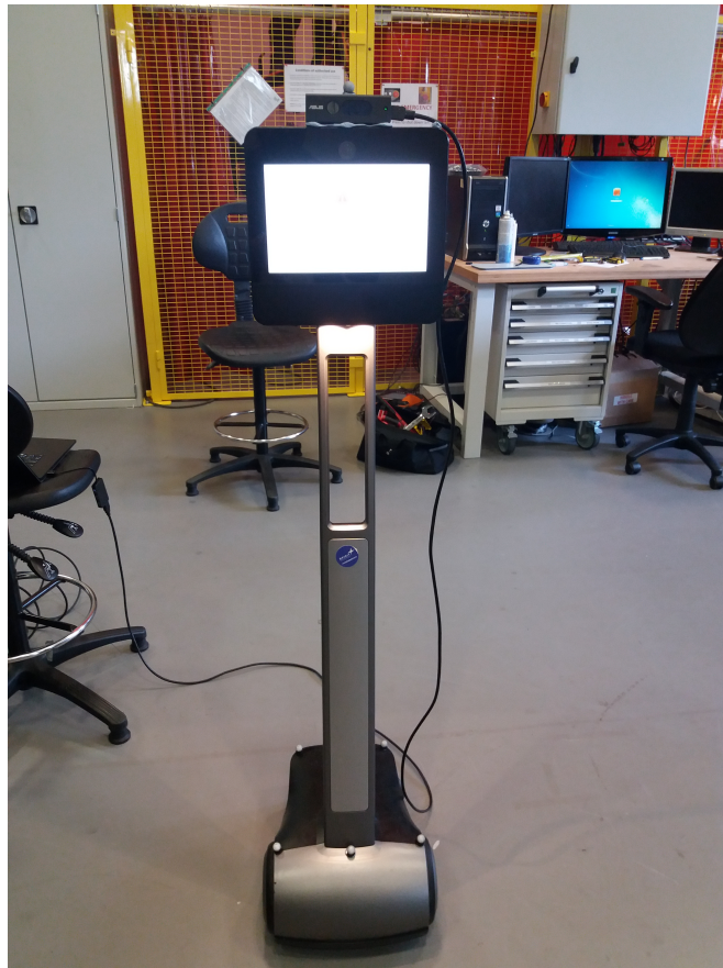
Figure 7.2: Telepresence robot Beam plus with ASUS Xtion-2 camera mounted for visual SLAM measurement in our experiment.
