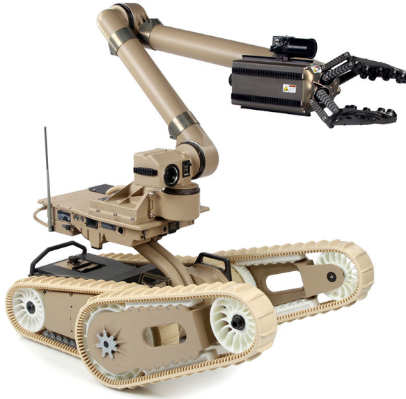
Figure 2.3: Example of a teleoperated robot for nuclear power plant application: iRobot Warrior [17].
