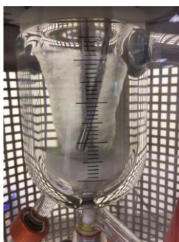
Figure 51 Ecoclave hydrogenation vessel equipped with gas-entrainment impeller.
