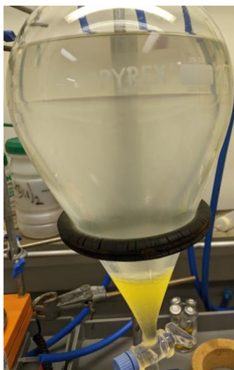
Figure 66 Formation of triphasic system; top layer: heptane, middle layer: aqueous acetonitrile, bottom layer: organic acetonitrile.
