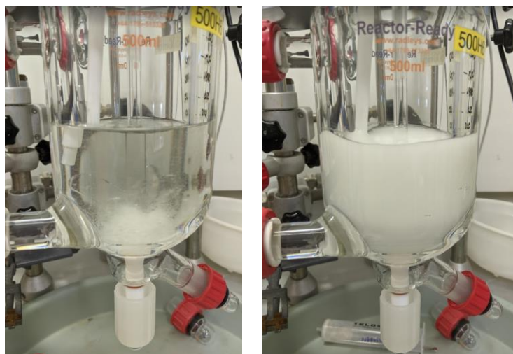
Figure 68 Seeded cooling crystallisation process of benzyl bromide ester ( 4.9 ).
