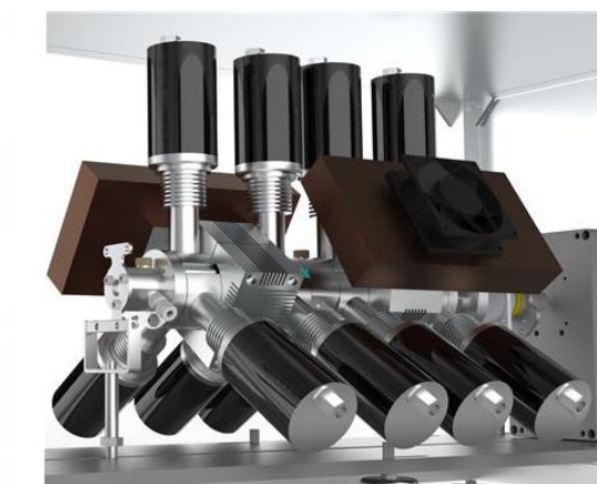
Figure 72 Computationally generated 3D model of next iteration of Photo DART Reactor design.
