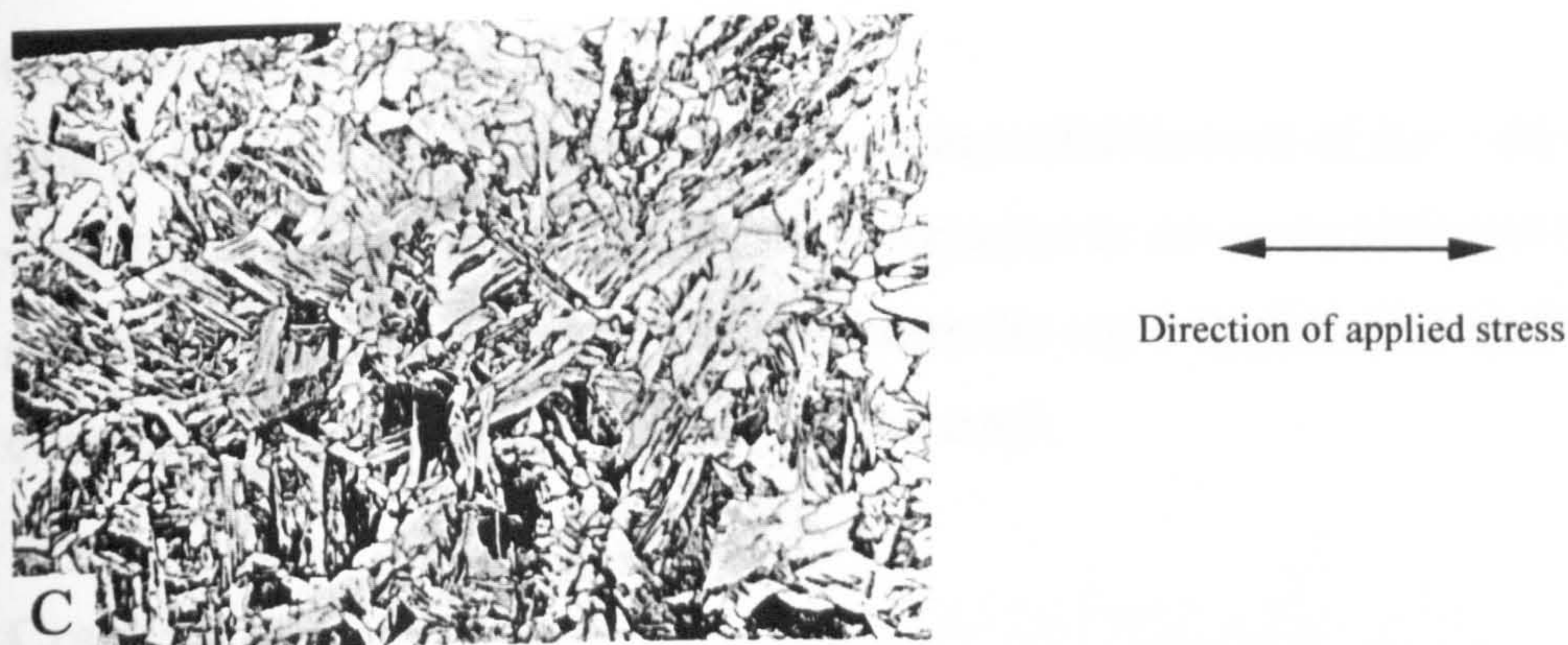
Figure 5.684 - Microstructure of vibrated specimens (points A, B, and C of the three sections Figure 5.681 and 5.682) ( \times 200 )
