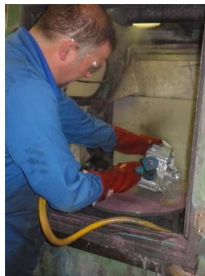
Figure 37: Rinsing of residue after shot blasting
