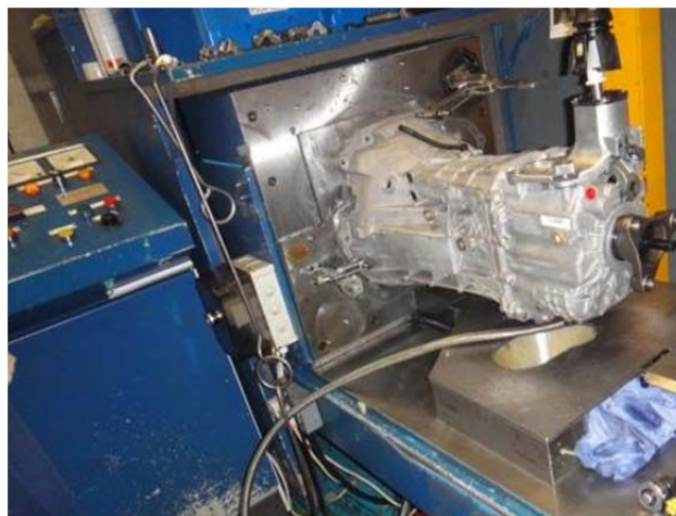
Figure 45: Testing a manual transmission
