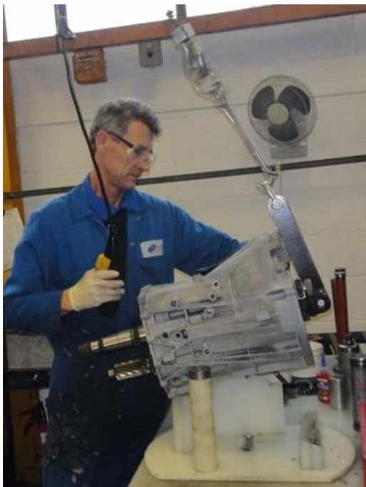
Figure 42: Electric hoists used during re-assembly
