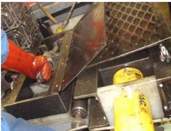
Figure 27: Custom made hydraulic pullers
