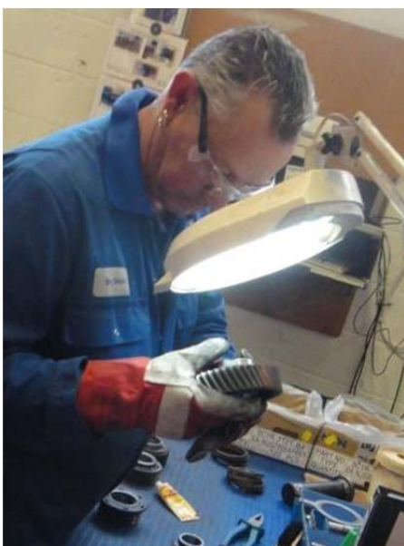
Figure 40: Visual inspection of a gear
