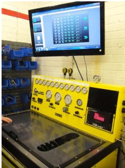
Figure 21: Transmission shifter test machine
