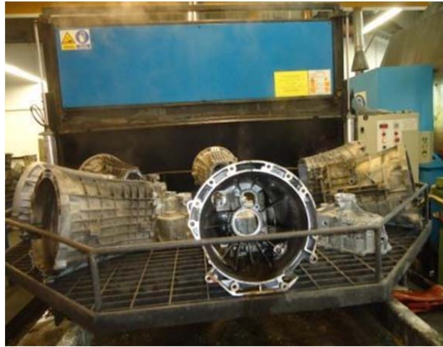
Figure 31: Aqueous-based chemical washer for transmission housing
