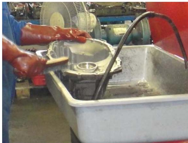
Figure 35 : Manual cleaning of transmission housing
