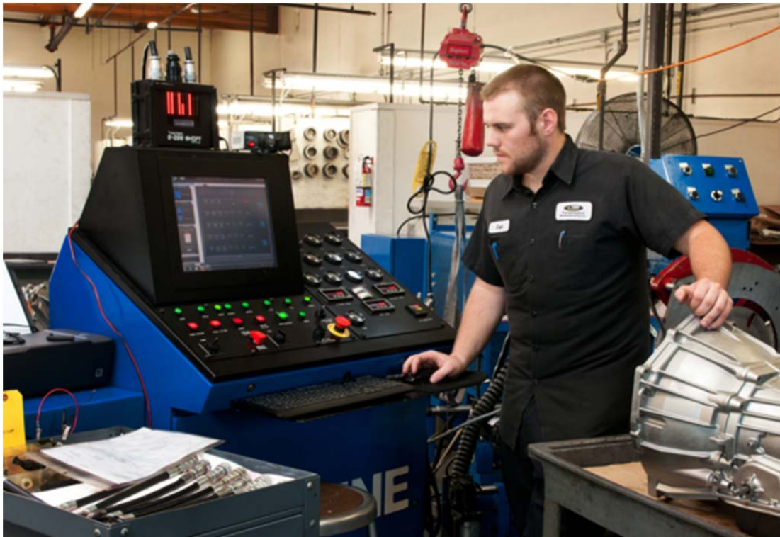
Figure 7: An automatic transmission testing unit (“ www.blureachautomation.com ,” 2013)
