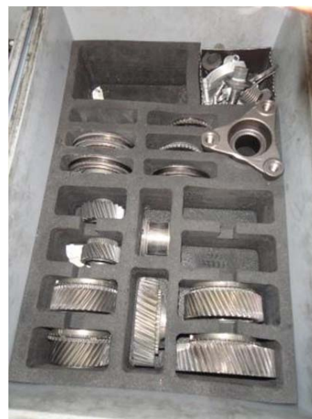
Figure 41 : Container to arrange the components for assembly
