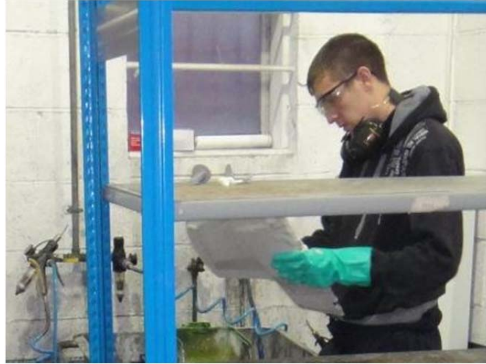
Figure 46: Cleaning a copier panel with an air-gun
