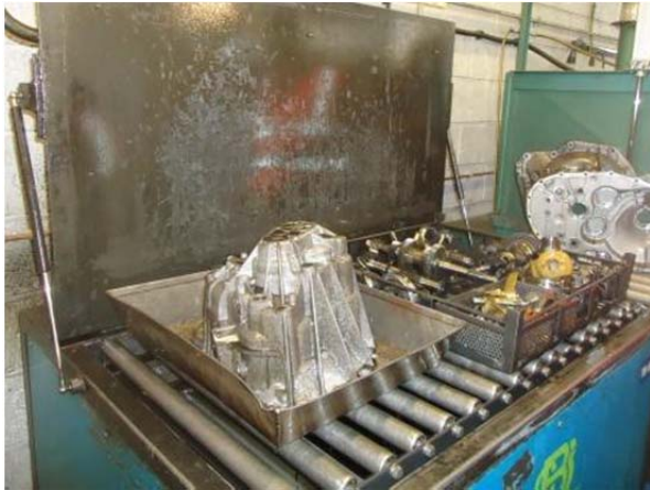
Figure 29: Kerosene washer tank
