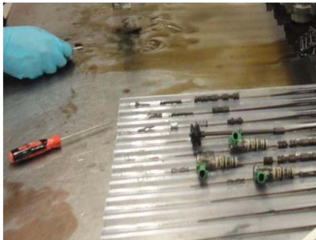
Figure 53: Cleaning of valves in the hydraulic controller unit of an automatic transmission
