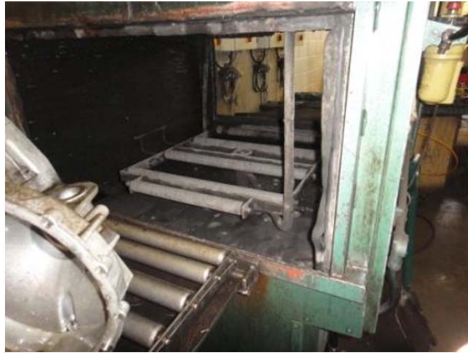
Figure 34: Spray cleaner inside view
