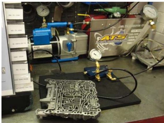
Figure 19: Vacuum test for valve body
