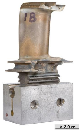
Figure 4-2 Image of turbine blade in blade holder.
