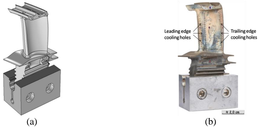
Figure 6-11 Turbine blade representation (a) FE model (b) image of turbine blade.
