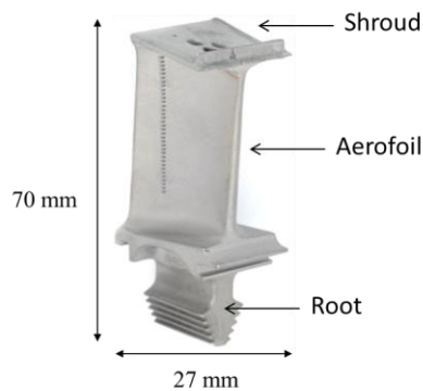
Figure 3-1 Turbine blade used in empirical study.
