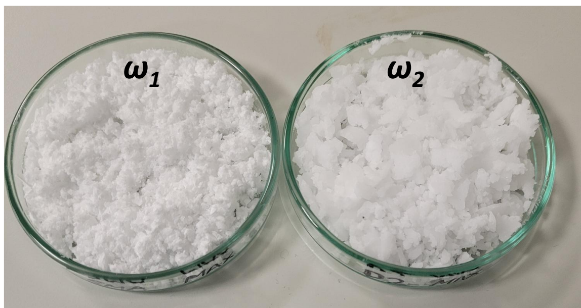
Figure C4: Pictures of obtained solids from batches \omega_1 and \omega_2 that present a wet aspect as they are not completely washed from their viscous liquor. While \omega_1 is described as slightly wet as it presents small agglomeration, \omega_2 is characterized as very wet as large agglomerates can be observed.
