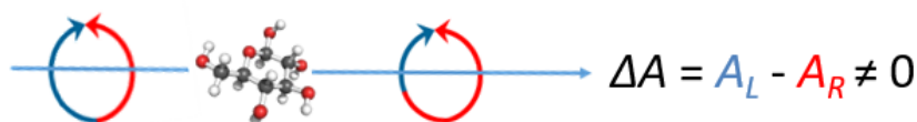
Figure 4.1: Circular dichroism: a light source composed of an equal amount of left-handed (blue) and right-handed (red) circularly polarized light, one of which is preferentially absorbed by a chiral molecule. A differential absorbance \Delta A is measured between the absorbance of left-handed light A_L and right-handed light A_R .
