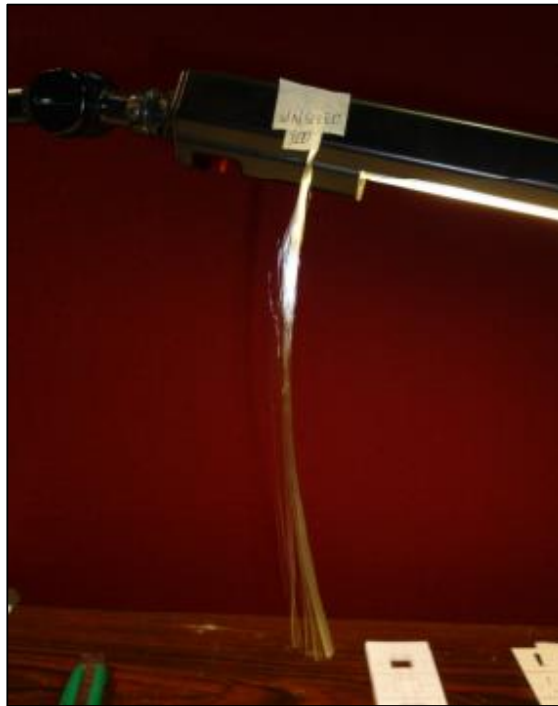
Figure 2.4 Single fibre separation from GF bundle.
