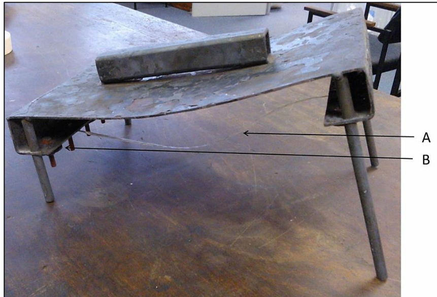
Figure 2.2 Bundles Steel Rig. A) GF Bundle. B) Nut, bolt and washer.
