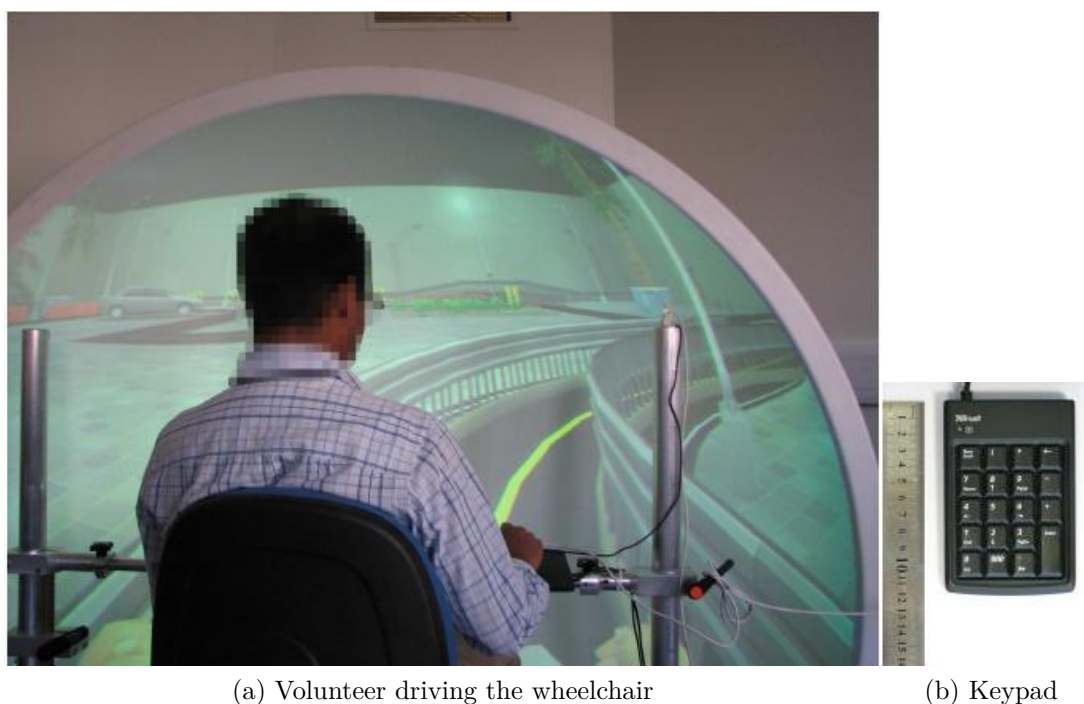
Figure 3.1: A volunteer driving the wheelchair in the VR simulator environment using a keypad as the access device. Adapted from Grychtol (2010)
