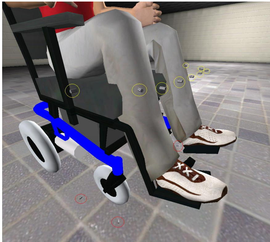
Figure 3.3: Side view of the wheelchair showing relative height of the sonar sensors, encircled in yellow. IR sensors are marked in red
