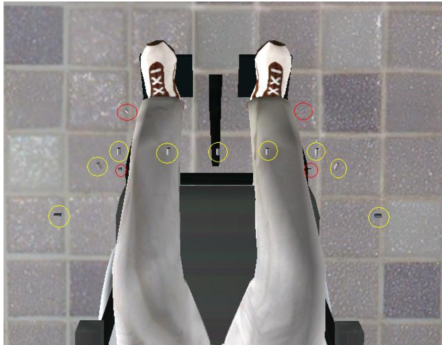
Figure 3.2: Top view of the sensor arrangement showing all 9 sonar sensors (encircled in yellow) and 4 IR sensors (encircled in red)
