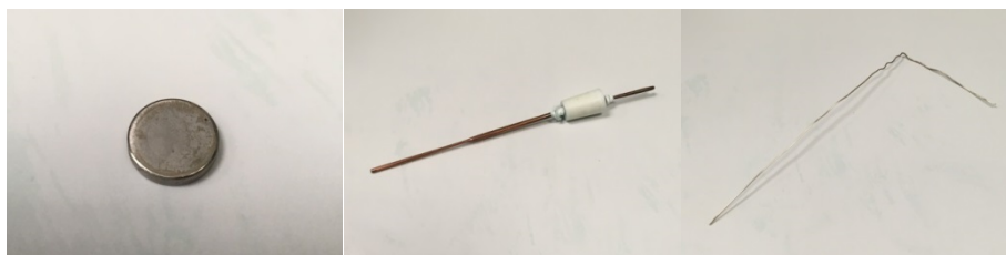
Figure 4-2 Working electrode (left), counter electrode (middle) and reference electrode (right)
