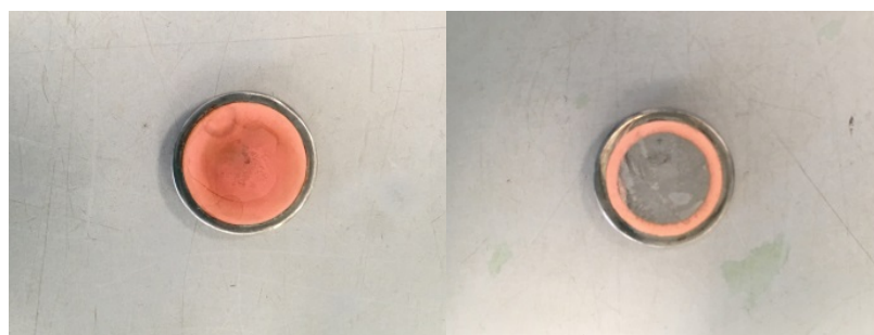
Figure 5-8 Plated Cu deposit on steel substrate before (left) and after (right) 15 minutes dissolution experiment in 0.2 M Cu ethaline under 700 rpm RDE rotation speed
