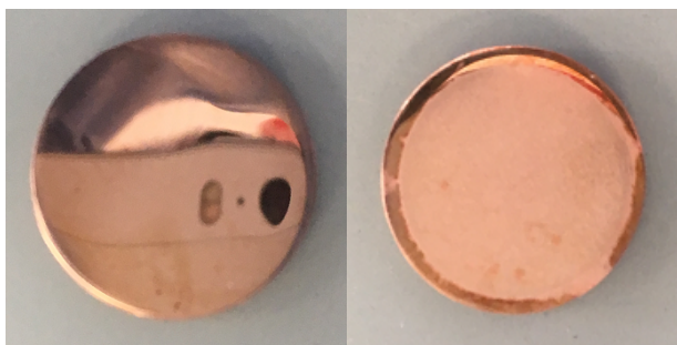
Figure 5-11 Visual appearance of Cu disc before (left) and after the dissolution experiment (right)
