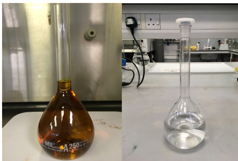
Figure 4-1 Virgin cupric ethaline melt DES electrolyte (left) and tin ethaline melt DES electrolyte (right)
