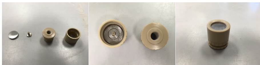
Figure 4-3 Working electrode tip holder assembly and components
