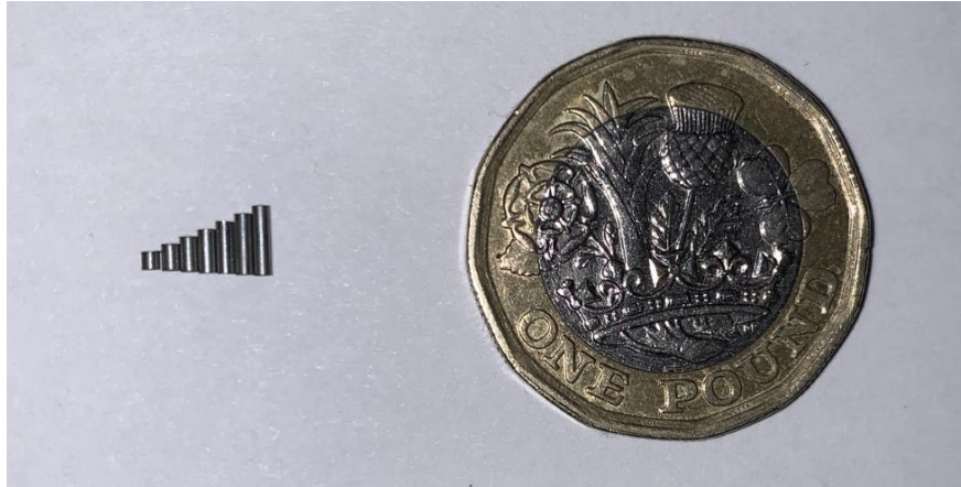
Figure 7.1 – Range of the samples used, from 1 mm length to 4 mm length with increments of 0.5 mm. Addition of £1 coin for size reference of the samples.
