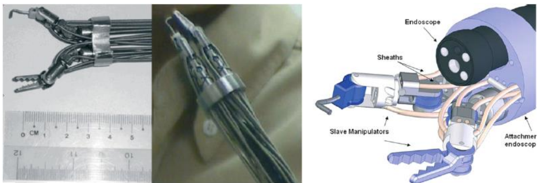
Figure 14: The MASTER system with its two cable actuated robotic arms with fixed end effectors (left) attached to a conventional endoscope (right). (Phee et al 2008)
