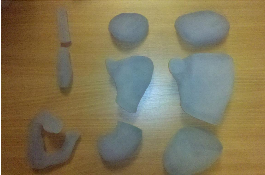
Figure 32: Prototyped UGI models in nylon. Parts to the left include oesophagus and duodenum. Parts in the middle consist of the fundus, body and antrum of the stomach at 100% size. The parts to the right consist of fundus, body and antrum of the stomach at 200%.
