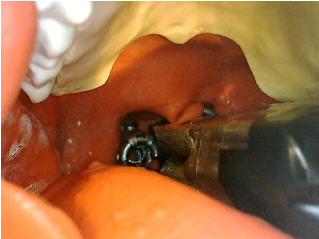
Figure 94: Endoscope in the oral cavity. The length of the front unit rendered intubation through the pharynx impossible.
