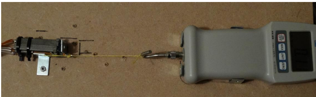
Figure 88: Pulley setup for measuring forward instrument traction.
