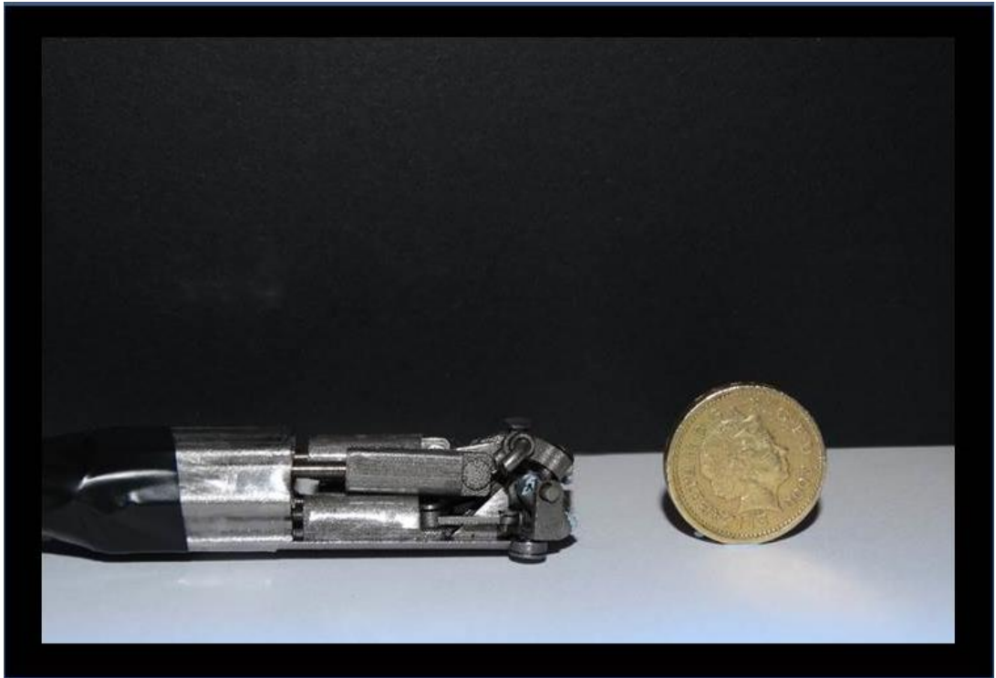
Figure 76: 1:1 stainless steel prototype side view. A £1 coin was used for size comparison.
