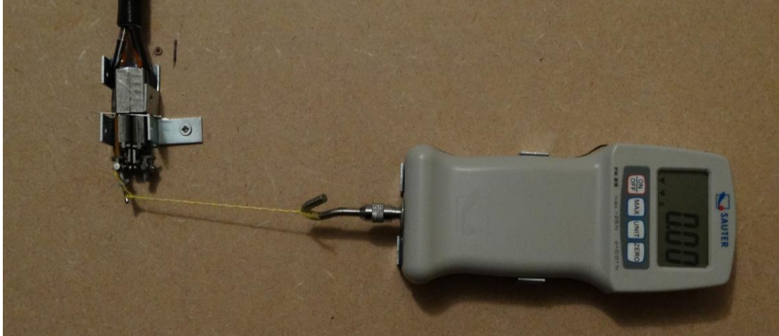
Figure 86: General setup for measurement of lateral, medial, upward and downward traction.
