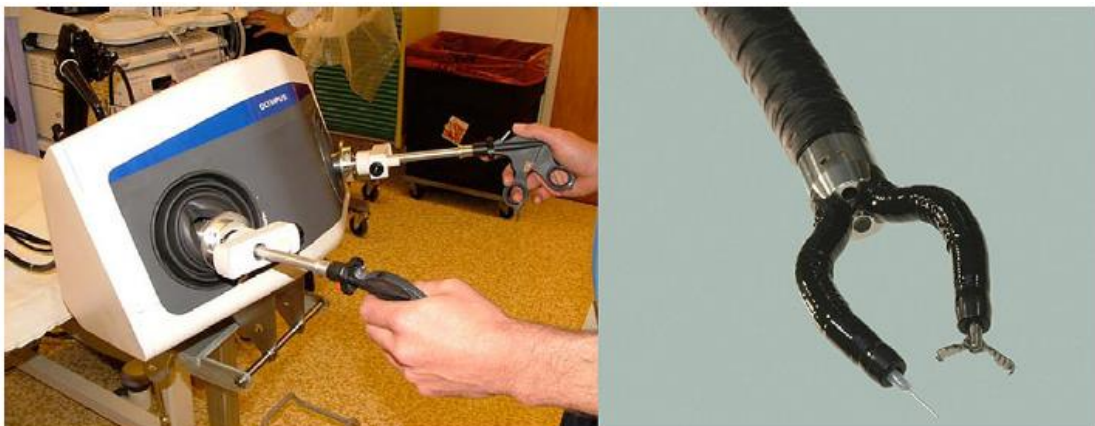
Figure 10: Endosamurai with its control console similar to a laparoscopic system (left) and two hollow cable controlled instrument guide arms (right). (Ikeda et al 2011, Spaun et al 2009)
