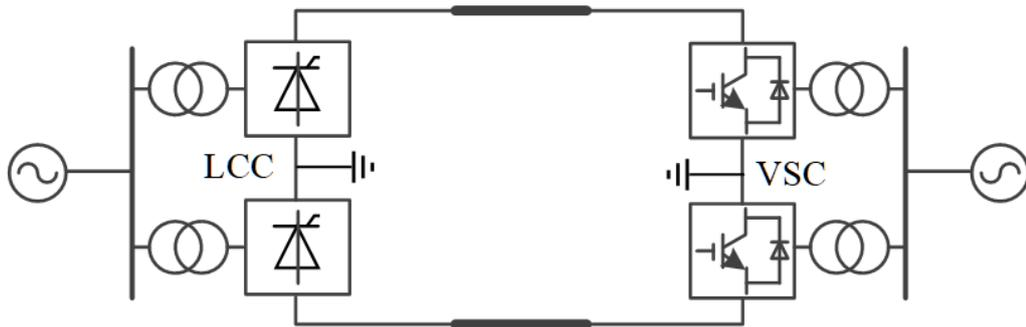
Fig. 2.9 HVDC system with hybrid terminals.
