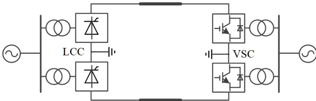
Fig. 2.9 HVDC system with hybrid terminals.
