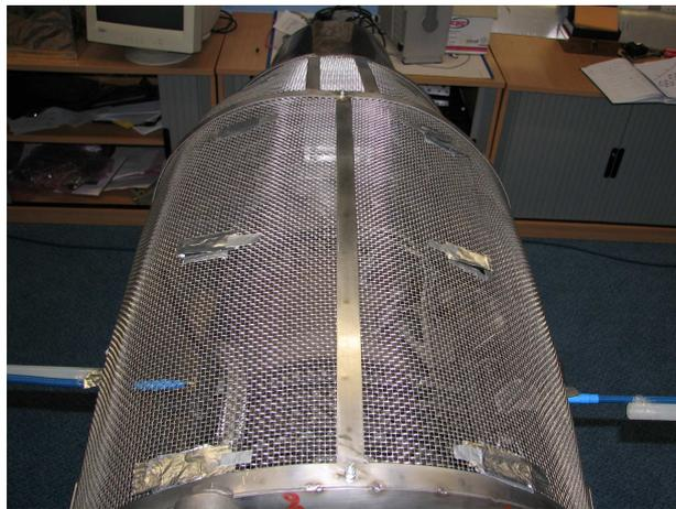
Figure 4.11: Gnome engine with cowling.
