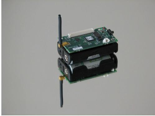
Figure 5.3: The MICAz transceiver.
