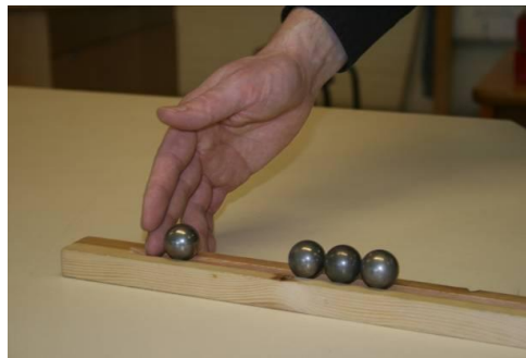
3. Ball running into a set of identical balls.
